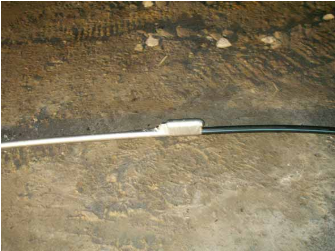
Figure 6. Upper geofone attached to the plastic hose used for cementing.
