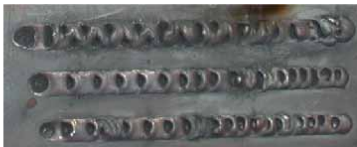
Figure 13. Blowholes in copper workpiece.
