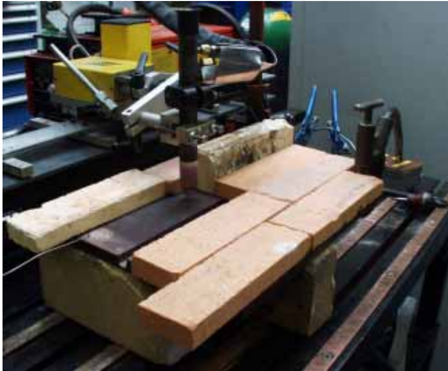
Figure 11. Preheating arrangements for the welding trials.
