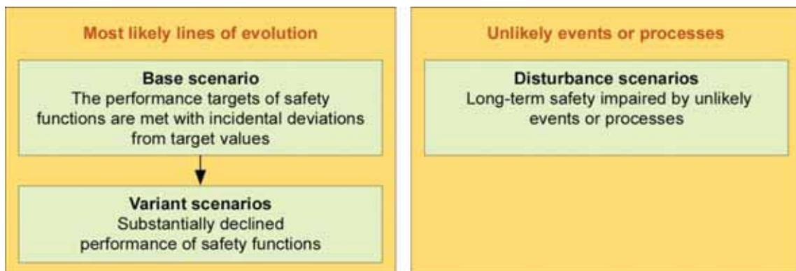
*Figure 2-1. Scenario classification according to YVL Guide D.5 (STUK 2009).*
