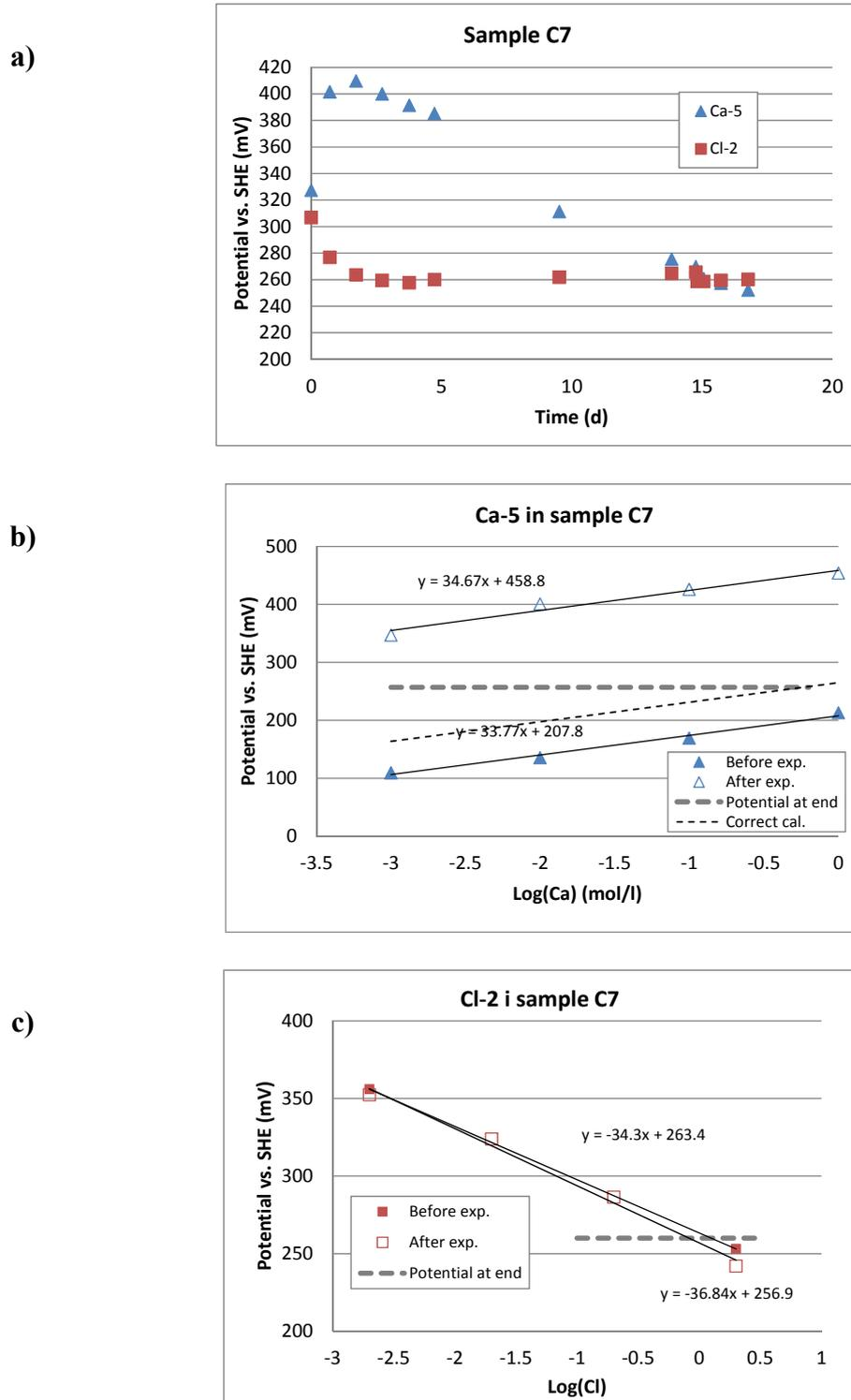
**Figure A6.** Measurement of calcium and chloride concentrations in the calcium bentonite sample C7. Dry density  $1.63 \text{ g/cm}^3$ , measured chloride concentration in bentonite  $0.817 \text{ mg/g}$ .
