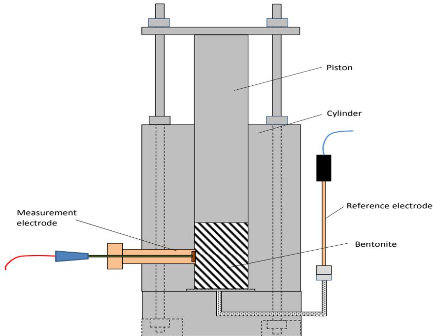
**Figure 11.** Schematic presentation of the measurement cell for ion-selective electrodes in compacted bentonite.
