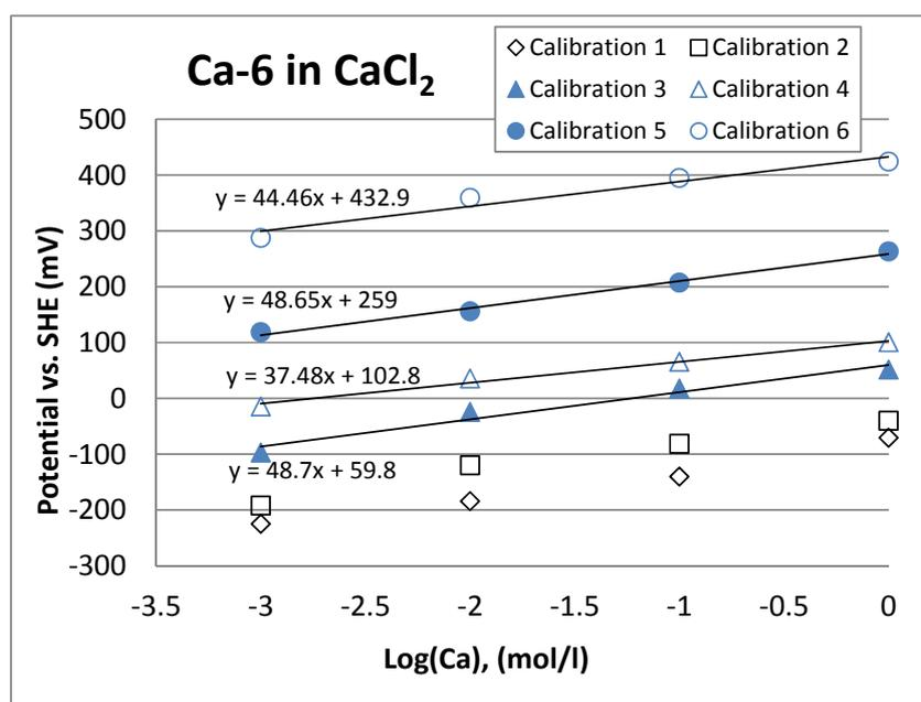
**Figure 10.** The potential of a calcium electrode as a function of the logarithm of the calcium concentration in  $\text{CaCl}_2$  solution in repeated calibrations. The numbers of the measurements are given in the legend. In the bentonite measurements the electrode was between the calibrations 3 – 4 and 5 – 6.
