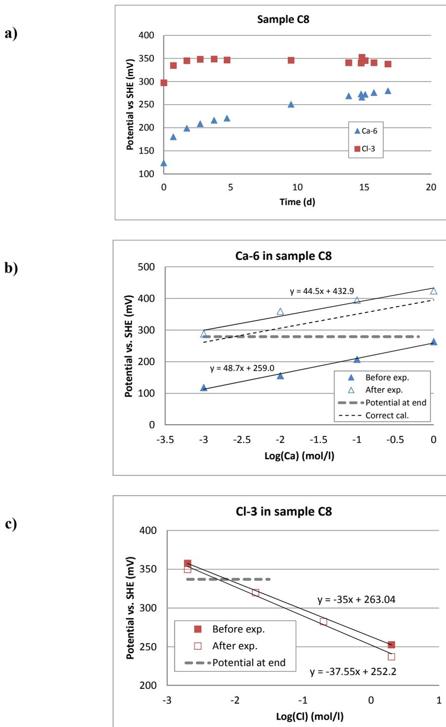
**Figure A7.** Measurement of calcium and chloride concentrations in the calcium bentonite sample C8. Dry density  $1.35 \text{ g/cm}^3$ , measured chloride concentration in bentonite  $0.0156 \text{ mg/g}$ .
