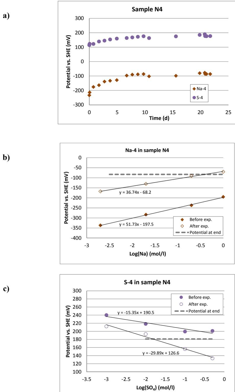
**Figure B4.** Measurement of sodium and sulphate concentrations in the sodium bentonite sample N4. Dry density  $1.64 \text{ g/cm}^3$ .
