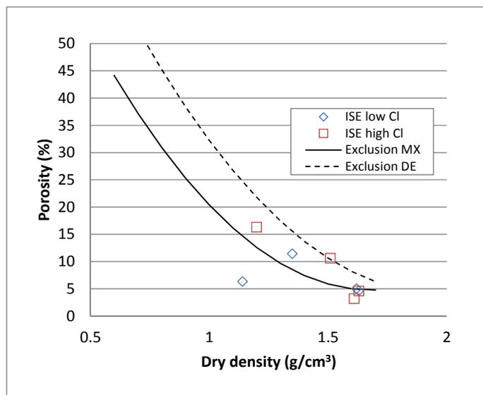
**Figure 16.** Chloride porosity based on the ISE and dispersion measurements of this study and exclusion measurement in MX-80 and Deponit of Muurinen (2009).
