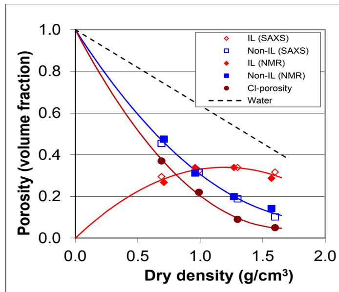
**Figure 2.** IL, non-IL, water and chloride porosity in MX-80 samples saturated with 0.1 M NaCl solution at different dry density. The IL and non-IL porosities were evaluated from SAXS and NMR measurements. The layer model was used for bentonite in SAXS modelling. The trend lines are IL:  $y = -0.2231x^2 + 0.541x$ ;  $R^2=0.981$ , non-IL:  $y = 0.223x^2 - 0.905x + 1$ ;  $R^2 = 0.997$ , Cl porosity:  $y = 0.337x^2 - 1.133x + 1$ ;  $R^2=0.999$  (Muurinen and Carlsson 2013).
