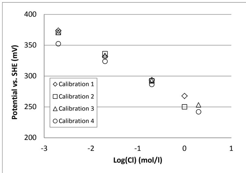
**Figure 6.** Potentials of a chloride electrode as a function of the logarithm of the chloride concentration of the  $\text{CaCl}_2$  solution in four subsequent calibrations. In the bentonite measurements the electrode was between the calibrations 1 – 2 and 3 – 4.
