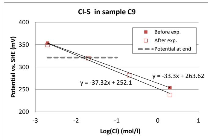
**Figure A8.** Measurement of calcium and chloride concentrations in the calcium bentonite sample C9. Dry density  $1.62 \text{ g/cm}^3$ , measured chloride concentration in bentonite  $0.0150 \text{ mg/g}$ .
