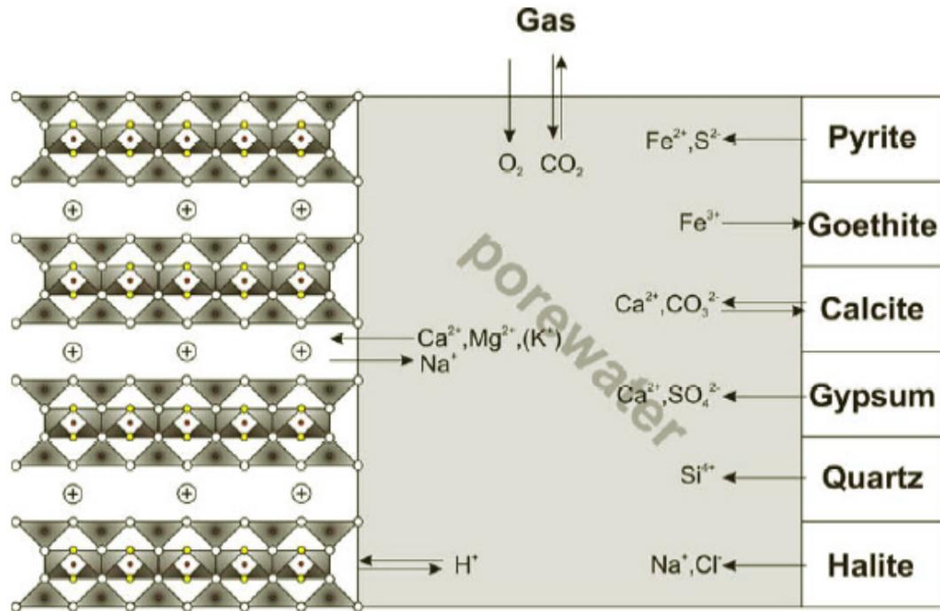
**Figure 3.** Schematic illustration of geochemical equilibrium processes used in modelling by Luukkonen (2004). The montmorillonite layering and interlayer sites are seen on the left, the mineral equilibria on the right and the entrapped gases on the top.
