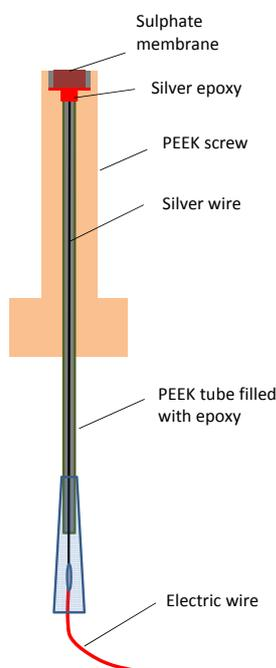
**Figure 7.** Structure of the sulphate electrode.
