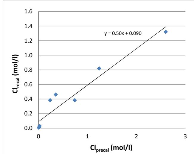
**Figure 12.** Comparison of the chloride concentration determined with ISEs using the calibration before the experiment ( $Cl_{precal}$ ) and after the experiment ( $Cl_{recaI}$ ).
