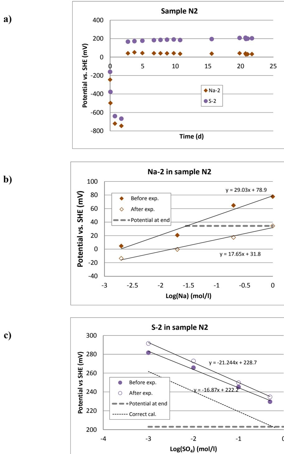
**Figure B2.** Measurement of sodium and sulphate concentrations in the sodium bentonite sample N2. Dry density  $1.66 \text{ g/cm}^3$ .
