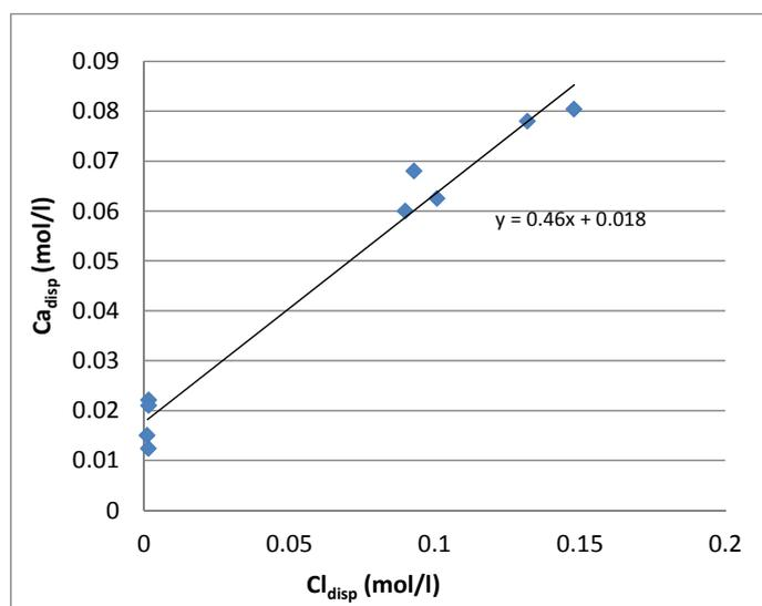
**Figure 14.** Presentation of the calcium concentrations as a function of chloride concentration in the bentonite. The concentrations were determined with the dispersion method and calculated per the total porewater volume.
