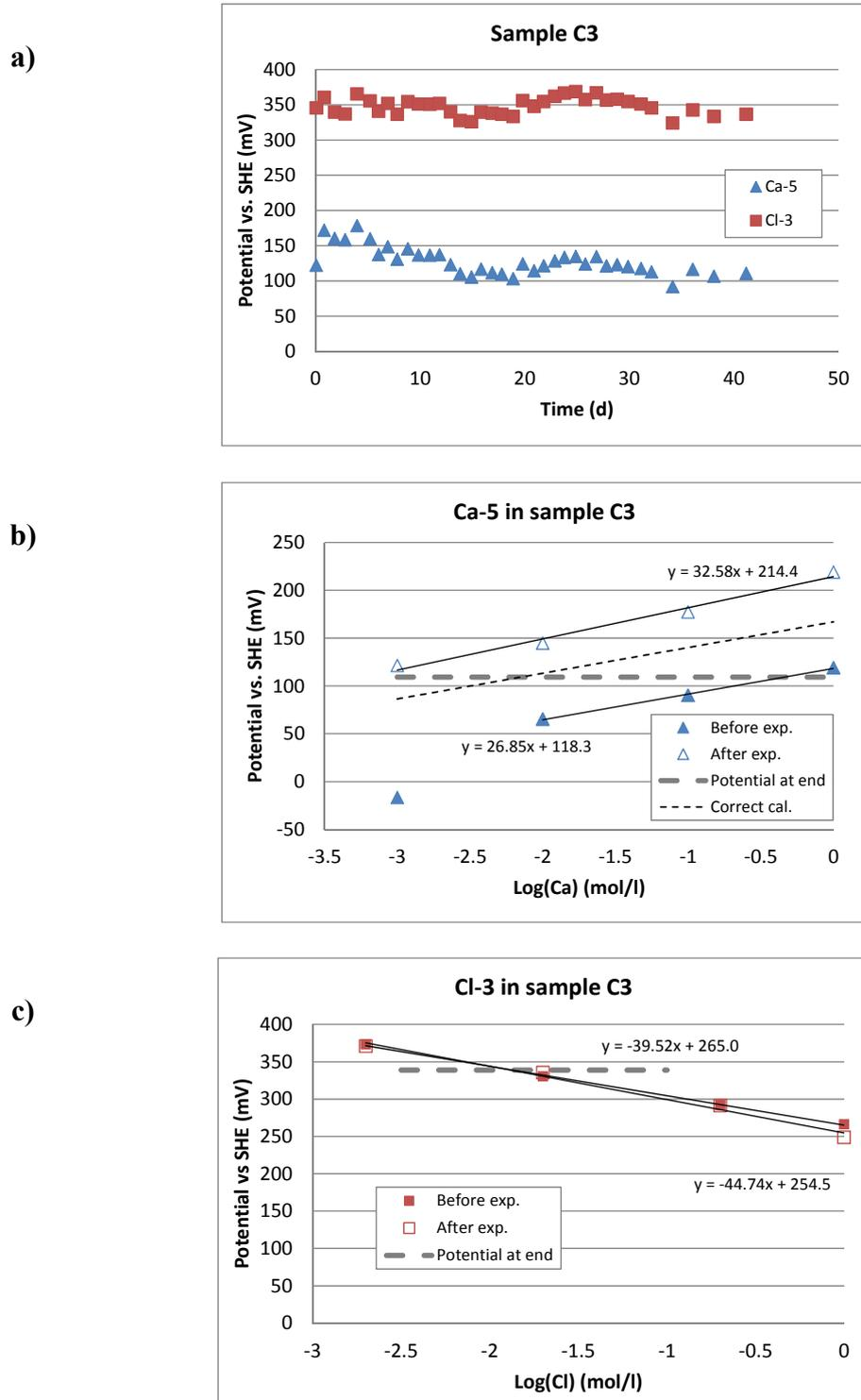
**Figure A2.** Measurement of calcium and chloride concentrations in the calcium bentonite sample C3. Dry density  $1.14 \text{ g/cm}^3$ , measured chloride concentration in bentonite  $0.0294 \text{ mg/g}$ .
