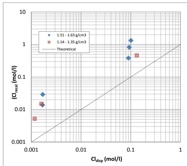
**Figure 13.** Comparison of the chloride concentrations in bentonite determined with ISE ( $Cl_{recaI}$ ) and dispersion method ( $Cl_{disp}$ ). The ISE values are based on the calibration after the experiment. The densities of the bentonite samples are given in the legend.
