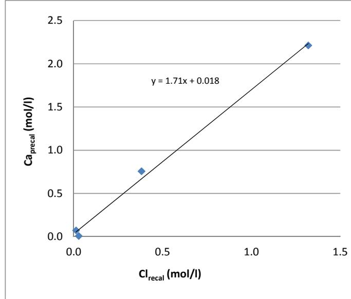
**Figure 15.** Comparison of the calcium and chloride concentrations determined with ISEs in the high-density bentonites. The calcium concentrations are based on the pre-calibration and chloride concentration on the re-calibration curves.
