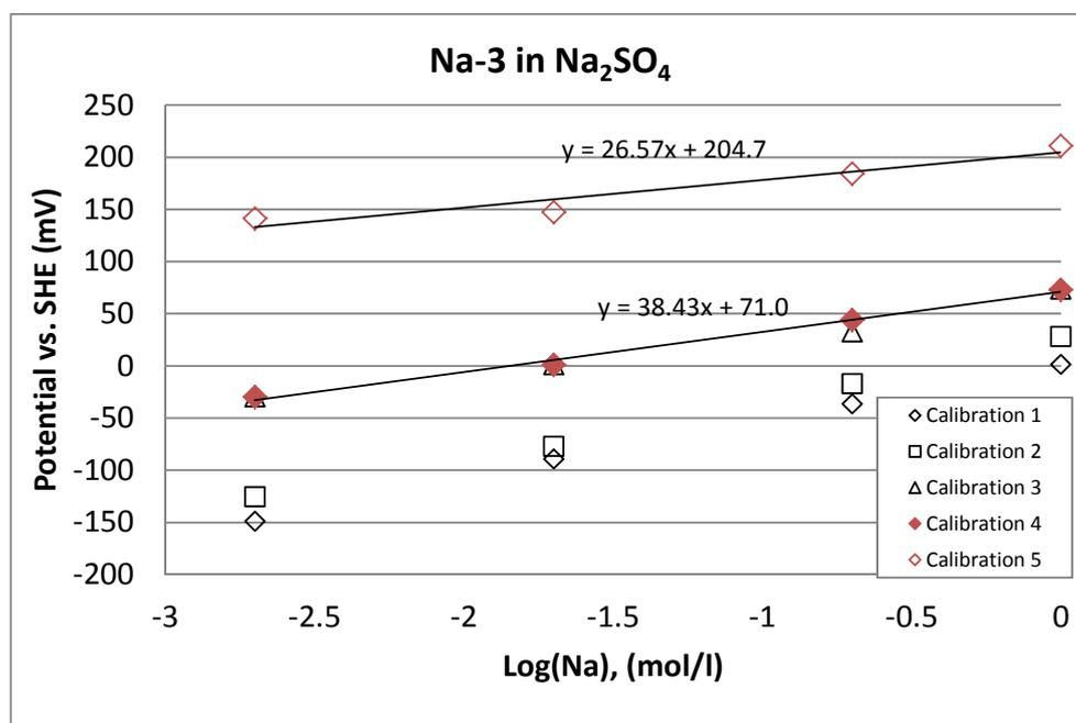
**Figure 9.** The potential of a sodium electrode as a function of the logarithm of the sodium concentration in the  $\text{Na}_2\text{SO}_4$  solution in repeated calibrations. The numbers of the measurements are given in the legend. The membrane was polished after the second calibration and in the bentonite measurement the electrode was between the calibrations 4 – 5.
