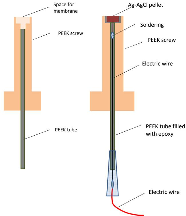
**Figure 5.** Structure of the chloride electrode. On the left is the electrode body and on the right the complete electrode.
