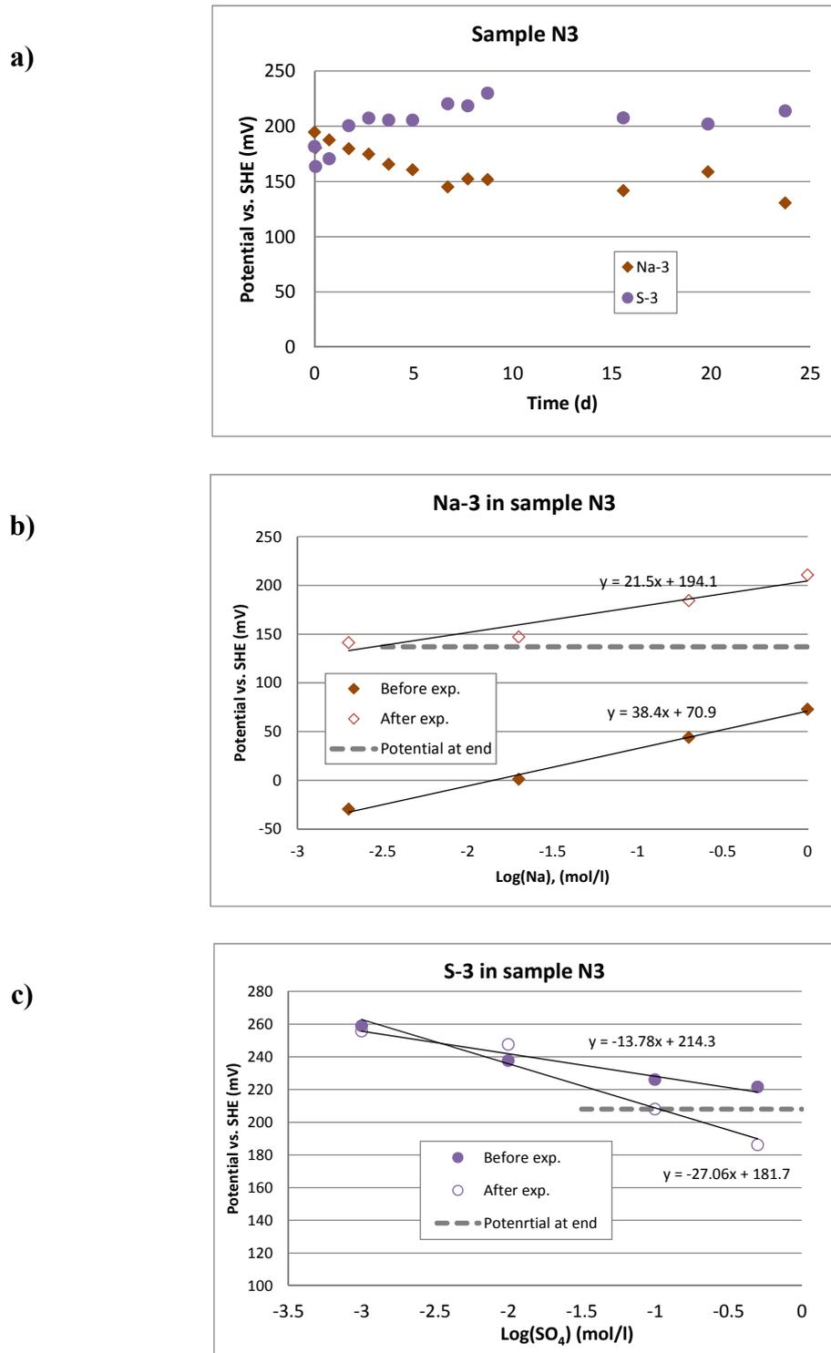
**Figure B3.** Measurement of sodium and sulphate concentrations in the sodium bentonite sample N3. Dry density  $1.21 \text{ g/cm}^3$ .
