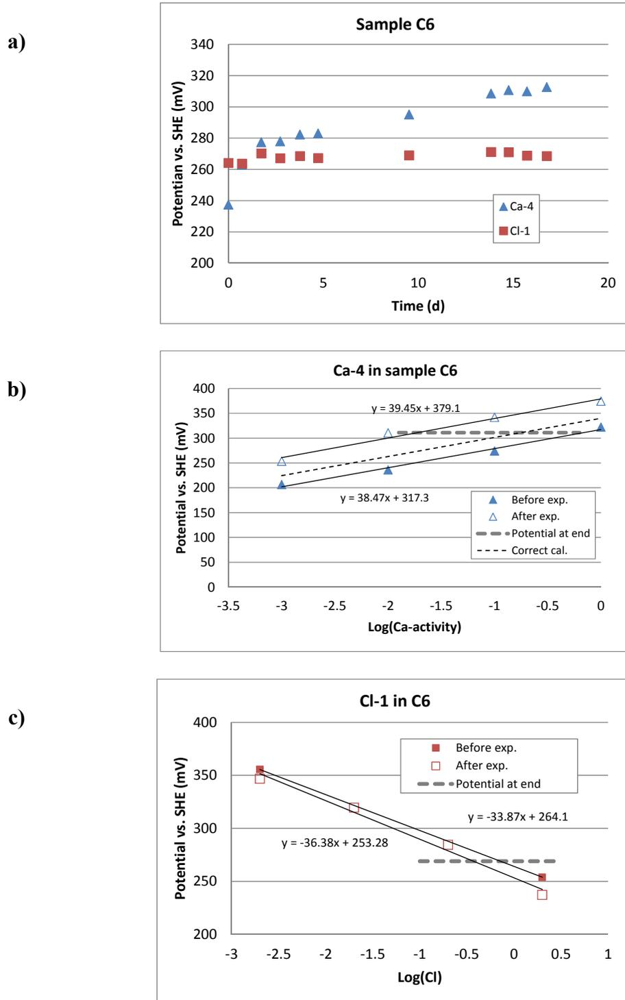
**Figure A5.** Measurement of calcium and chloride concentrations in the calcium bentonite sample C6. Dry density  $1.51 \text{ g/cm}^3$ , measured chloride concentration in bentonite  $0.955 \text{ mg/g}$ .
