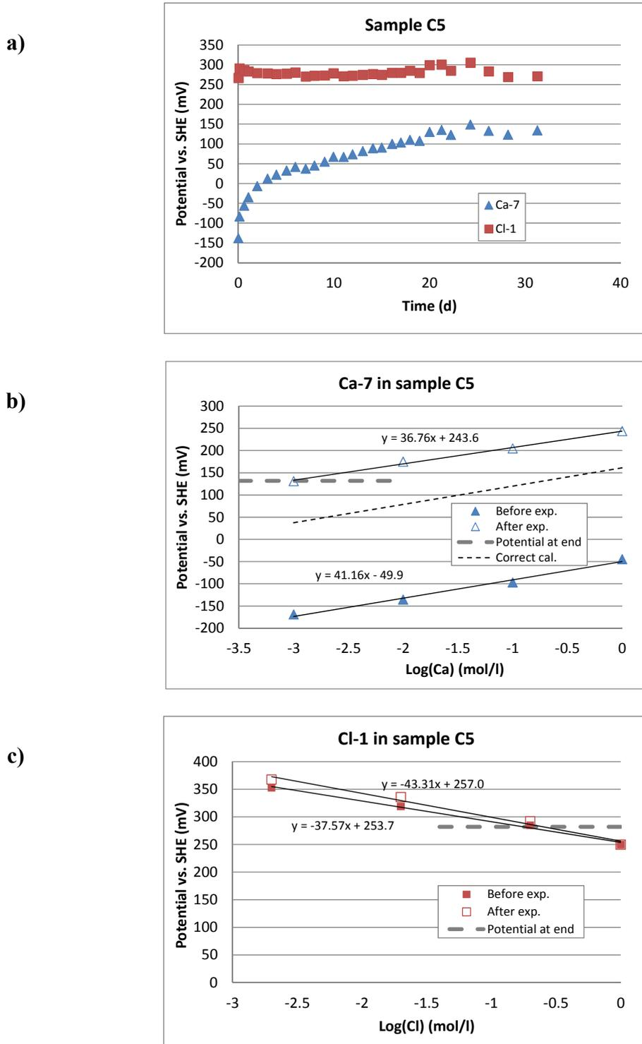
**Figure A4.** Measurement of calcium and chloride concentrations in the calcium bentonite sample C5. Dry density  $1.20 \text{ g/cm}^3$ , measured chloride concentration in bentonite  $2.22 \text{ mg/g}$ .
