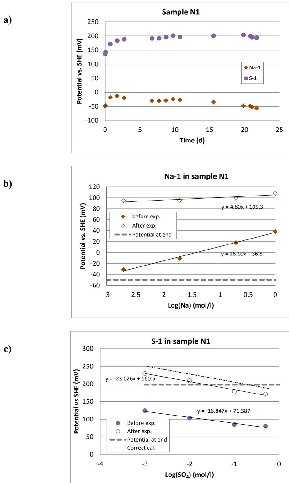
**Figure B1.** Measurement of sodium and sulphate concentrations in the sodium bentonite sample N1. Dry density  $1.20 \text{ g/cm}^3$ .
