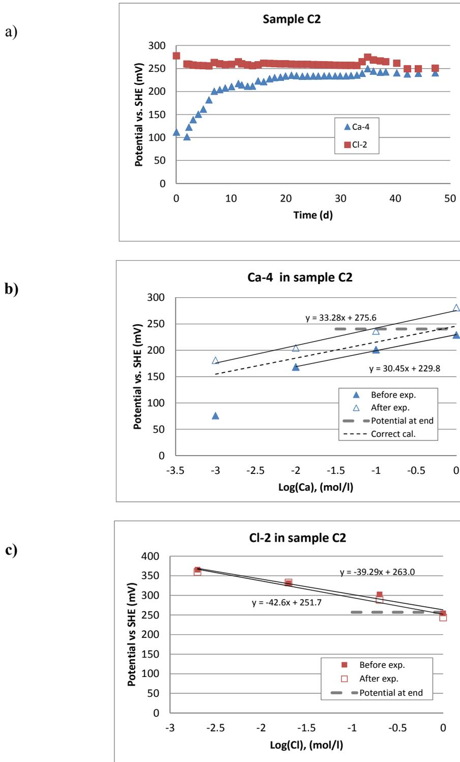
**Figure A1.** Measurement of calcium and chloride concentrations in the calcium bentonite sample C2. Dry density  $1.61 \text{ g/cm}^3$ , measured chloride concentration in bentonite  $0.916 \text{ mg/g}$ .
