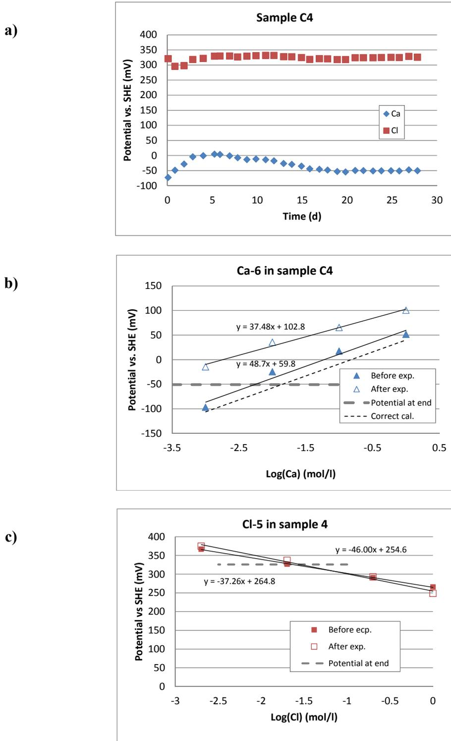
**Figure A3.** Measurement of calcium and chloride concentrations in the calcium bentonite sample C4. Dry density  $1.63 \text{ g/cm}^3$ , measured chloride concentration in bentonite  $0.0156 \text{ mg/g}$ .
