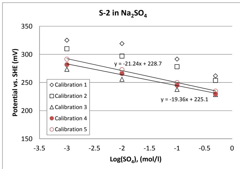
**Figure 8.** The potential of a sulphate electrode as a function of the logarithm of the sulphate concentration in  $\text{Na}_2\text{SO}_4$  solutions in repeated calibrations. The numbers of the measurements are given in the legend. The membrane was polished after the second measurement. In the bentonite measurement the electrode was between the calibrations 4 – 5.
