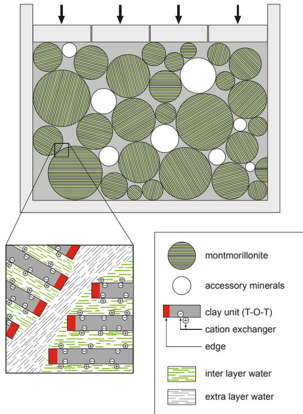
**Figure 1.** Generalized microstructure of MX-80 (Wersin 2003).
