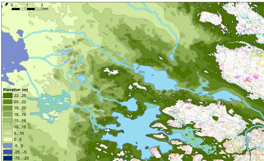
Figure 4. A possible map of the Olkiluoto site about 5900 years after present (25 m land uplift, omitting changes in sea level due to climate change).
