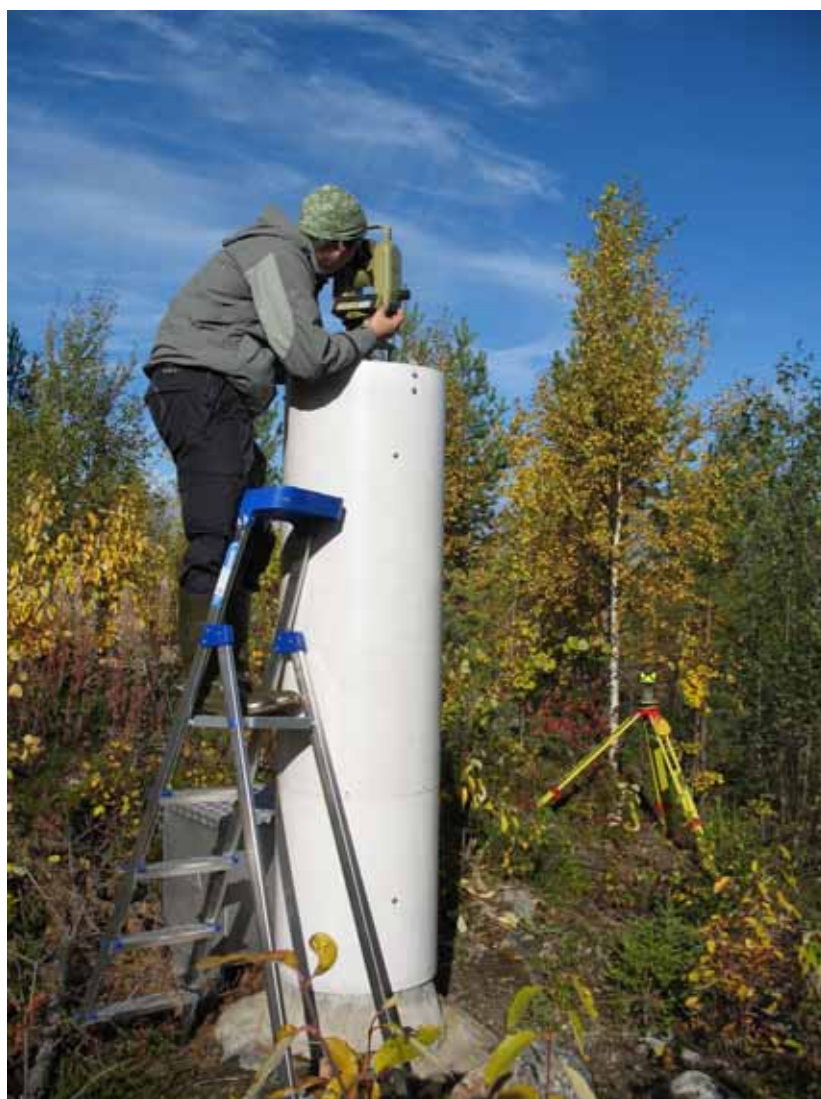
Figure 6-1. The distances between pillars and control markers were measured using the Distomat Wild DI2002 EDM instrument. The horizontal and vertical angles were observed with the theodolite Theomat Wild T2002. (Photograph J. Puupponen 2006.)
