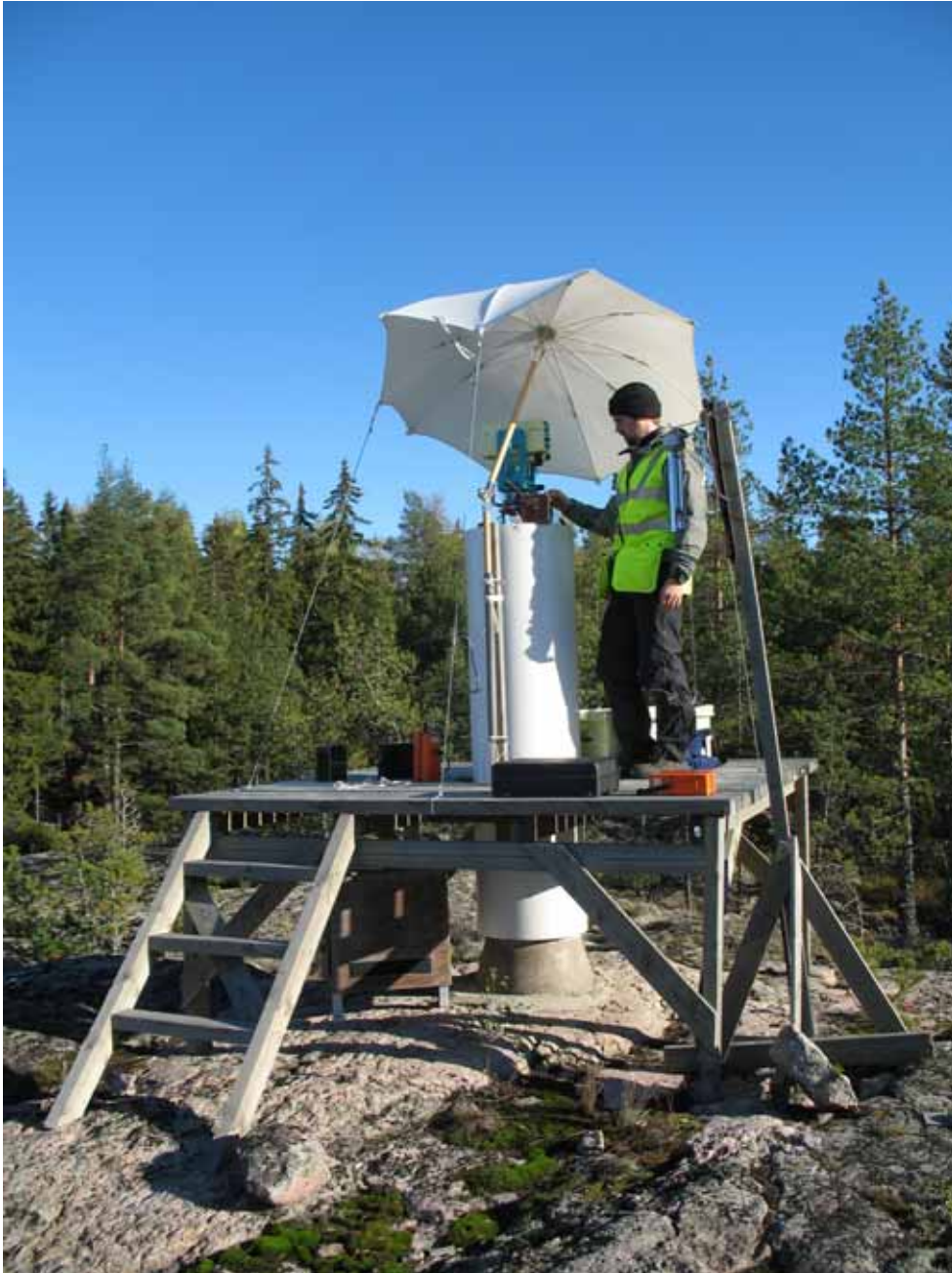
Figure 5-1. The mekometer Kern ME5000 at the pillar GPS8 during baseline observation on October 2006. (Photograph T. Ahola 2006.)
