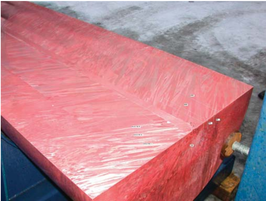
A copper billet machined axially to the very centre to find any casting defects.
