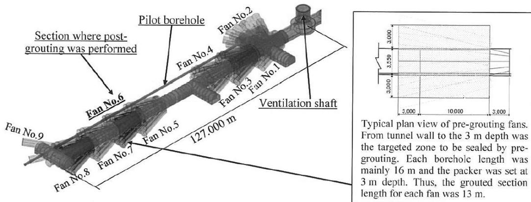
**Fig. 6 Schematic layout of pre-excavation grouting fans<sup>6)</sup>**
