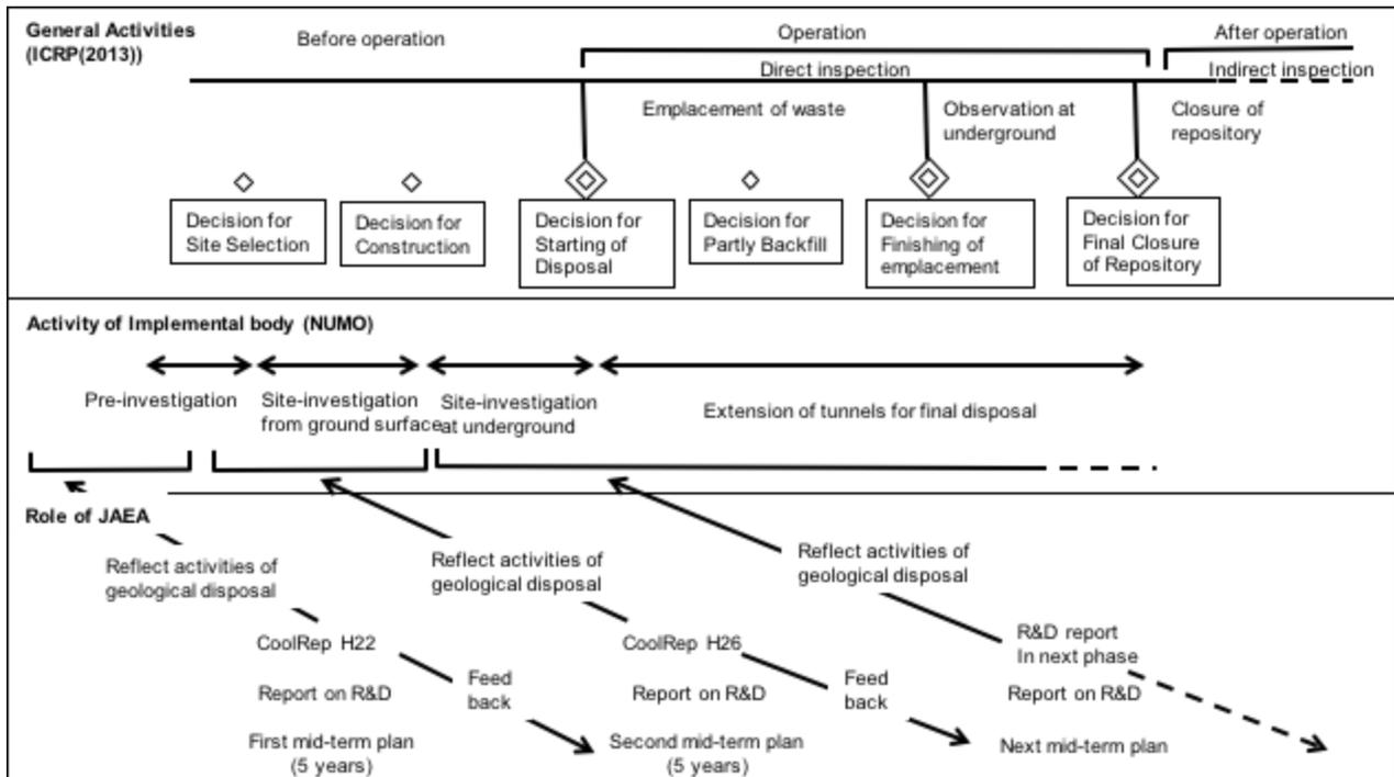
**Fig.3 The interrelationship between the progress of geological disposal, and the activities of the implemental body (NUMO) and JAEA R&D activity<sup>4)</sup>**
