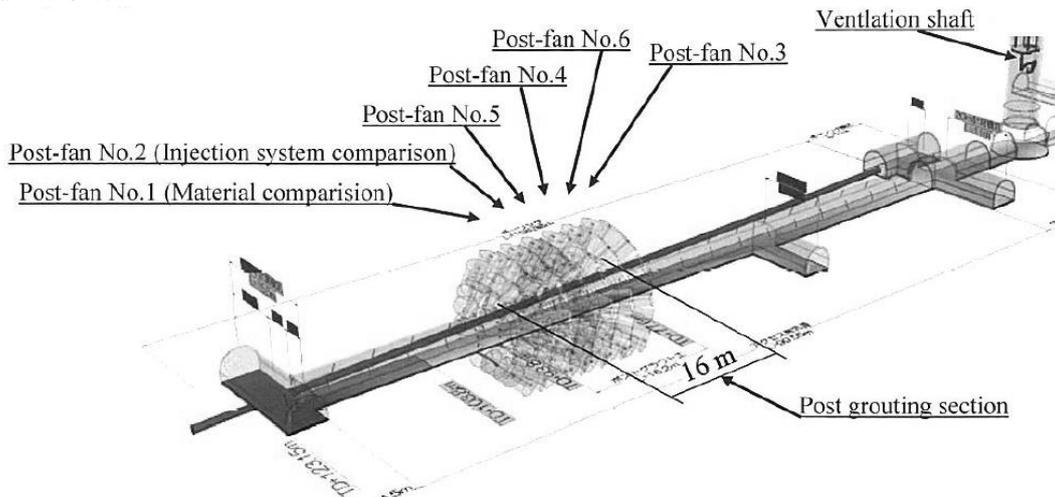
**Fig.7 Schematic layout of post-excavation grouting fans**<sup>6)</sup>
