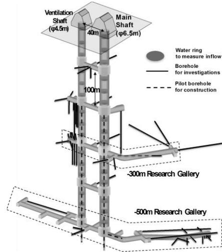
**Fig.2 Schematic layout for investigation and drift in MIU<sup>3)</sup>**
