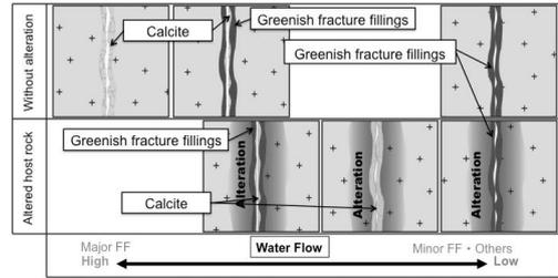
**Fig.4 Conceptual model for fractures observed in MIU<sup>5)</sup>**
