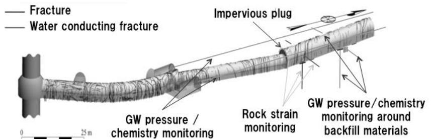
**Fig.8 Fracture distribution and monitoring layout at groundwater recovery experiment site**<sup>3)</sup>
