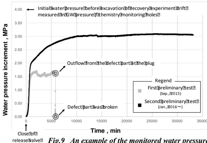
**Fig.9** An example of the monitored water pressure recoveries in the groundwater recovery experiment drift during the preliminary tests
