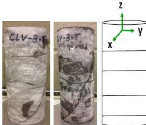
Figure 3-5. Failure mode of specimen CLV-3-T and the 3D sketch corresponding to the seismic velocity measurement.
