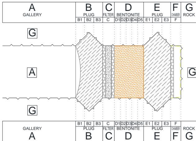
Figure 1 - Scheme of EPSP (measurement profiles)
