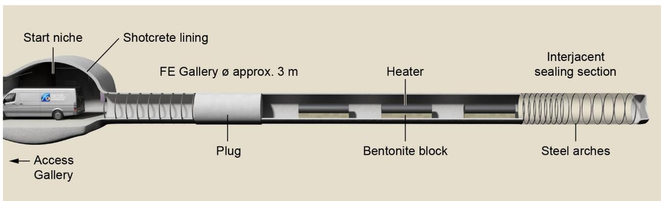
Figure 1: Visualisation of the FE/LUCOEX experiment at the Mont Terri URL representing a section of the repository tunnel (backfill not shown).
