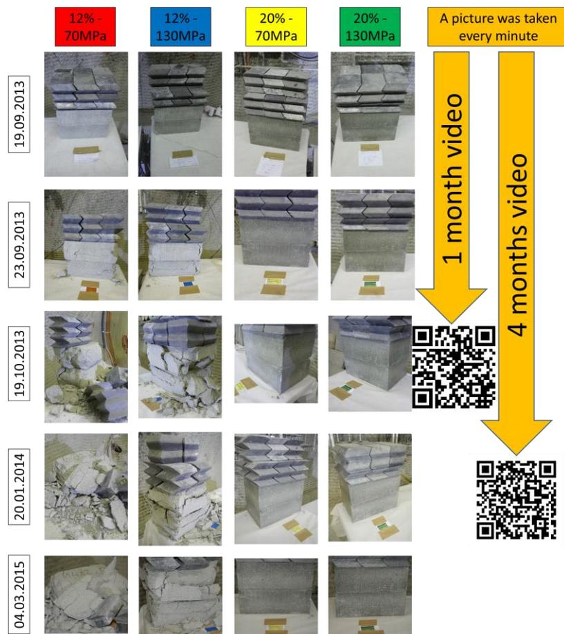
Figure 5: Behaviour of compacted bentonite blocks exposed to a relative humidity varying between 60 % and 85 % for different production parameters (water content and compaction pressure are indicated at the top of the figure).
