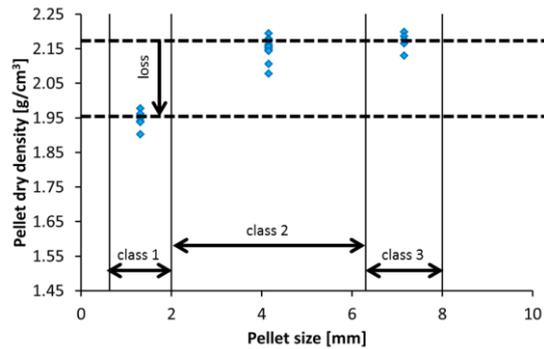
Figure 4: Pellet dry density measured on material sieved out from mixture 3 at ETH using a GeoPyc for three different sizes of pellets (1: between 0.63 mm and 2 mm; 2: between 2 mm and 6.3 mm and 3: between 6.3 mm and 8 mm).
