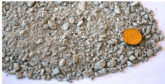
Figure 2: Photo of the granulated bentonite mixture (GBM) produced for the FE experiment.
