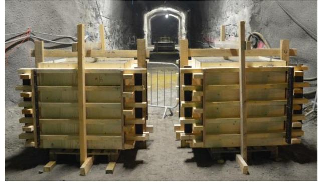
**Figure 2. Example of 1m<sup>3</sup> quality control blocks produced with POPLU experiment.**
