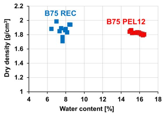
Figure 3-4 - Comparison of dry densities of both final products.
