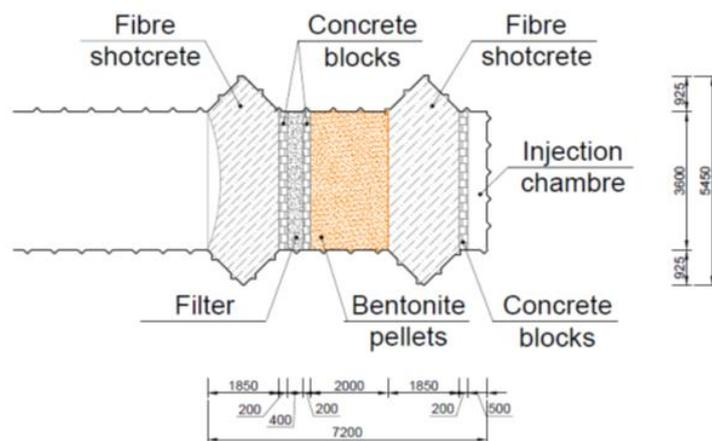
*Figure 1-1- Scheme of the conceptual design of the EPSP. Dimensions in mm.
