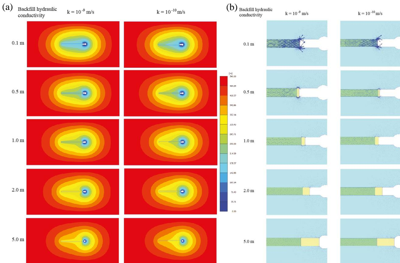
**Figure 2. (a) Pressure head distribution for different sealing length, left:  $k=10^{-9}$  m/s of the backfill hydraulic conductivity; right:  $k=10^{-10}$  m/s of the backfill hydraulic conductivity and (b) Velocity distribution near the plug for different sealing length, left:  $k=10^{-9}$  m/s of the backfill hydraulic conductivity; right:  $k=10^{-10}$  m/s of the backfill hydraulic conductivity**
