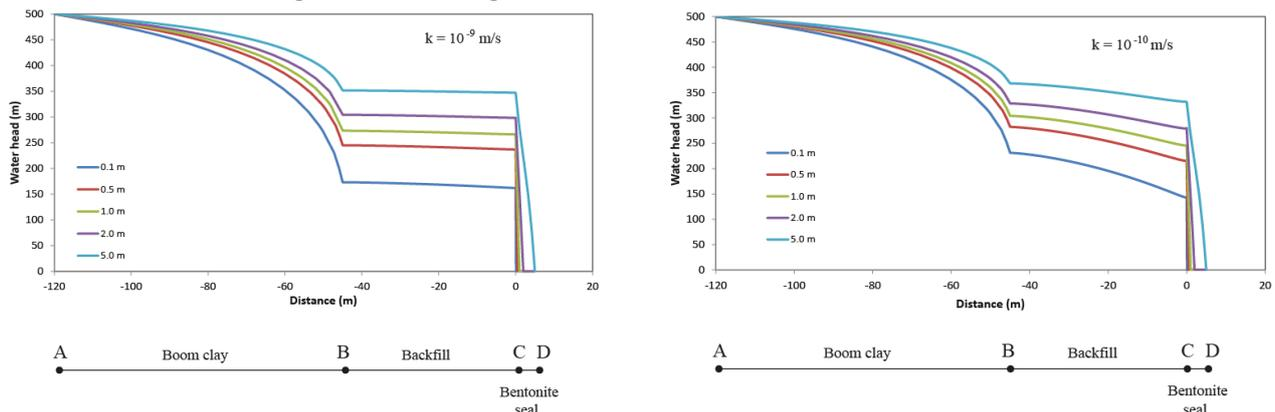
**Figure 3. Pressure head distribution along the tunnel for different sealing length, left:  $k=10^{-9}$  m/s of the backfill hydraulic conductivity; right:  $k=10^{-10}$  m/s of the backfill hydraulic conductivity**
