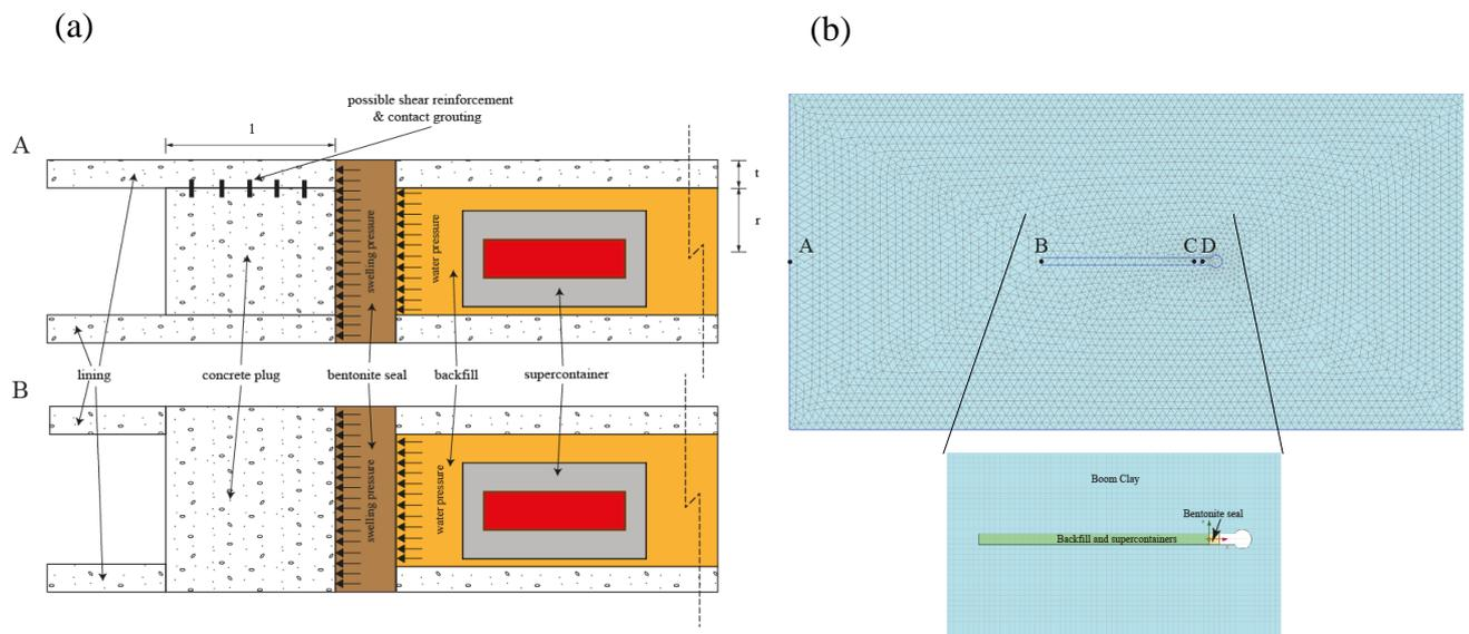
**Figure 1. (a) Two types of conceptual plug system design; A: with the concrete plug installed inside the tunnel lining, and B: with the tunnel lining removed locally where the concrete plug is installed and (b) The mesh and details of the deposition tunnel and plug system used for the hydraulic simulation**
