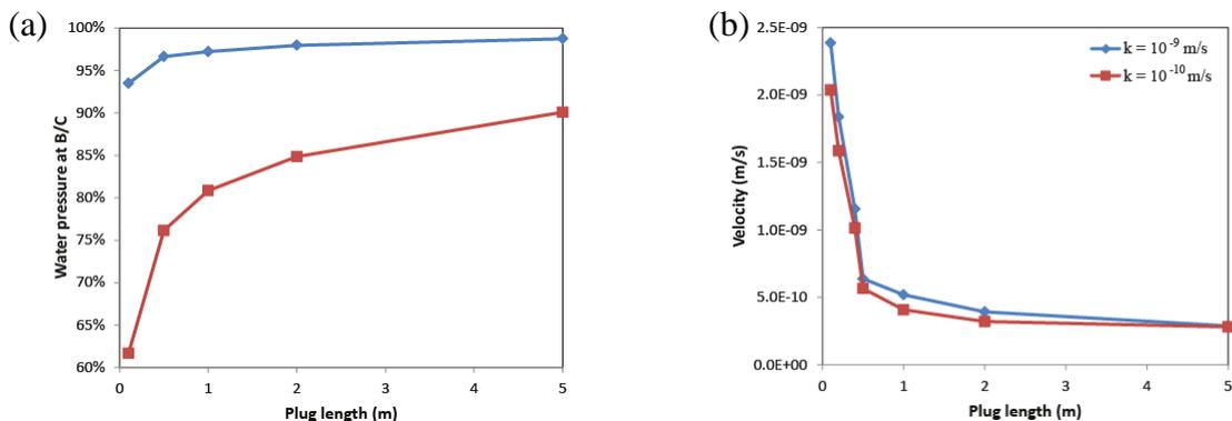
**Figure 4. (a) Percentage of water head taken by the plug verses sealing length for different backfill hydraulic conductivity; (b) Maximum velocity in the domain versus sealing length for different backfill hydraulic conductivity**
