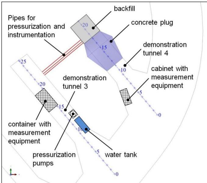
**Figure 1. Top view of POPLU monitoring system arranged in demonstration tunnels 3 and 4, including pressurization system and data collection measuring equipment.**
