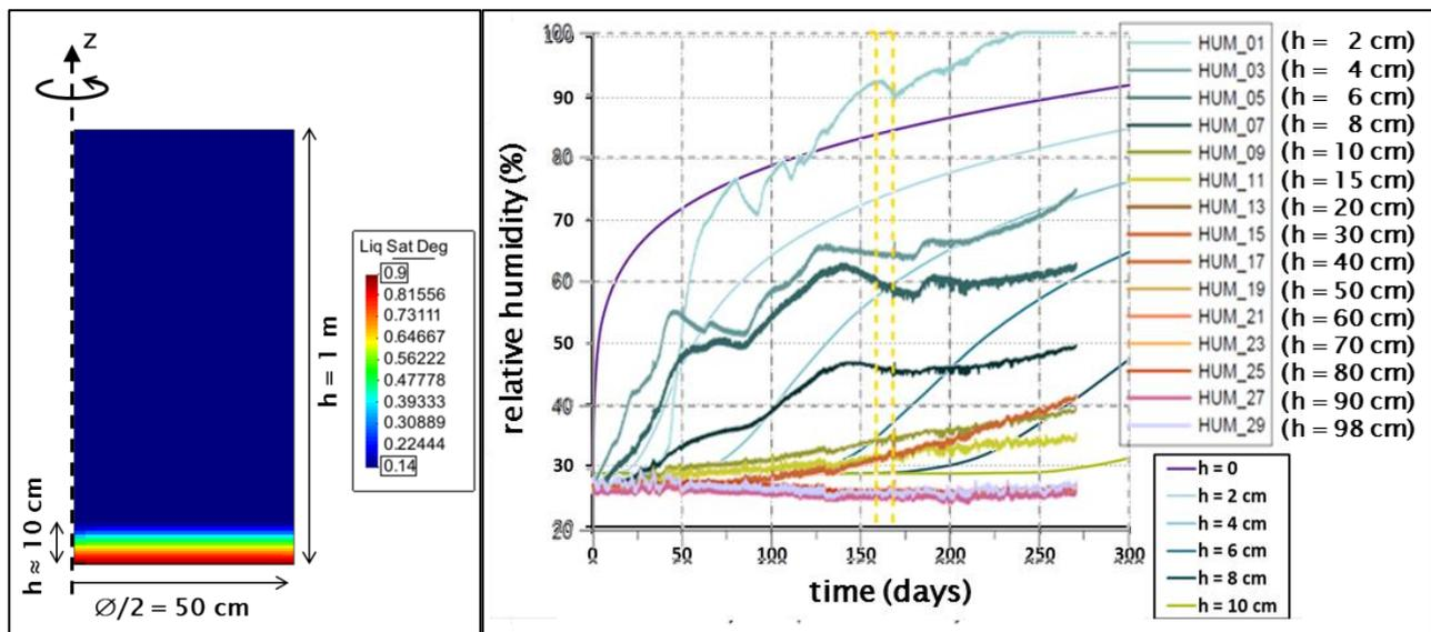
**Figure 4-1. Liquid saturation field at time 265 days and relative humidity changes at different heights in the lower part of REM: Comparison between measurements and preliminary 2D-axisymmetric simulations**
