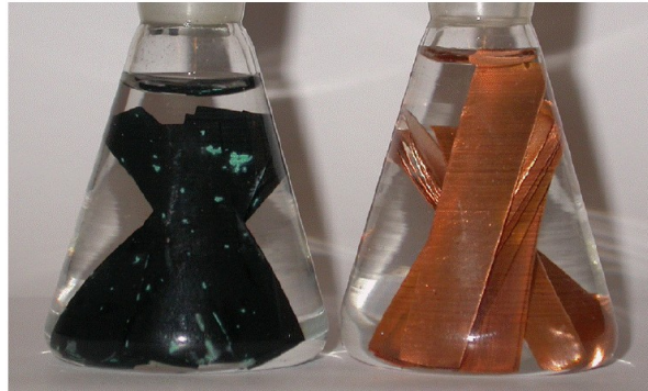
Figure 1: Experimental arrangement in which copper samples have been immersed in water in a glass container for 15 years. In the container on the left, hydrogen is allowed to diffuse from the bottle through a palladium membrane. The container on the right is completely sealed (Hultquist, 2008).
