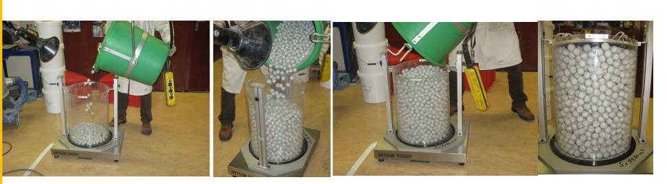
In a first time the best possible arrangement of the pellets dropped in the box is looked after, and for that purpose the effective bentonite density in the box is measured.
