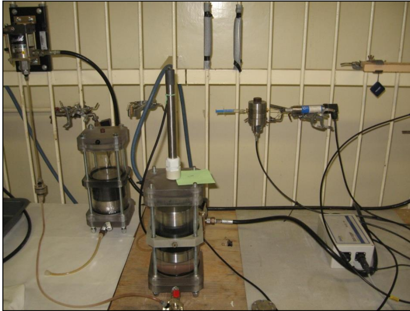
Figure 16 - Small-scale chamber for monitoring the saturation of bentonite
