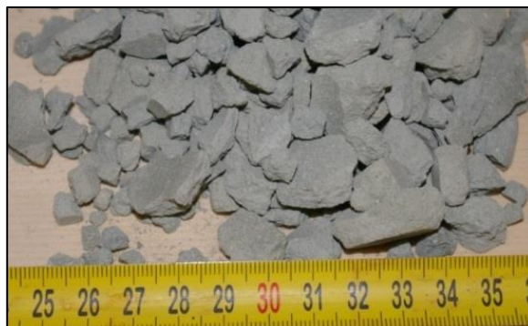
Figure 9 – Compacted bentonite B75_REC
