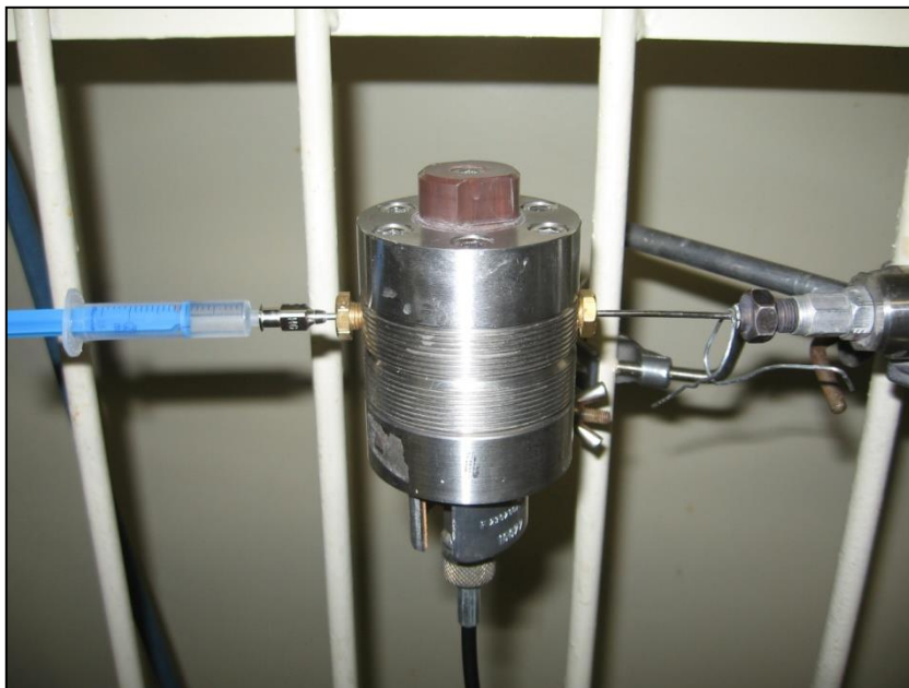
Figure 17 – Detail of drainage needles and sensors for the measurement of pore water pressure
