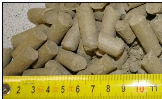
Figure 8 – Compacted bentonite pellets B75_PEL_12 from the roller compaction machine (Šťástka, 2013)
