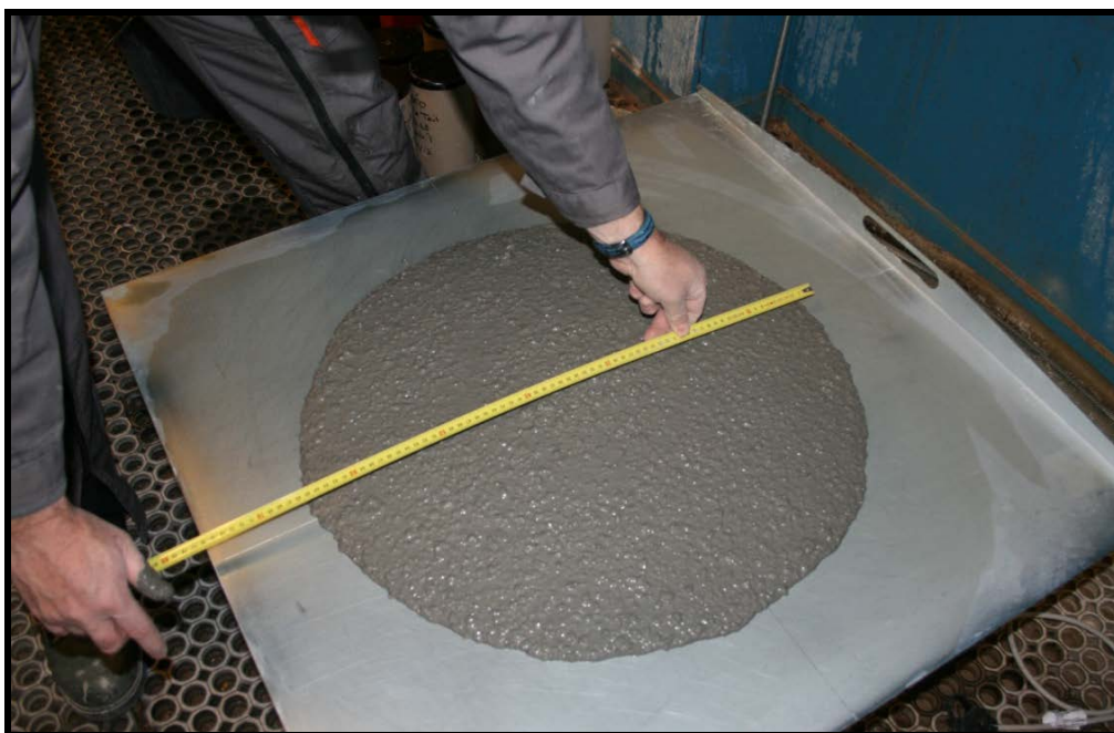
Figure 9: Slump test measurement.
