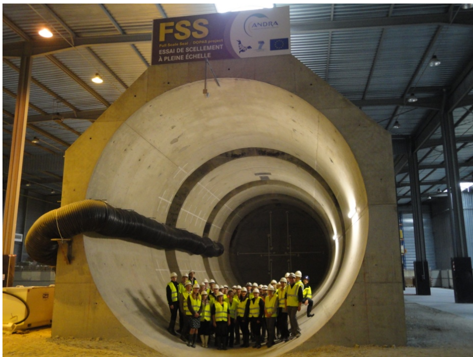
Figure 1. This Experiment 1. FSS drift model has been partly filled with concrete. Photo: Andra.
