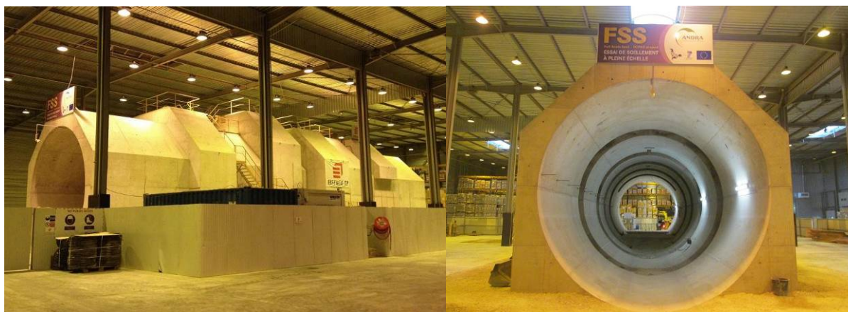
Figure 4: The FSS test box ready for seal construction
