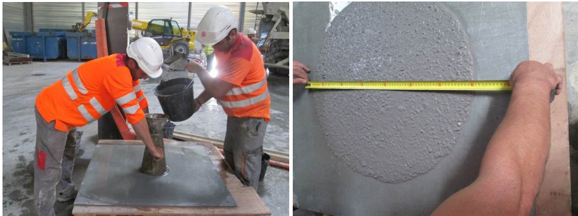
Figure 12: Concrete slump flow test - Abrams values remained between 55cm & 75cm
