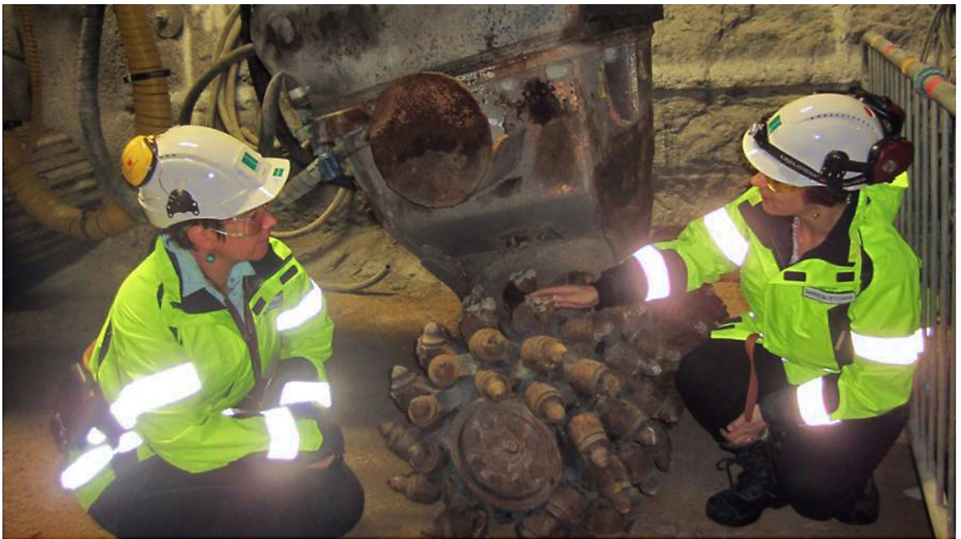
Production of plug location with grinding is a pioneering process. Johanna Hansen and Sanna Mustonen from Posiva are studying the wearing of the grinding tool. © Marjatta Palmu/DOPAS.
