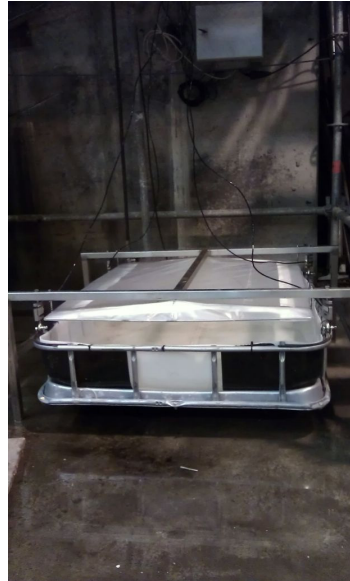
Figure 4-5. Left: The watertight weir. Right: Basin for weighing of leakage water outflow from the weir
