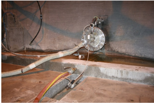
Figure 4-5. Left: The watertight weir. Right: Basin for weighing of leakage water outflow from the weir
