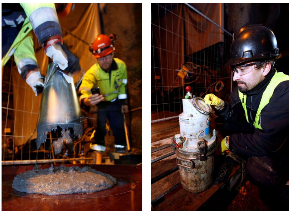
Figure 5-16. Clocking t_{500} while measuring slump flow (left), measuring air content (right).
