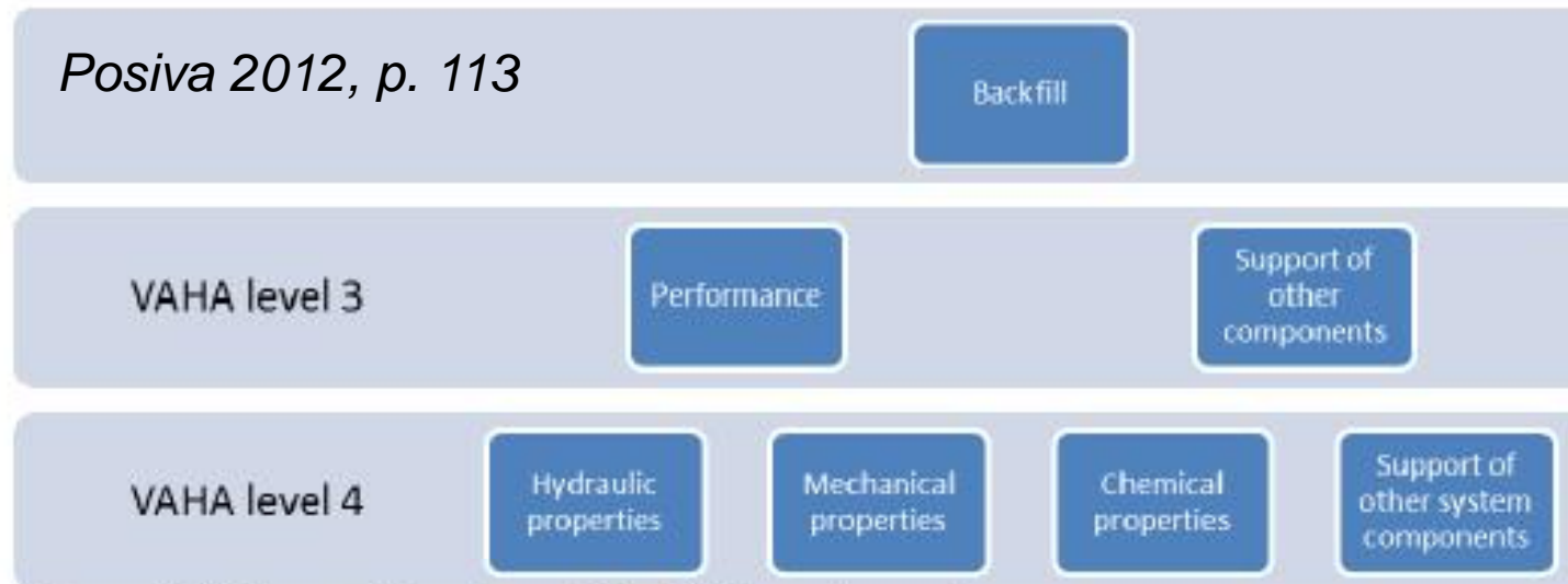
Figure 9-1. General structure of backfill requirements.
