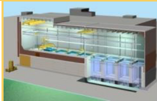
Interim storage of spent nuclear fuel
