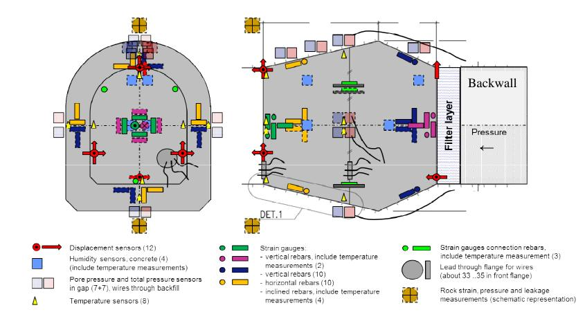
Values to be measured: temperature, humidity, strain, displacement, pressure, and water leakage.
