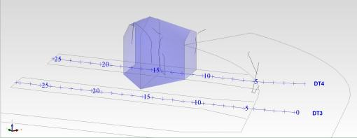
It was concluded that the criteria set for the plug location are fulfilled in the demonstration tunnel 4 in general and that the suggested chainage 11 -17 m is suitable for the plug location.
