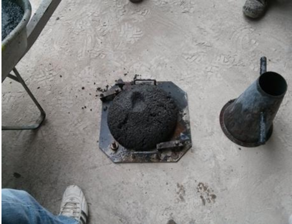
Verification of slump flow after 2 hours
