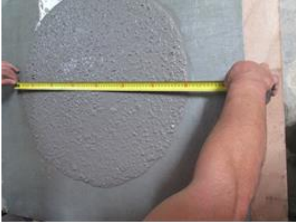
Slump control 2 hours after fabrication (has to be between 55 cm to 75 cm)
