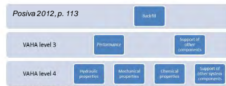
Figure 9-1. General structure of backfill requirements.
