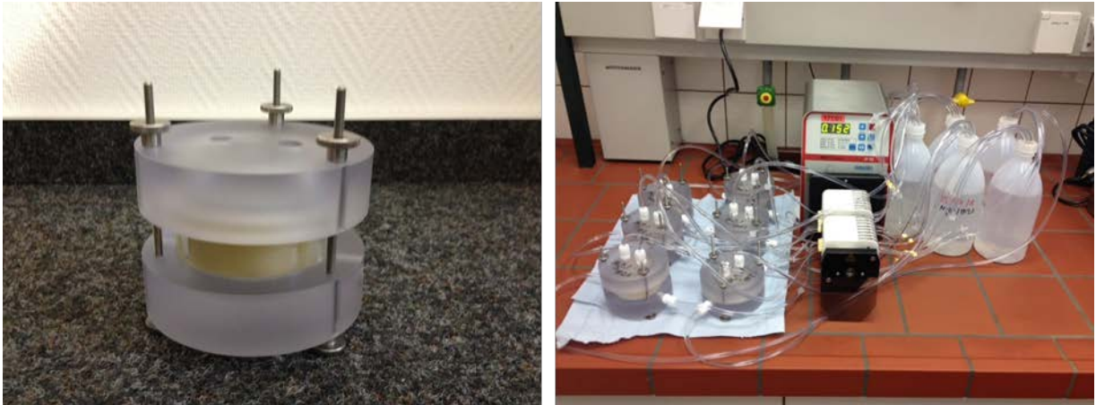
Fig. 5-8 Diffusion cell with inserted sample (left) and layout of through-diffusion experiments during phase 2 of experiment (right)
