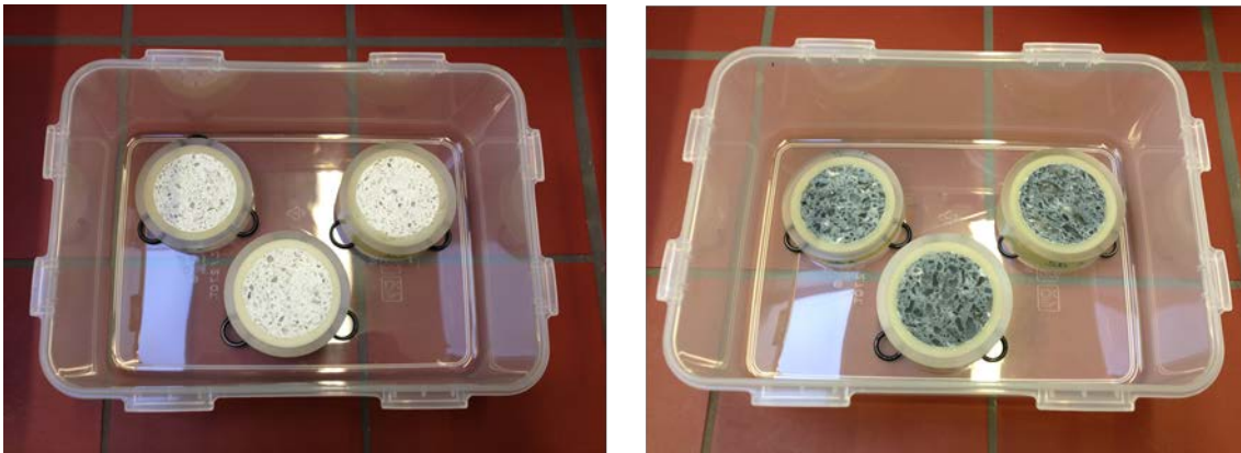
Fig. 5-7 Samples in first phase of through-diffusion experiments before solutions were admitted. sorel concrete (left) and salt concrete (right)
