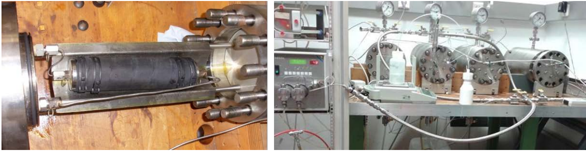
Fig. 5-11 Coated sample in an isostatic cell (left) and cell arrangement (right)
