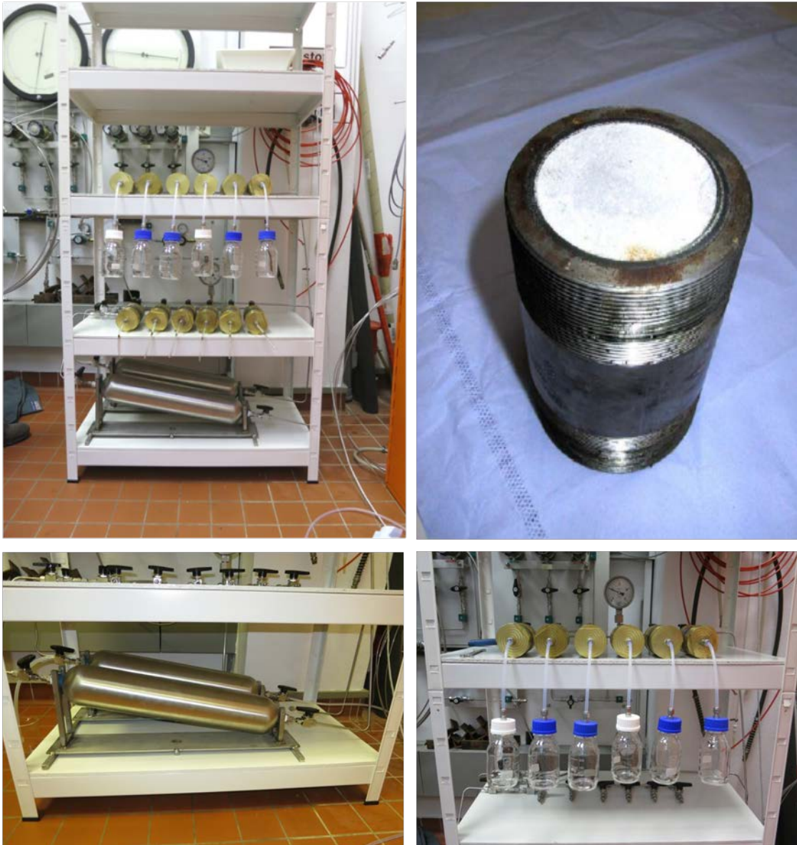
Fig. 4-6 Experimental set up of advection experiment in laboratory
