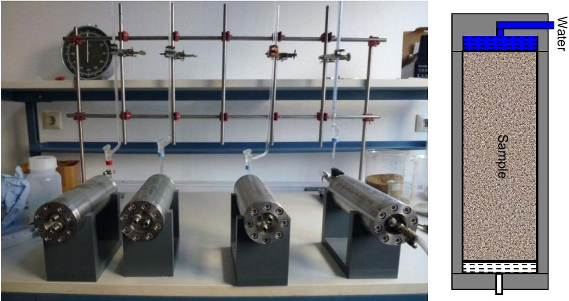
Fig. 4.5 Test layout for water saturation of the seal materials in steel cylinders
