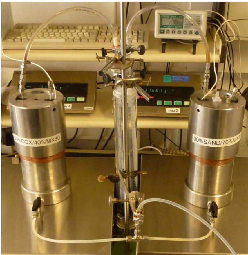
Fig. 4.19 Setup of the small-scale borehole sealing tests in steel cylinders with compacted blocks of claystone-bentonite and bentonite-sand mixtures
