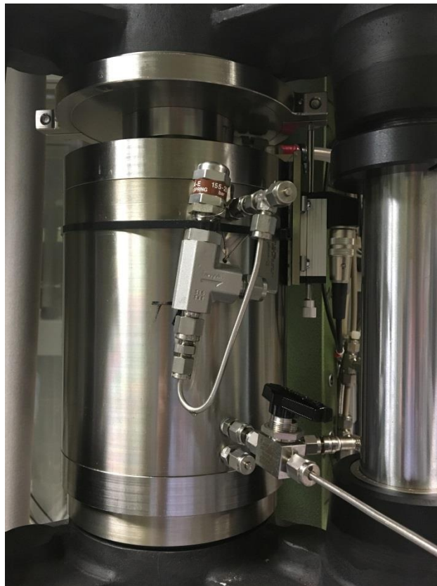
Fig. 3.25 Steel cylinder for individual oil pressure built-up on a salt concrete sample
