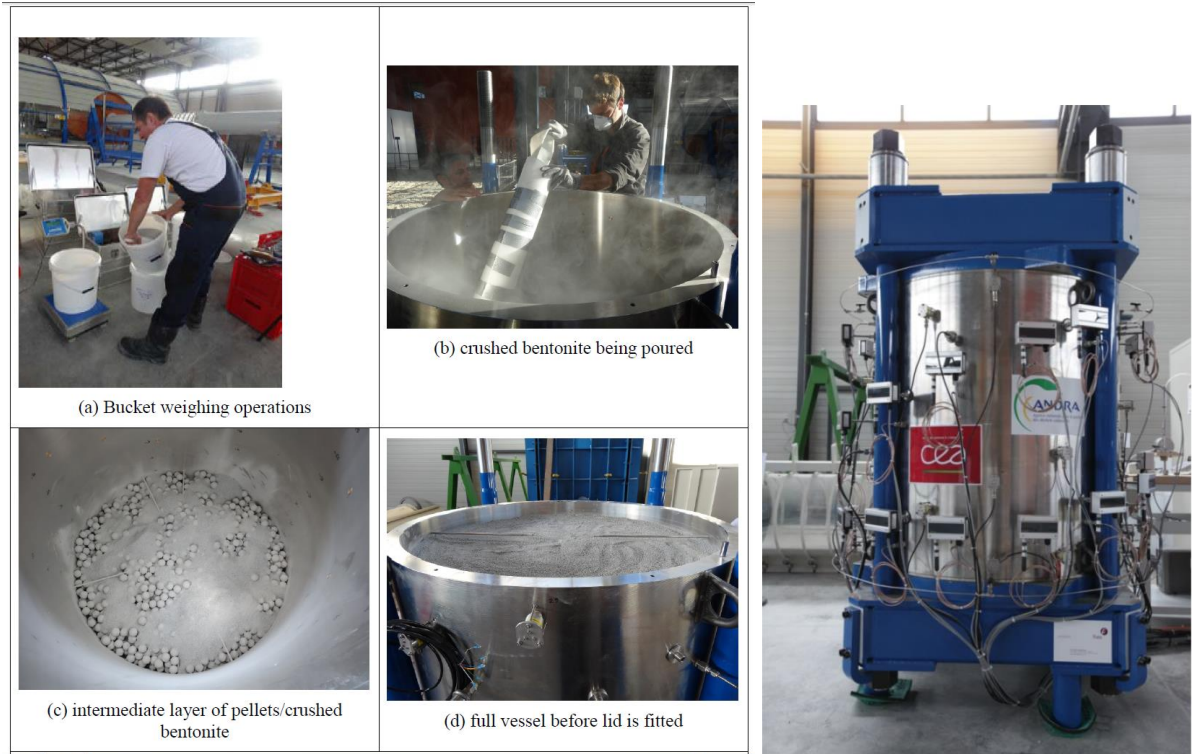
Fig. 6.18: Principal REM installation phases
