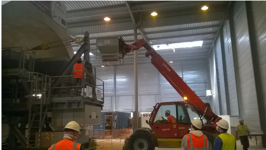
Figure 2: Transferring the bentonite into the filling machine using forklift trucks.
