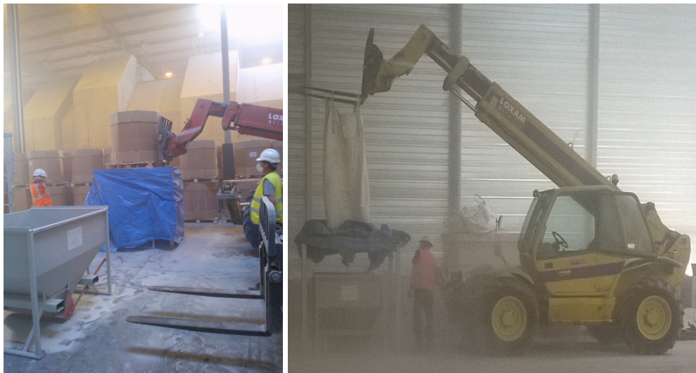
Figure 1: Emptying of octabin containing bentonite pellets (left) and bag with bentonite powder (right) into hoppers.
