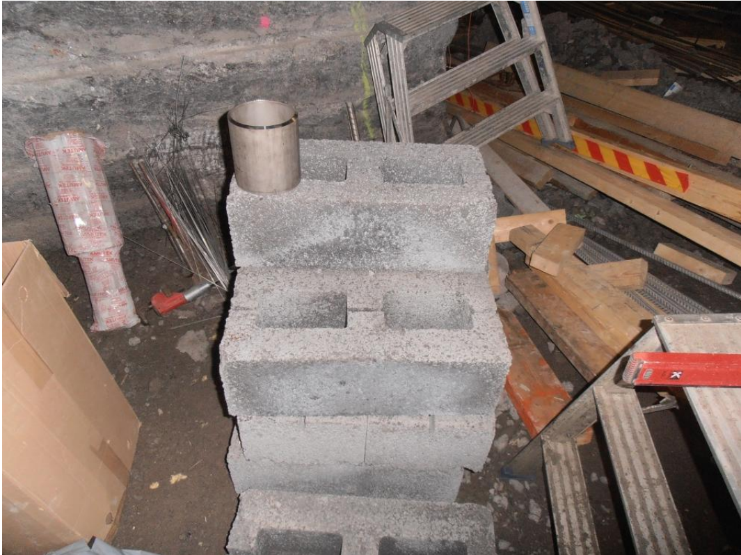
Figure 4.4 Lightweight low-pH concrete blocks (hollow LECA ® ), of the type that make up the filter layer. Photo by Michal Roll.
