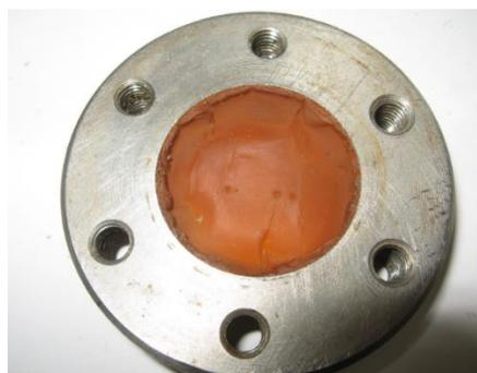
Figure 34 - Sample of a polyurethane-based grouting material subjected to the permeability test.
