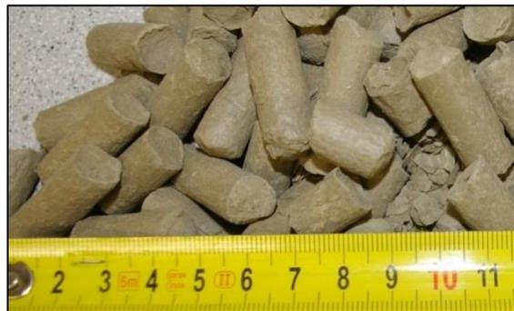
Figure 10 – Compacted bentonite pellets B75\_PEL\_12 from the roller compaction machine (Štástka, 2013)
