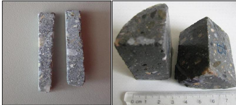
Figure 58- Concrete samples for porosity measurements, on left - samples for mercury intrusion porosimetry, on right - samples for water submersion method
