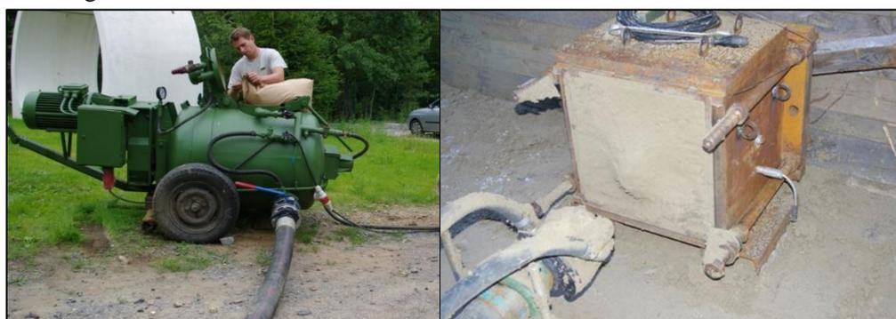
Figure 17 – The Mixokret machine for the spraying of bentonite pellets with crushed ice and the filling of the steel box for the medium-scale tests
