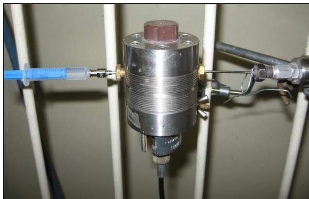
Figure 36 – Detail of drainage needles and sensors for the measurement of pore water pressure
