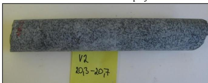
Figure 35 - Host rock sample; drilled core from borehole V2
