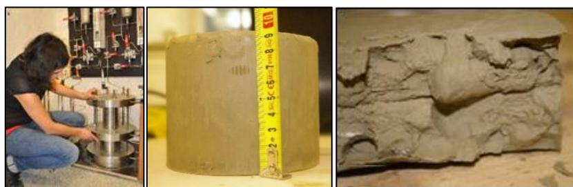
Figure 13 – A large cell and a pellet-form bentonite sample prior to and following testing
