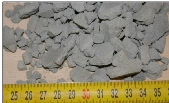
Figure 11 – Compacted bentonite B75\_REC
