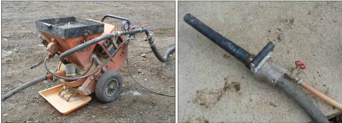
Figure 19 – Spraying machine SSB14 and a nozzle
