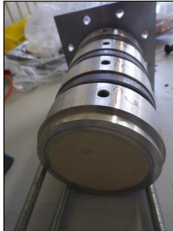
Figure 42 - The dismantling of the physical hydraulic model into individual cells
