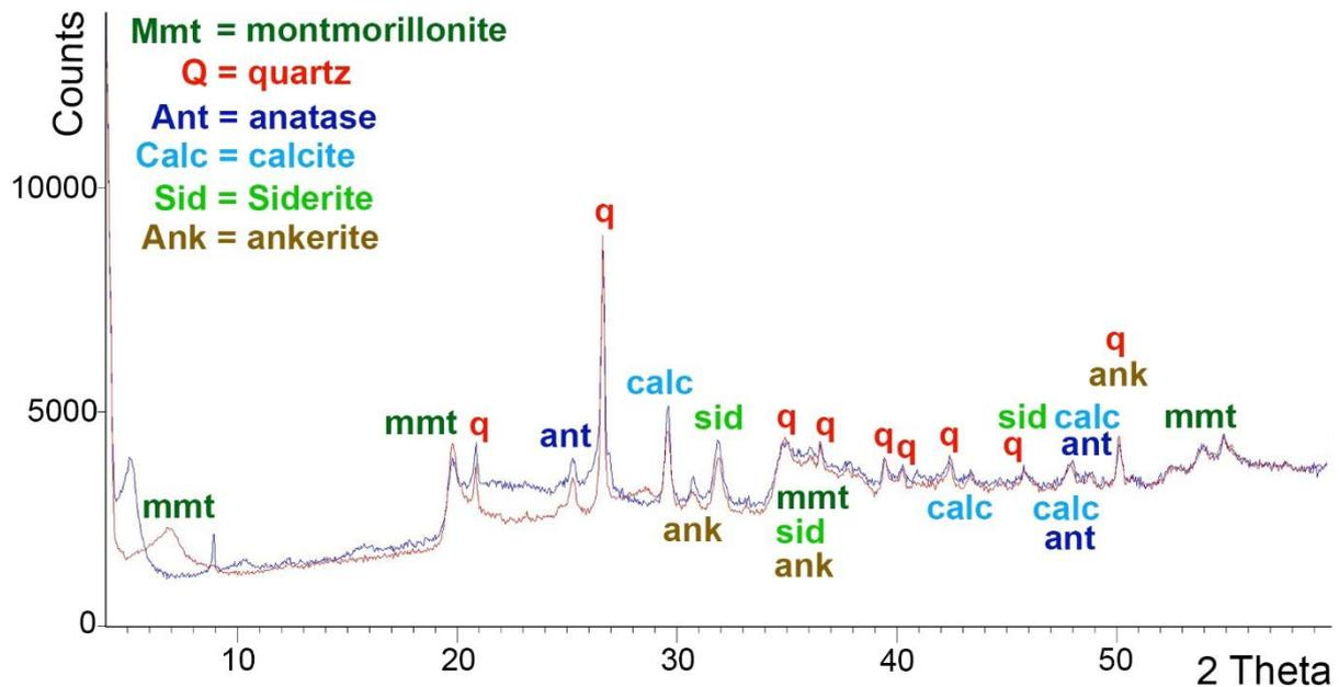
Figure 5 - X-ray diffraction pattern for B75\_2013. The red spectrum shows the pattern for untreated B75\_2013 and the blue spectrum shows the pattern following glycolation
