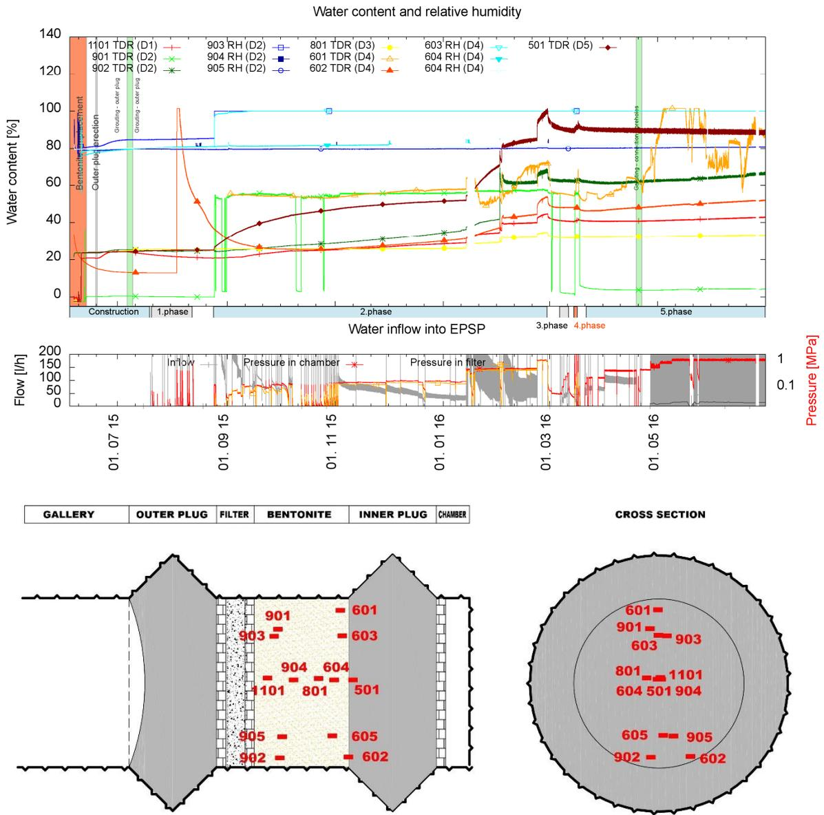
Figure 60 - Water content evolution in the bentonite sealing
