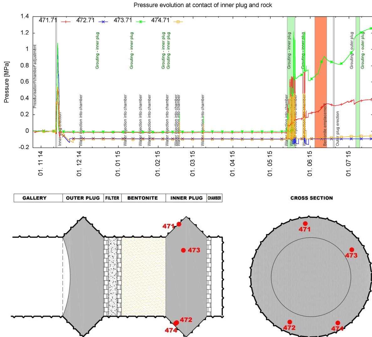
Figure 52 - Pressure evolution at on the contact between the inner plug and the rock mass
