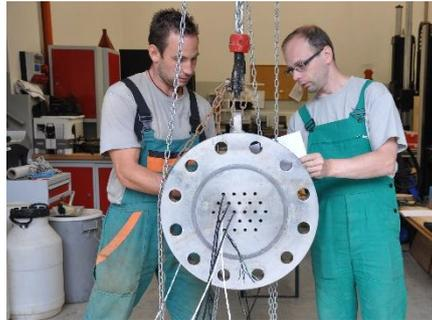
**Figure 16 - Cable head preparation**
