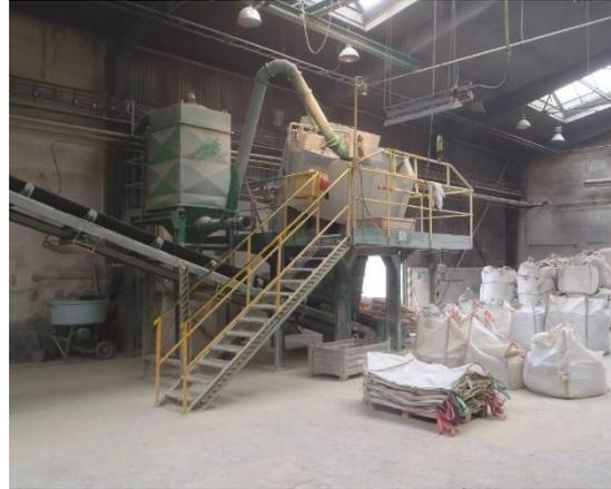
**Figure 30 - Mixing machine for adjusting water content in the dry bentonite**
