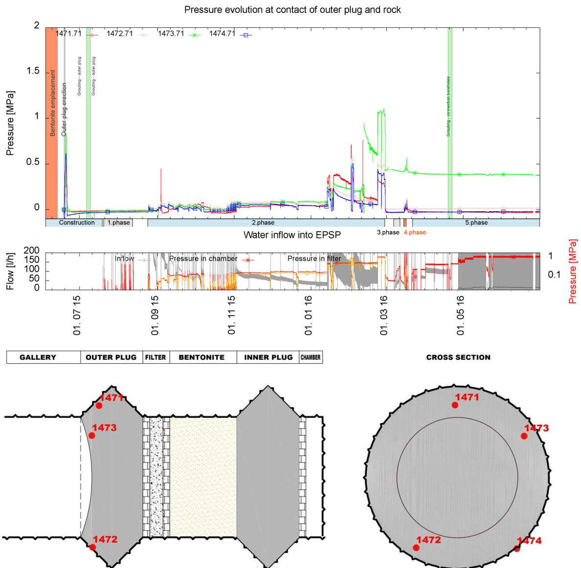
Figure 62 - Contact stress evolution between the plug and the rock mass (outer plug)
