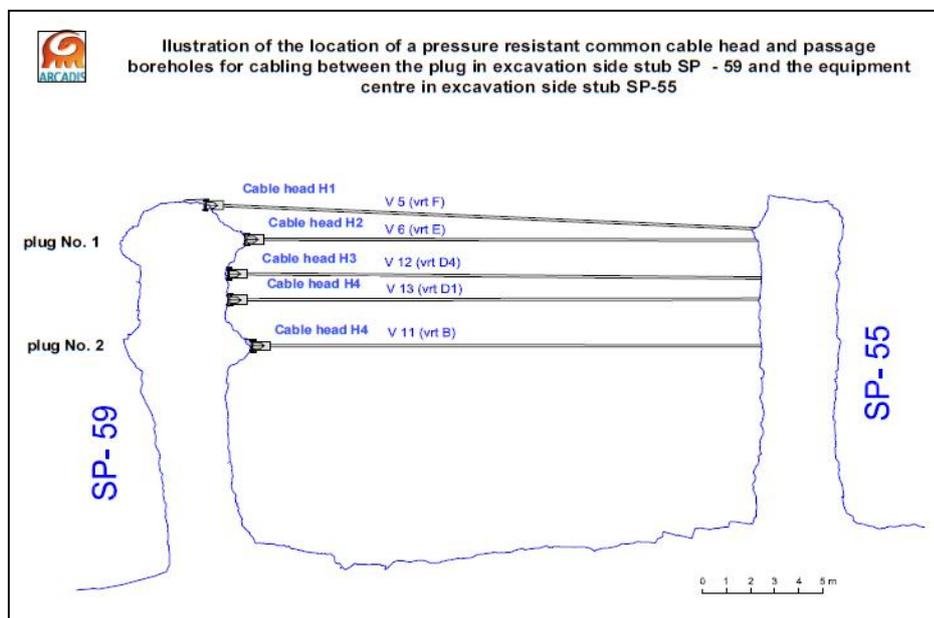
Figure 23 – Boreholes for the cabling connecting the experimental and technology niches
