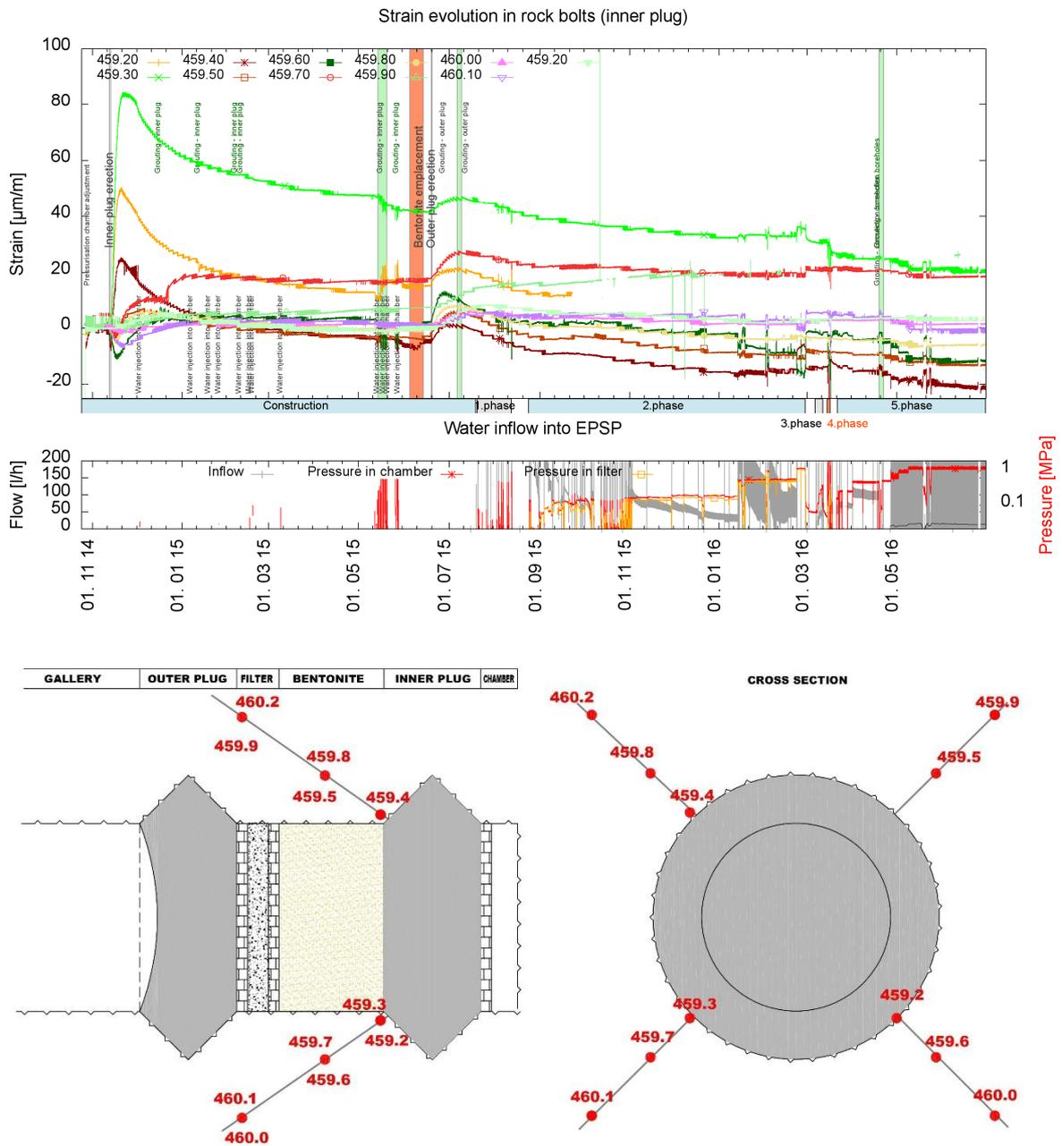
Figure 64 - Deformation of the rock
