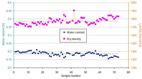
**Figure 29 - Results of sampling during the production process**
