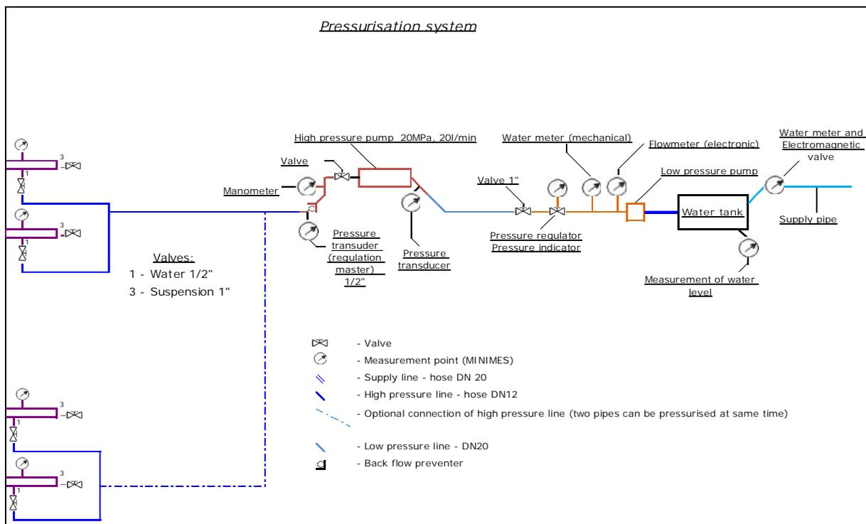
**Figure 19 - Pressurisation system (technology)**
