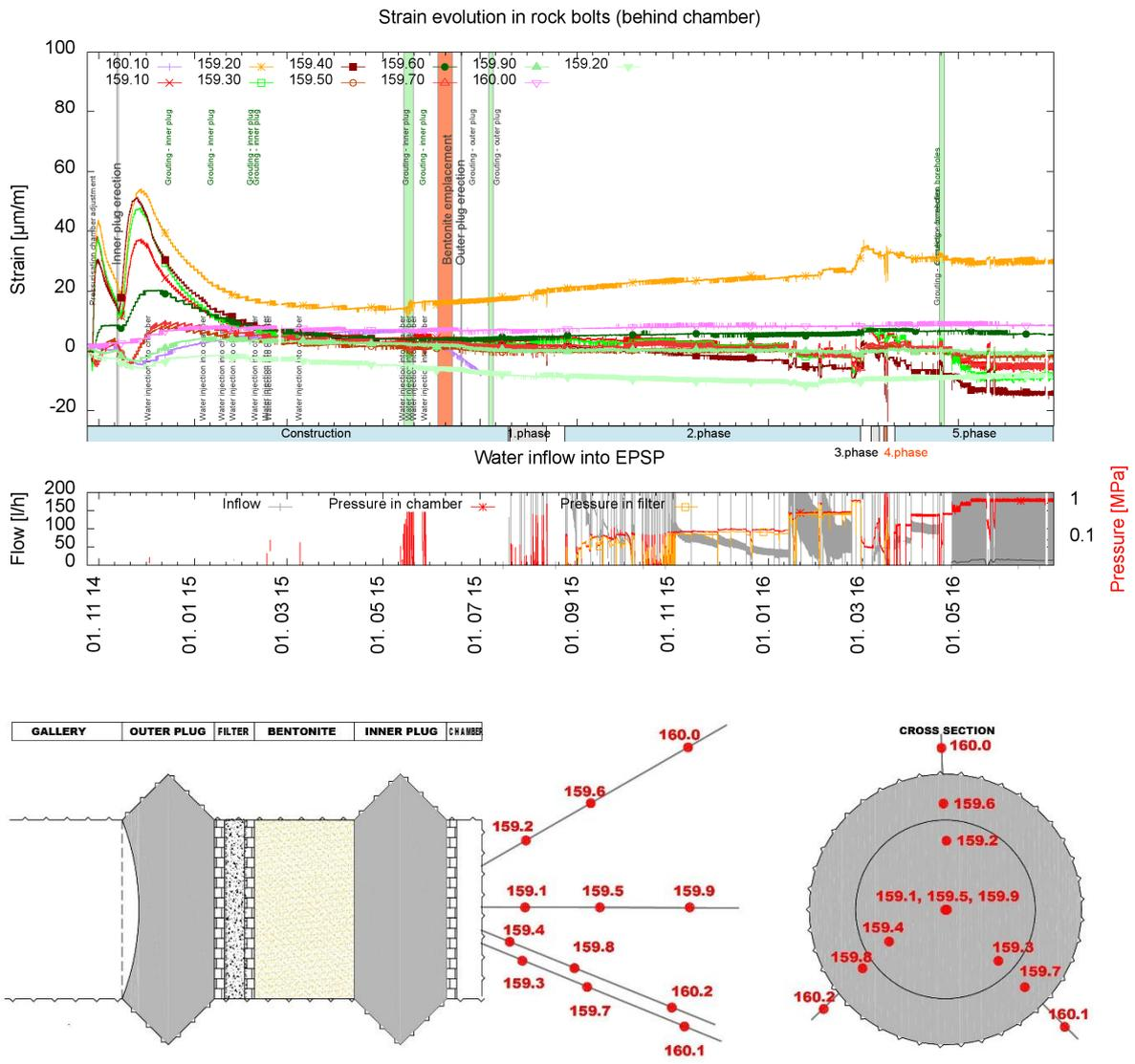
Figure 63 - Deformation of the rock
