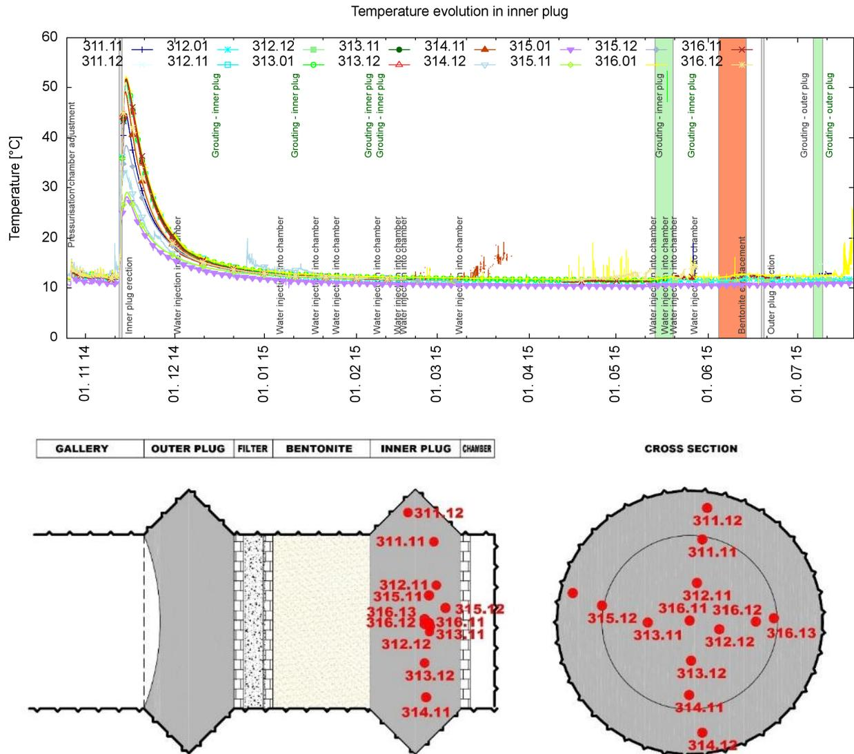
Figure 48 – Temperature in the inner shotcrete plug
