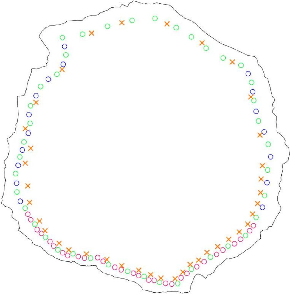
**Figure 25 – Drilling pattern for injection work on the inner plug**
