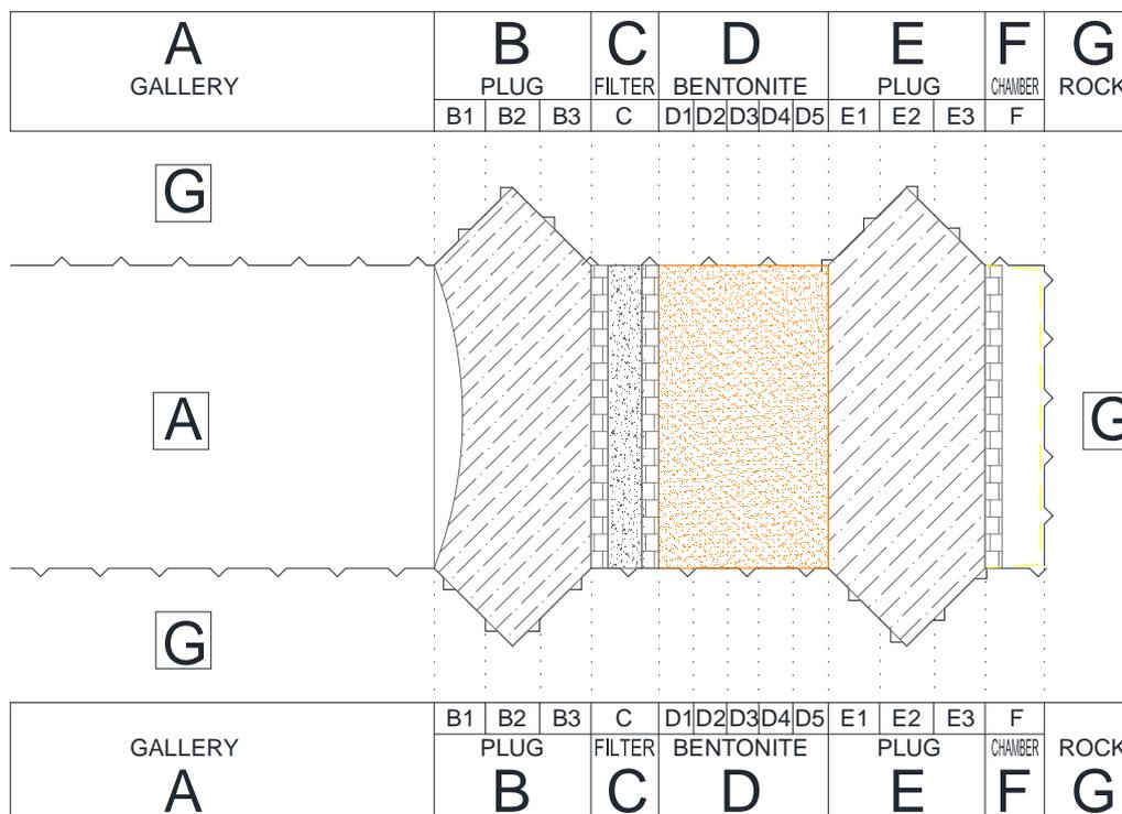
Figure 17 - profiles (A – gallery, B – outer concrete plug, C – filter, D – bentonite, E – inner glass fibre shotcrete plug, F – pressure chamber, G – rock, H – technology)
