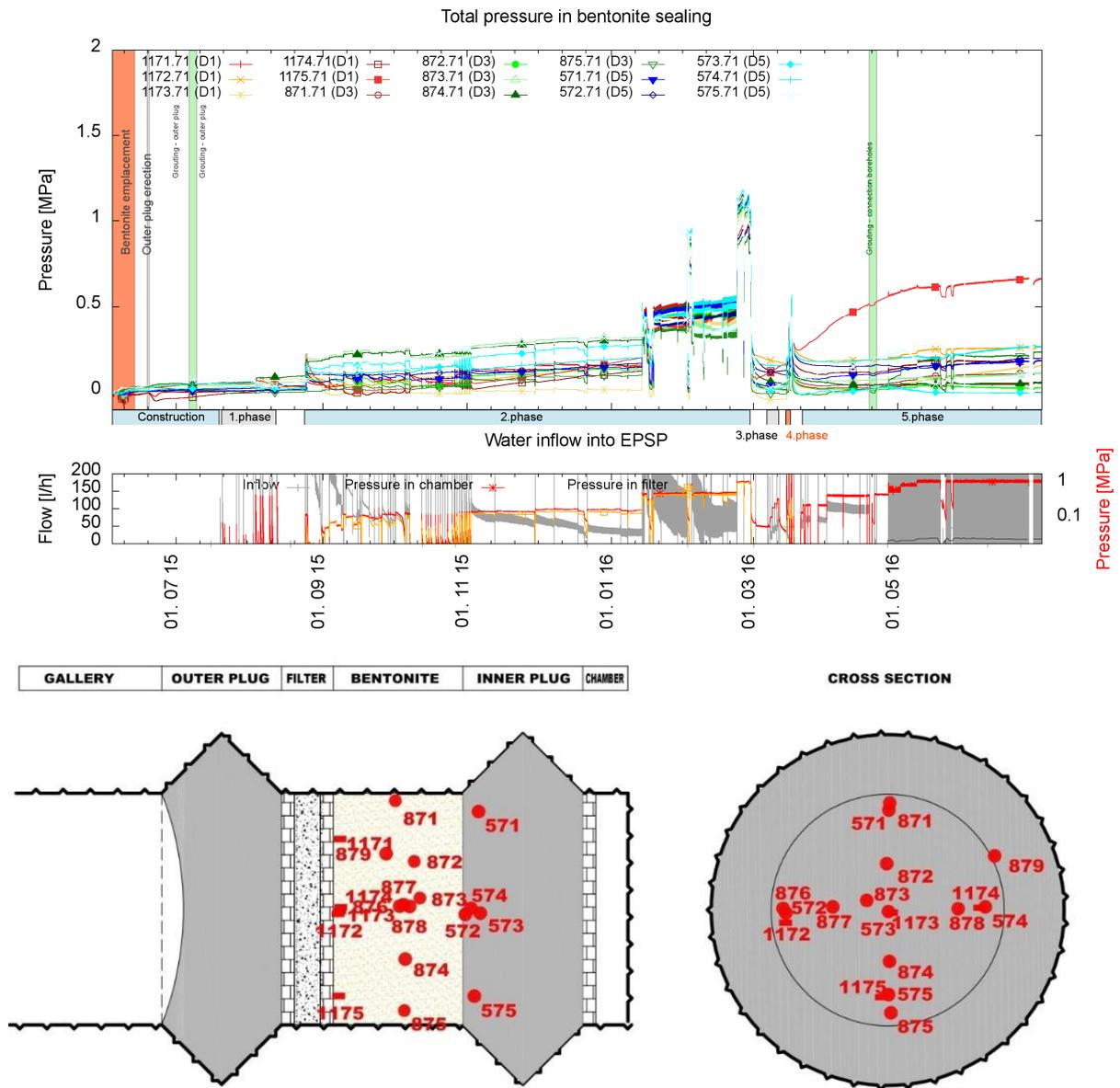
Figure 58 - Total pressure evolution in the bentonite sealing
