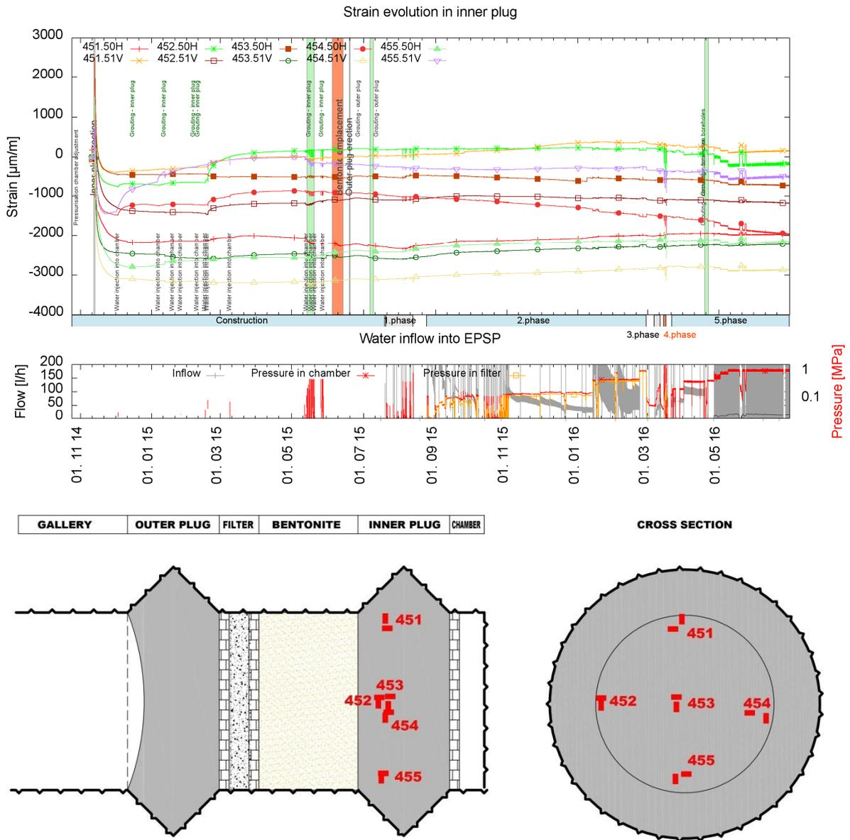
Figure 55 - Deformation of inner plug
