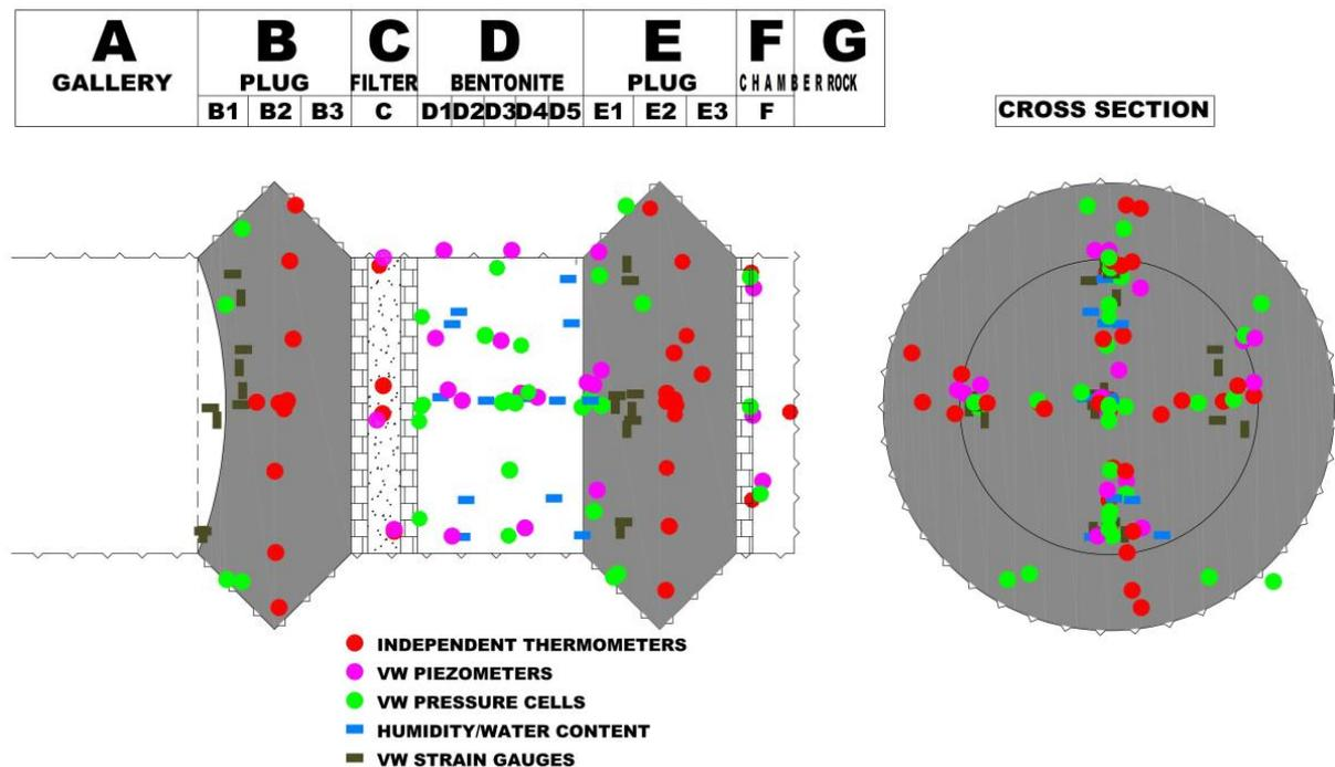
Figure 42 – Sensors installed in the EPSP
