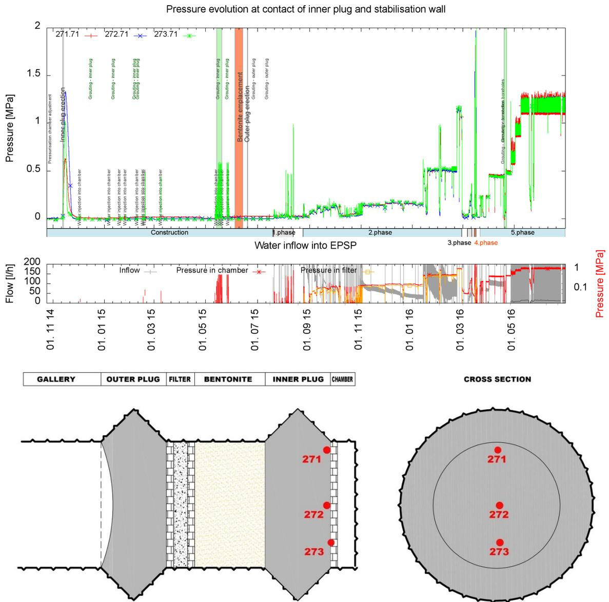
Figure 57 - Contact stress at the contact of inner plug and the stabilisation wall
