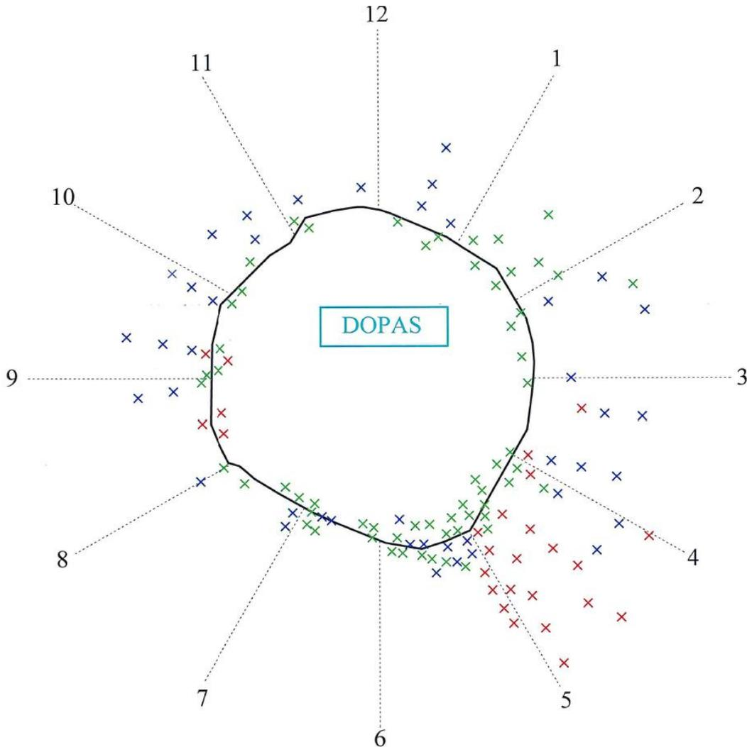
**Figure 26 – Drilling pattern for injection work on the outer plug**
