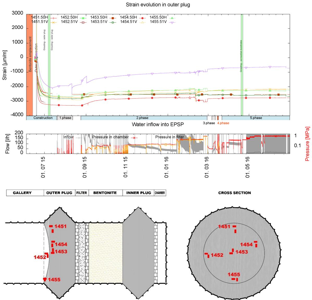
Figure 61 - Deformation of the outer plug
