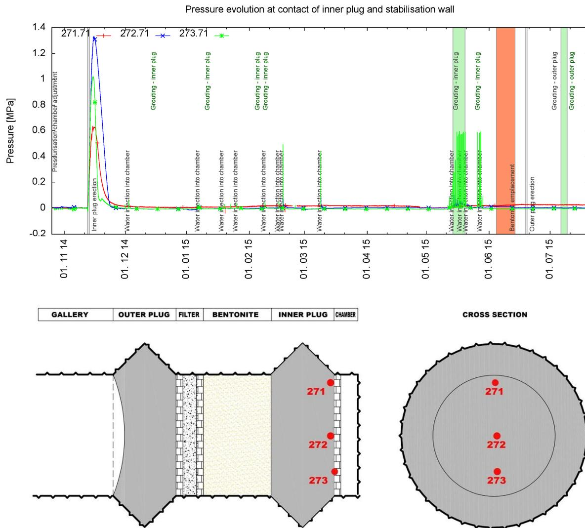
Figure 54 - Contact stress evolution at the contact between the inner plug and the stabilisation wall
