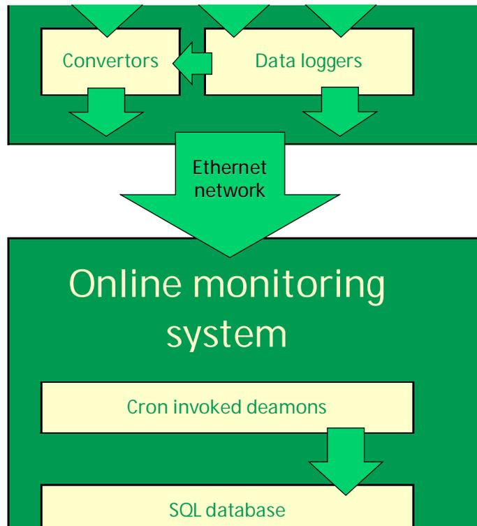
**Figure 12 - EPSP measurement system**
