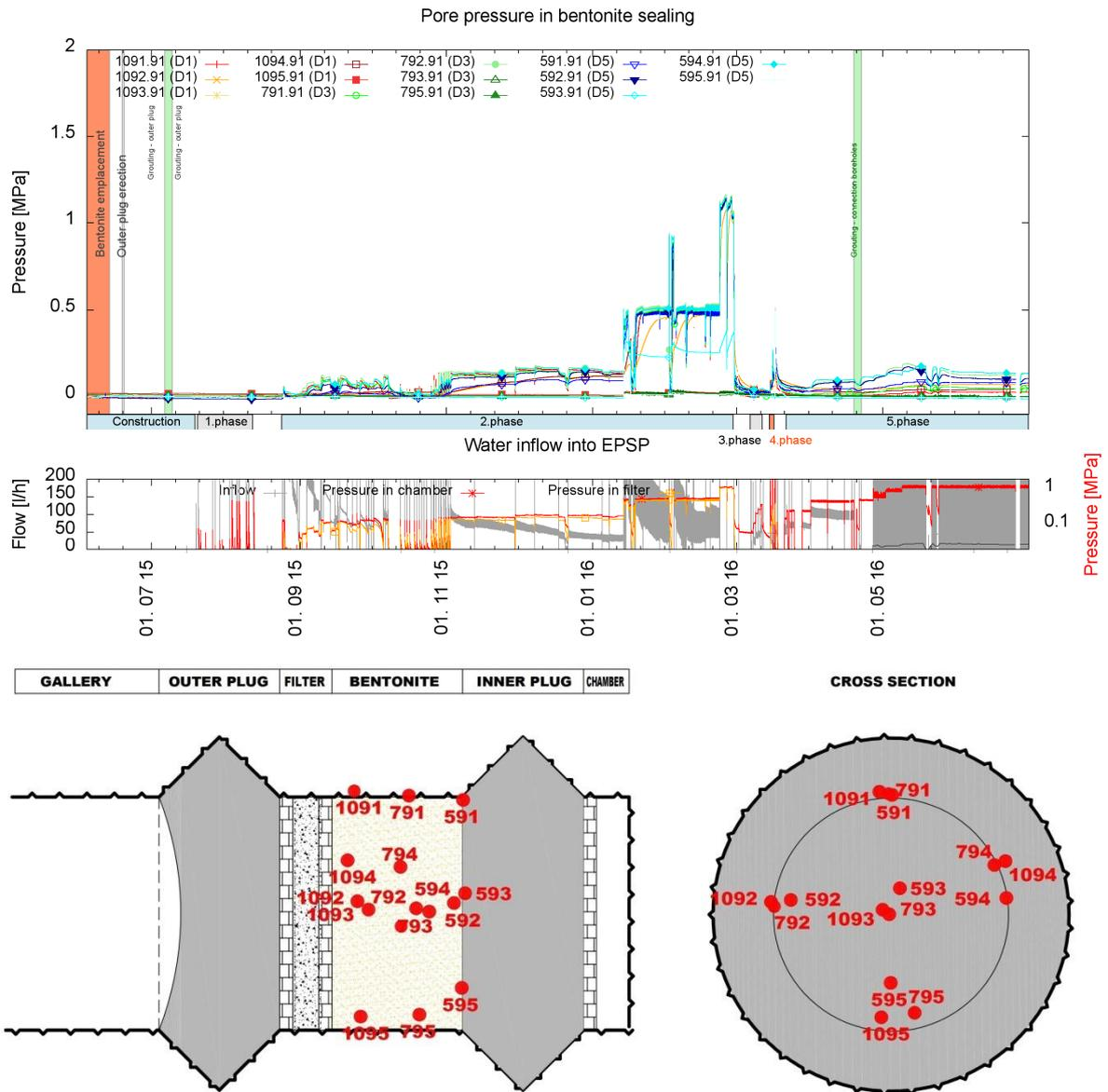
Figure 59 - Pore pressure evolution in the bentonite sealing
