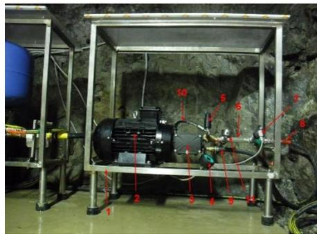
**Figure 21 - High pressure unit**
