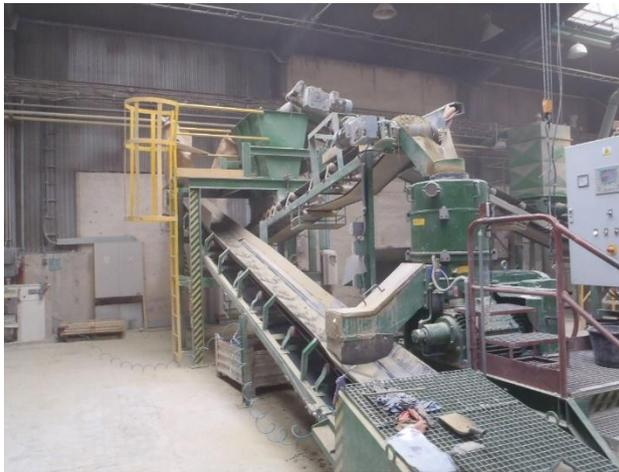
**Figure 31 - Roller compaction machine**
