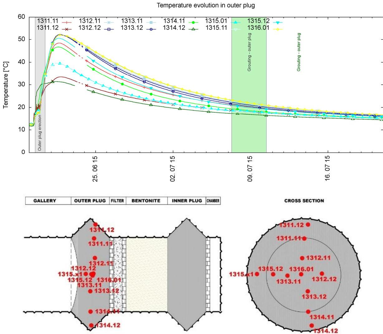
Figure 49 – Temperature in the outer shotcrete plug
