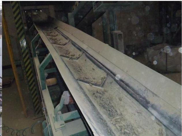
**Figure 32 - Transport of the pellets from the roller compaction machine**
