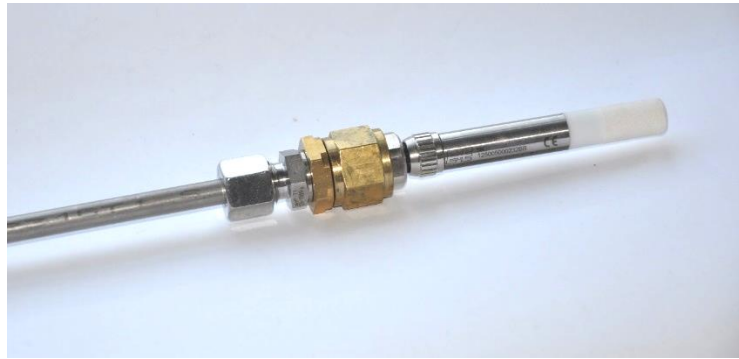
Figure 5 - RH sensor including cabling protection
