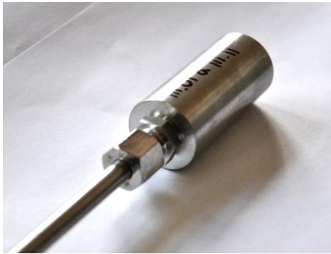
Figure 4 - temperature sensor in a protective housing
