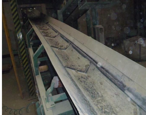
Figure 35 - Transport of the pellets from the roller compaction machine
