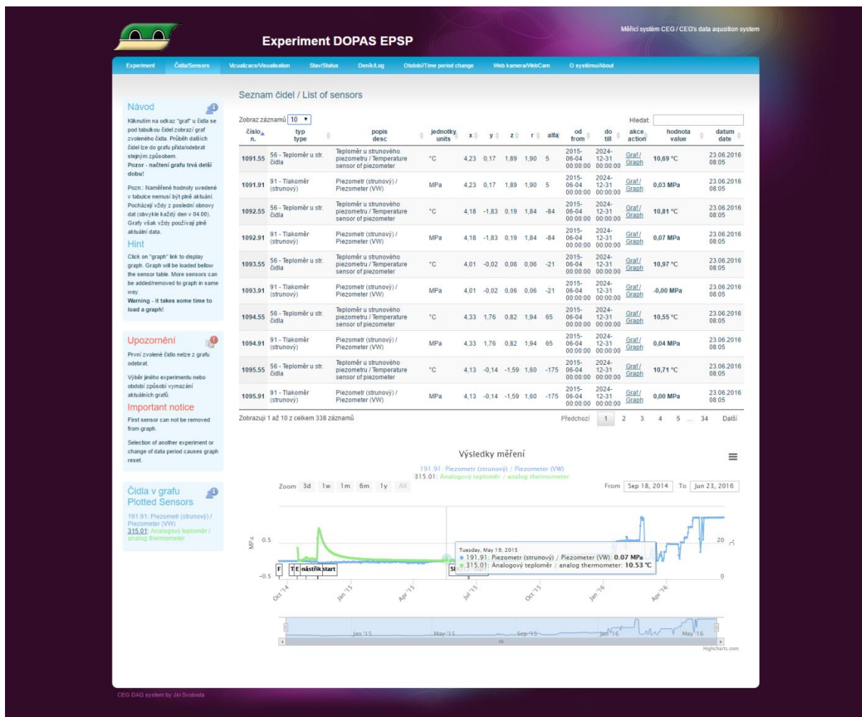
Figure 75 - EPSP measurement system web frontend UI
