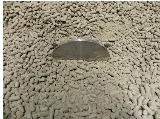
Figure 48 - Pressure cell (8 June 2015)
