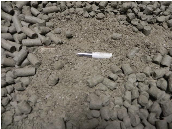
Figure 47 - RH sensor installation (7 June 2015)
