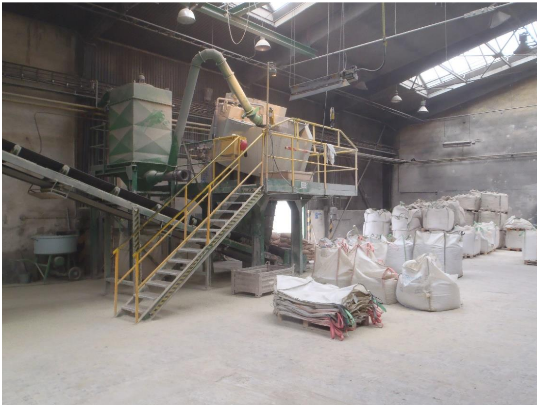
Figure 33 - Mixing machine for adjusting water content in the dry bentonite (from w=8\% to approx. 19\% )
