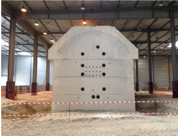
(a) Coring of the wire sawn low-pH SCC containment wall
