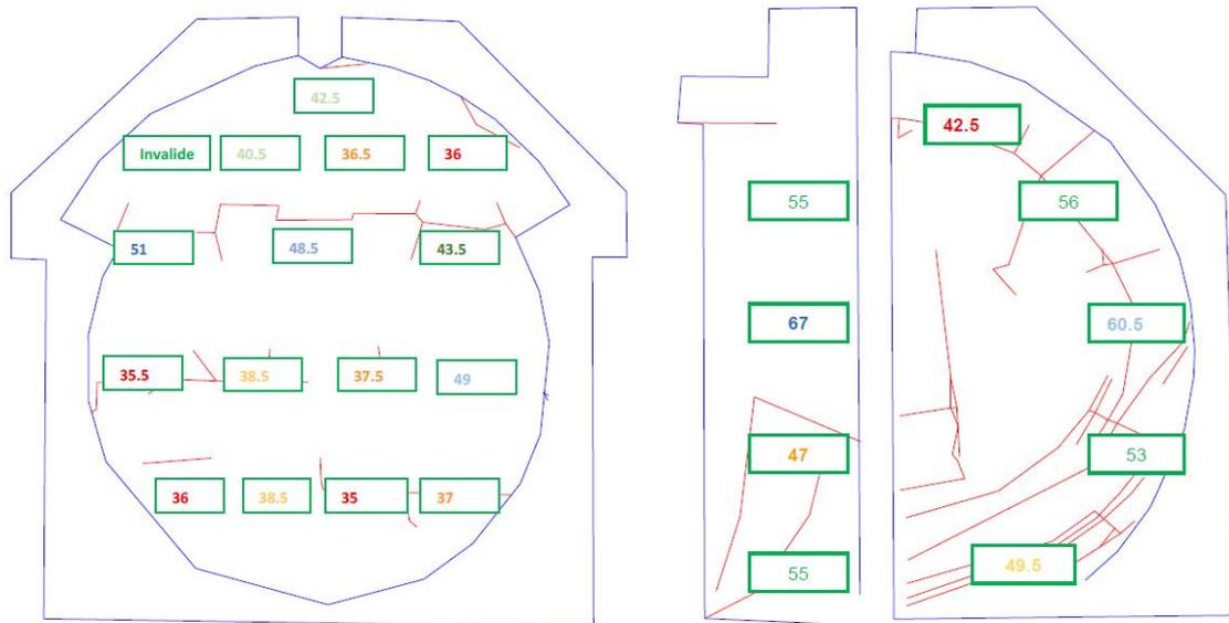
**Figure 2.13:** Results for hardness tests on the concrete (left) and shotcrete (right) containment walls (numbers indicate values in MPa).
