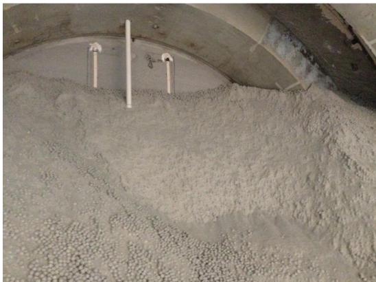
(e) Removal of the bentonite clay core
