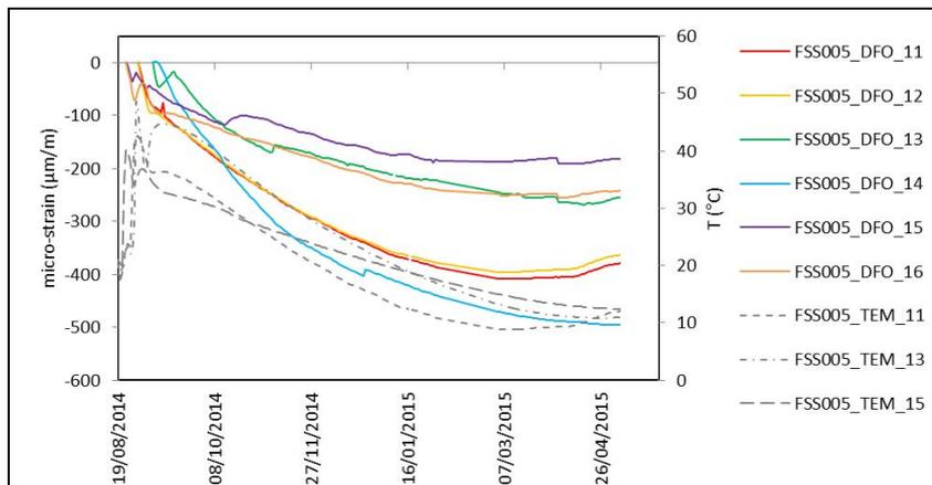
**Figure 2.6:** Temperature and strain measured for the low-pH shotcrete containment wall at the Section 5 location.
