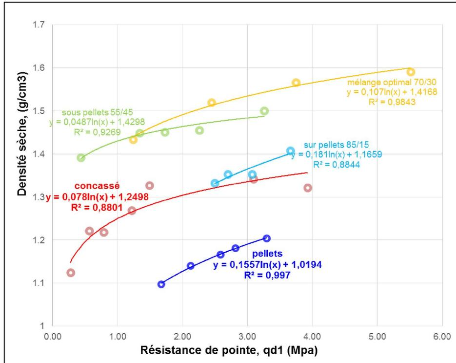
**Figure 2.11:** Calibration curves for the five bentonite mixes tested. “Densité sèche” means “dry density”, “mélange” means “mix”, “concassé” means “crushed”, and “Résistance de pointe” means “resistance of the tip” of the penetrometer.
