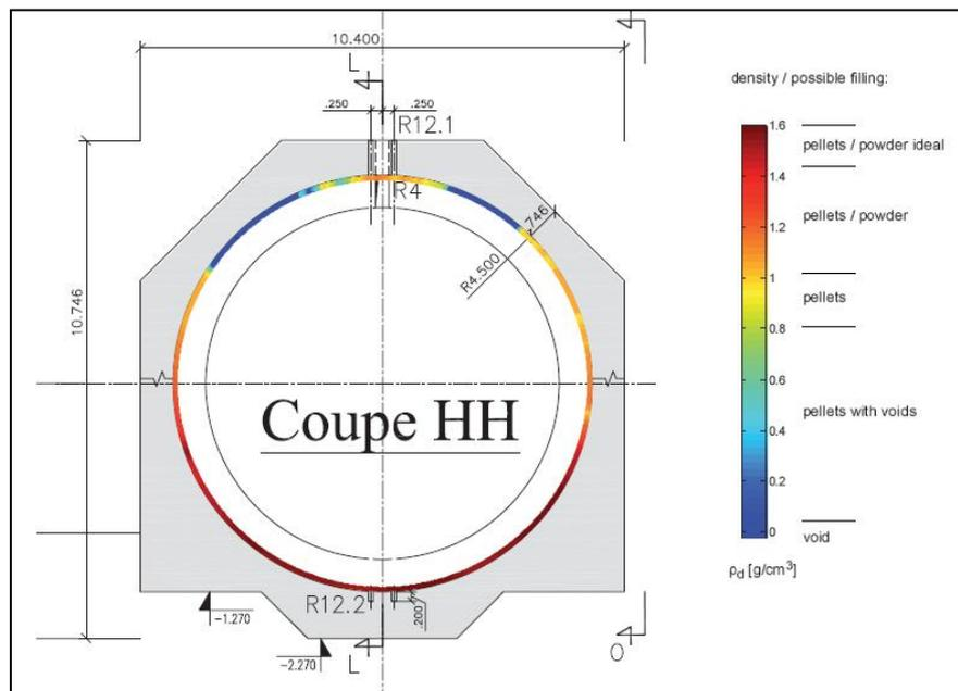
**Figure 2.10:** Illustration of TDR sensors measure of dry mix density at the HH section.
