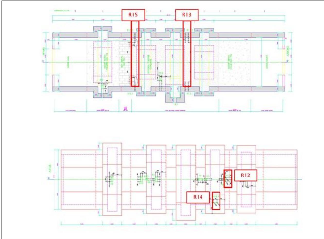
**Figure 2.4:** Location (in red) of the different pipes pre-positioned in FSS for gamma-gamma logging of the swelling clay core.
