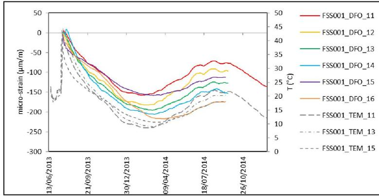
**Figure 2.5:** Temperature and strain measured for the low-pH SCC containment wall at the Section 1 location.
