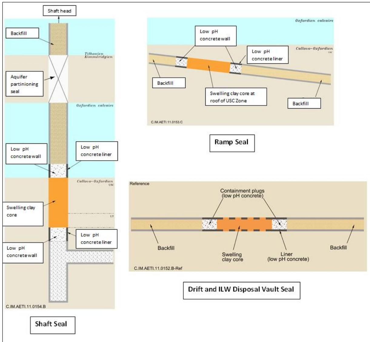
**Figure 2.1:** Schematic illustration of the conceptual designs for shaft, ramp, and drift and ILW disposal vault seals for the Cigéo reference disposal concept (Andra).
