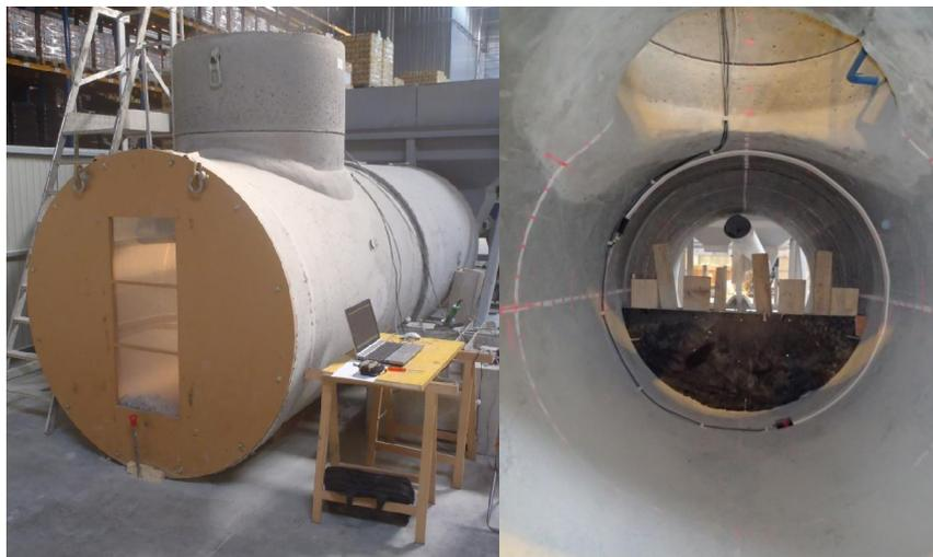
**Figure 2.9:** TDR sensor calibration inside the metric emplacement test pipe.
