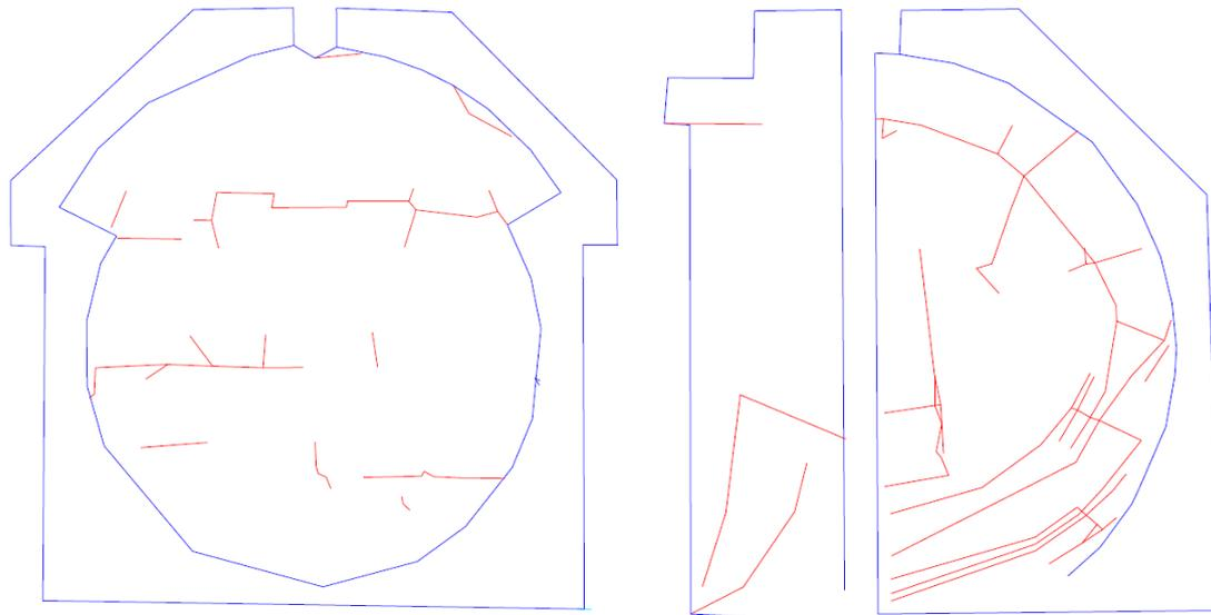
**Figure 2.12:** The pattern of cracks in the low-pH SCC (left) and shotcrete (right) containment walls.
