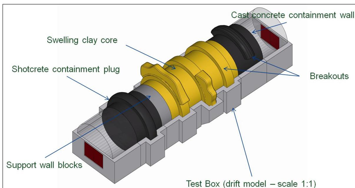
**Figure 2.2:** Schematic illustration of the FSS experiment design.
