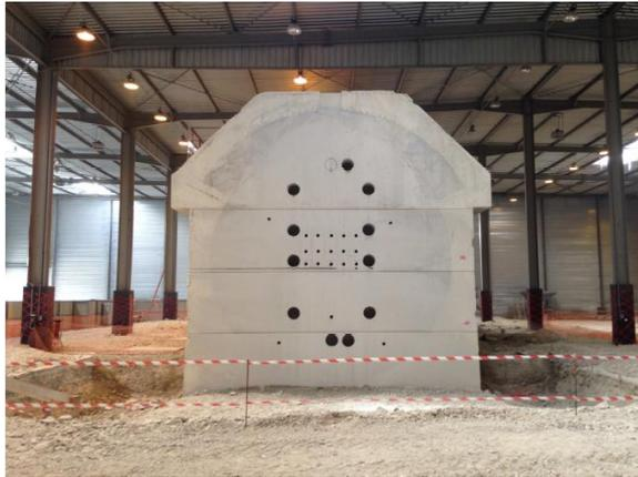
(a) Coring of the wire sawn low-pH SCC concrete containment wall
