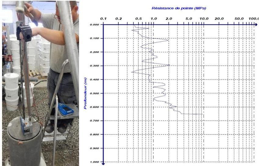
**Figure 2.12:** Calibration test on FSS 70/30 mix (left) and related penetrogram (right)
