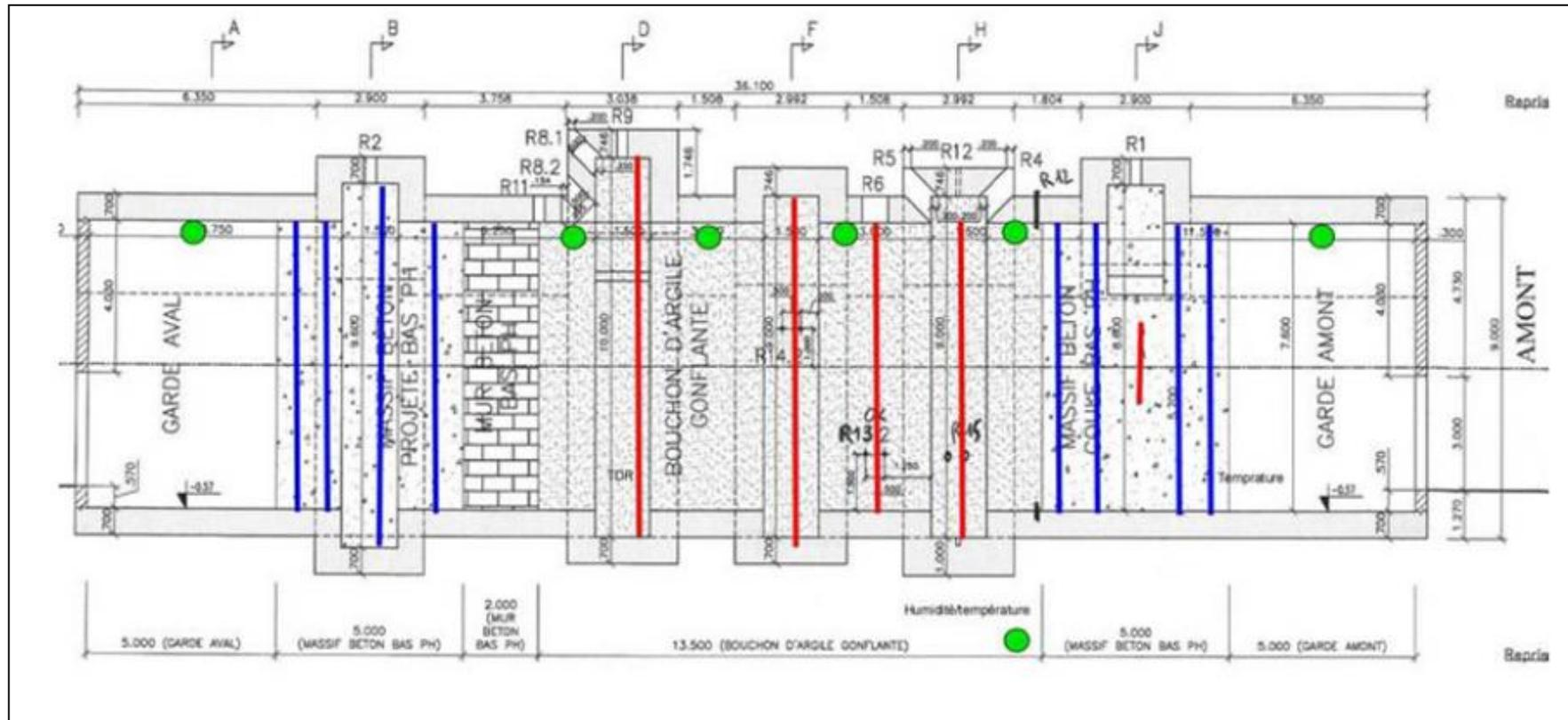
**Figure 2.3:** Location of the different sensors in FSS (blue: strain and temperature sensors in the low-pH concrete containment walls; green: relative humidity and temperature sensors; red: TDR sensors located in the swelling clay core).
