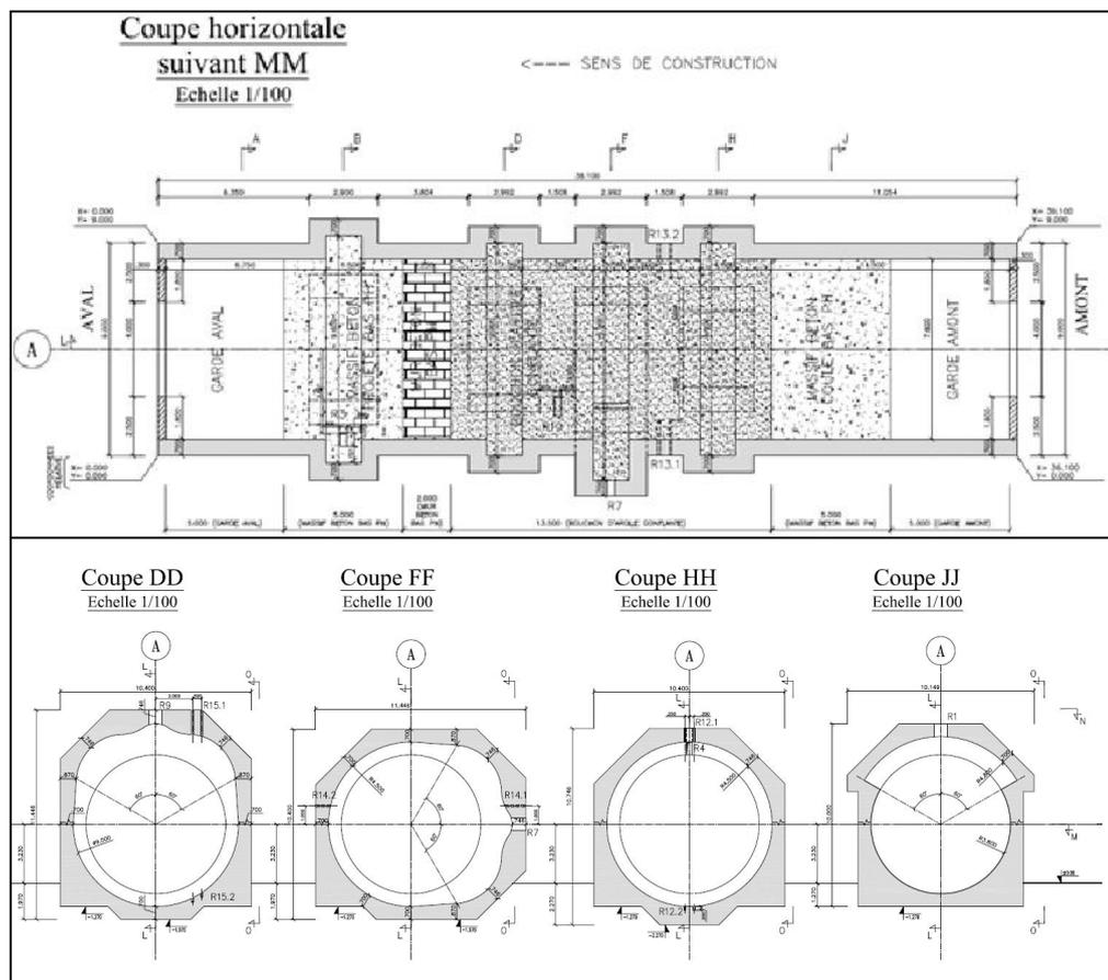
**Figure 2.7:** Longitudinal (top) and sectional (bottom) positioning of the TDR sensors.
