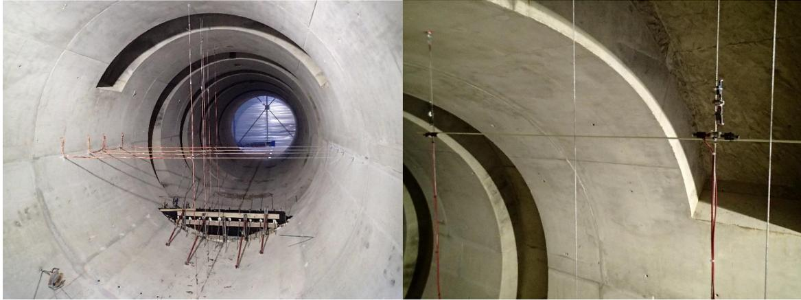
**Figure 2.5:** Photos of temperature sensors and strain gauges as installed in the test box
