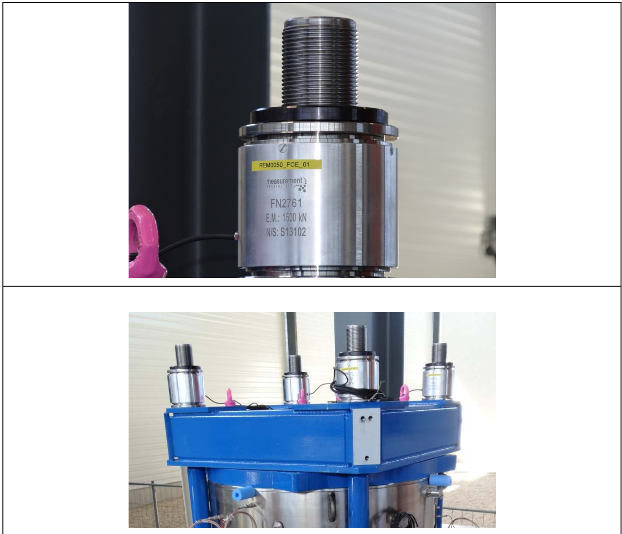
Figure 4-16 Installation of force washers
