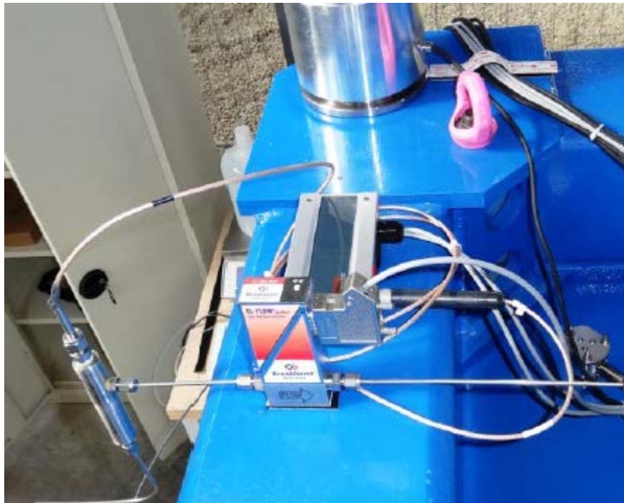
Figure 4-18 Humidity and temperature sensor (REM0060_HUM/TEM_01) and flowmeter (REM0080_DAI_01) in-line on the outlet circuit
