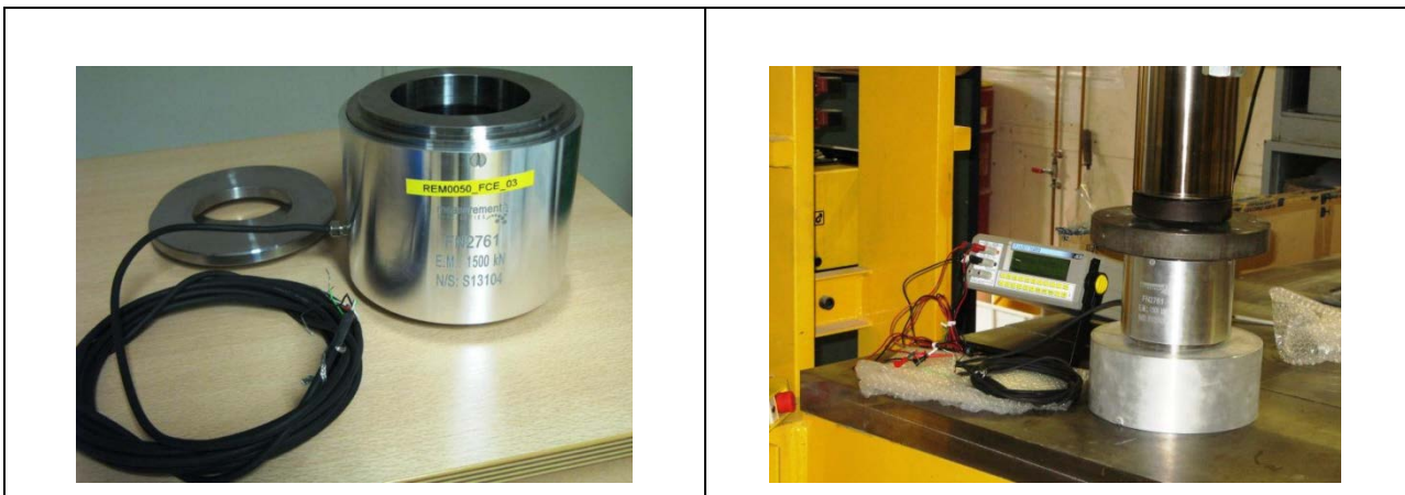
Figure 3-8 Force washer (left) with its support washers and under the press during calibration (right)
