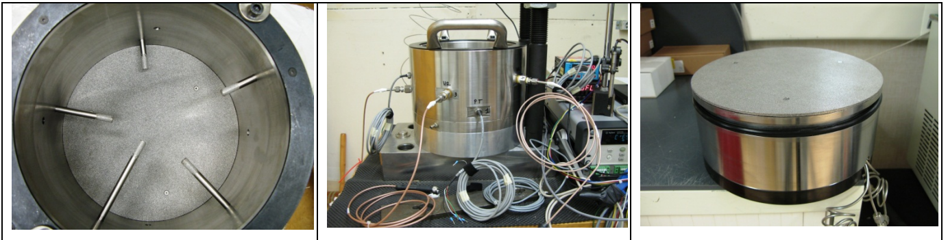
Figure 6-10 Confinement cylinder set-up, radial sensor installation
