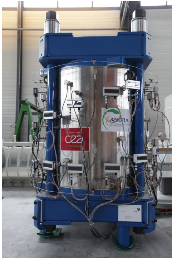
Figure 4-22 REM cell following complete installation
