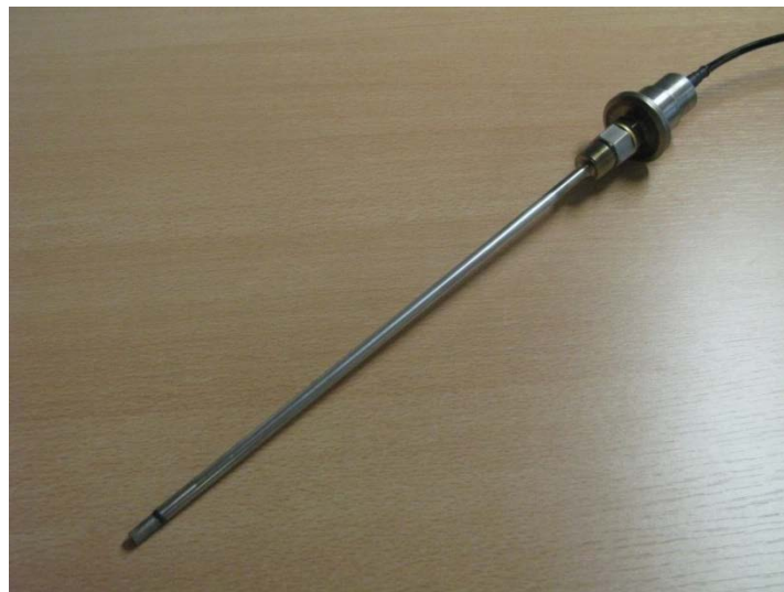
Figure 3-12 Pore pressure sensor fitted onto its extension tube
