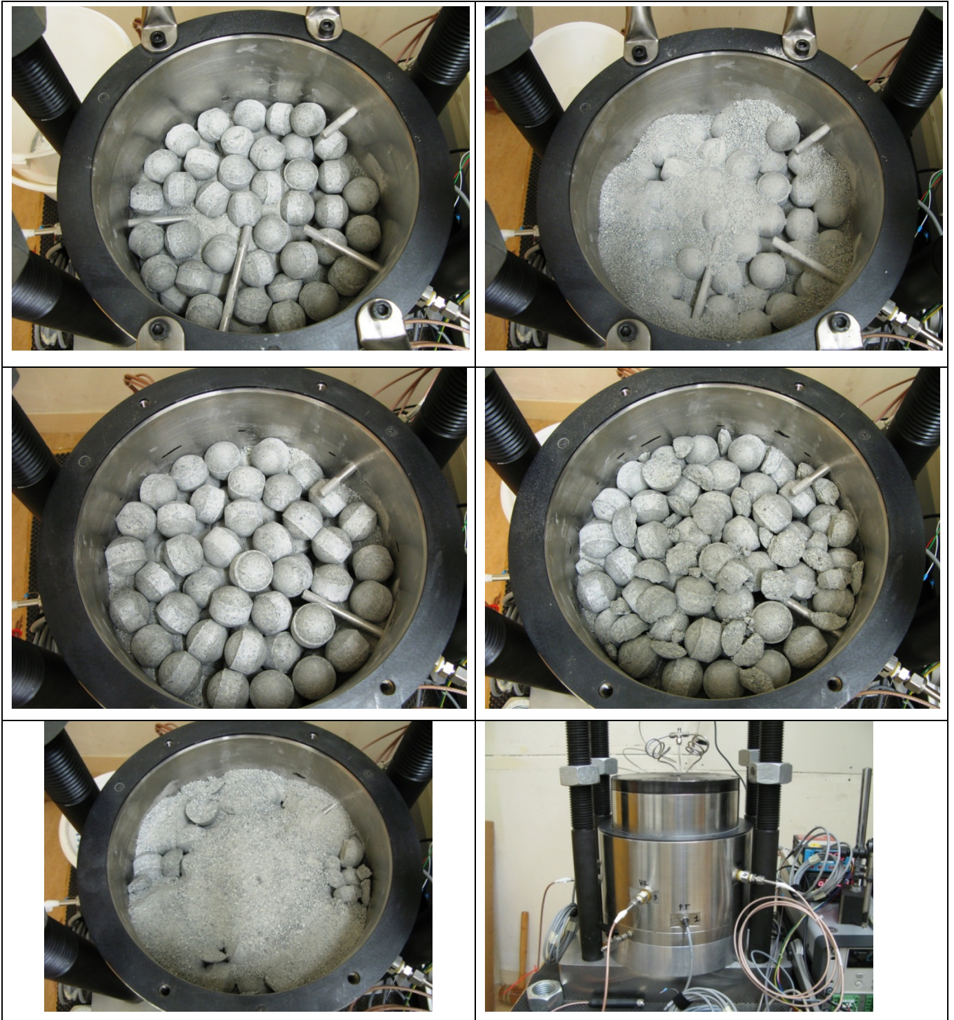
Figure 6-11 Emplacement of MM1 sample in the 240 mm cell
