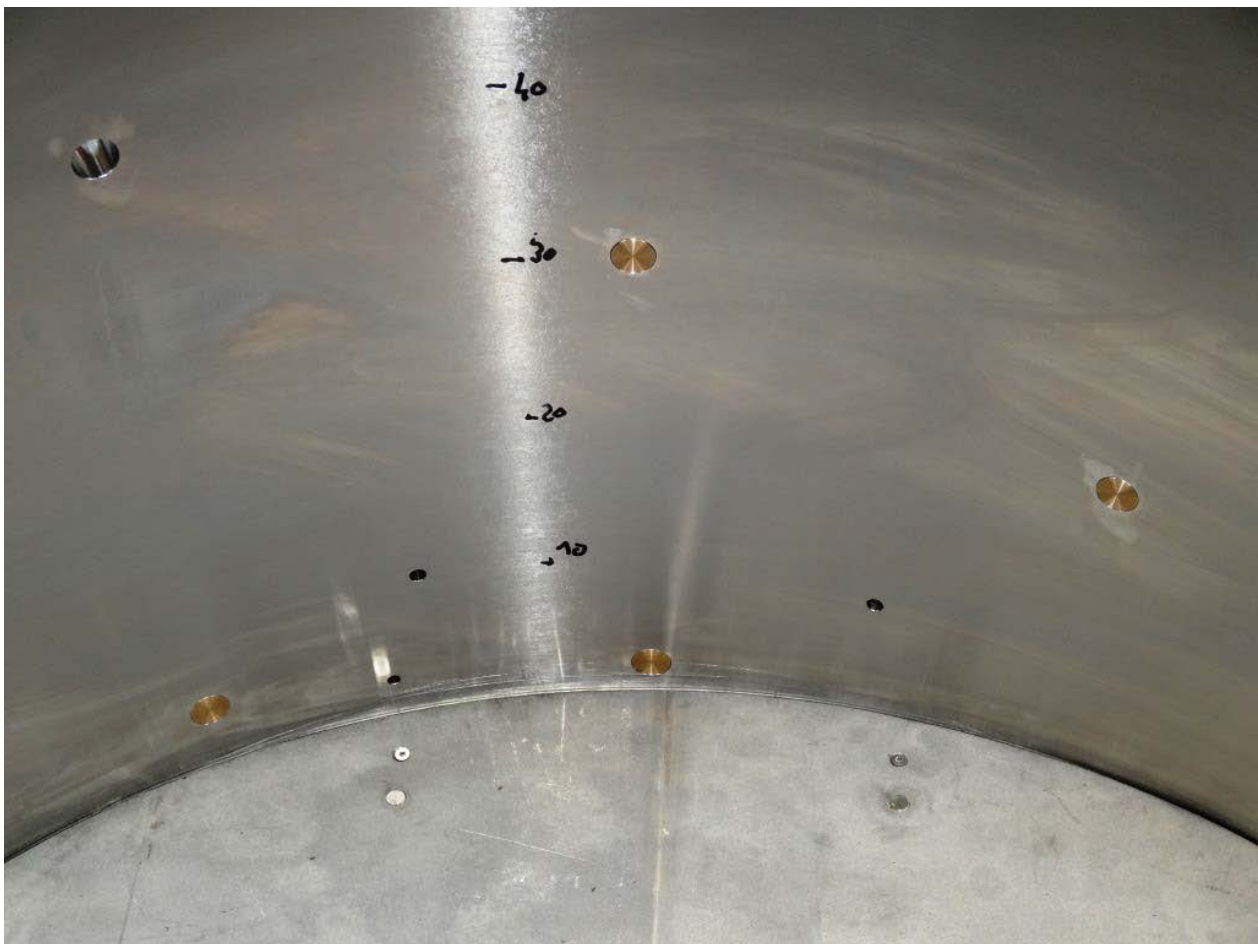
Figure 4-7 Ends of the radial load cell pistons
