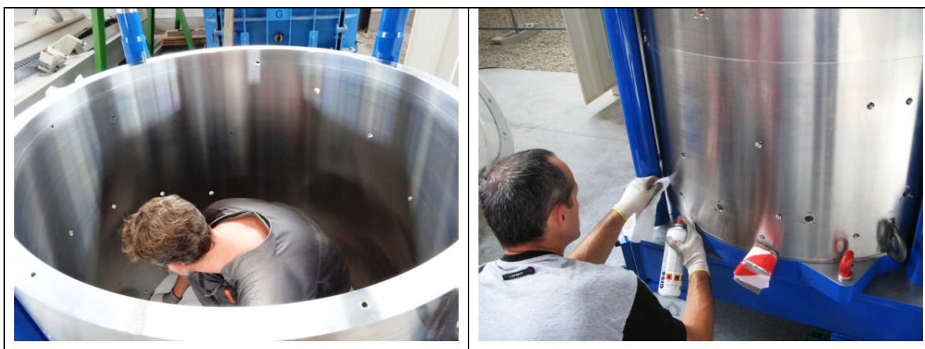
Figure 4-4 Careful cleaning of the vessel by CEA before sensor installation
