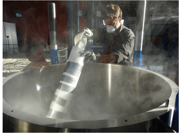
(b) crushed bentonite being poured
