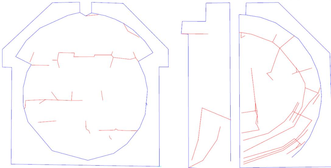
**Figure 4.14:** The pattern of cracks in the low-pH SCC (left) and shotcrete (right) containment walls.
