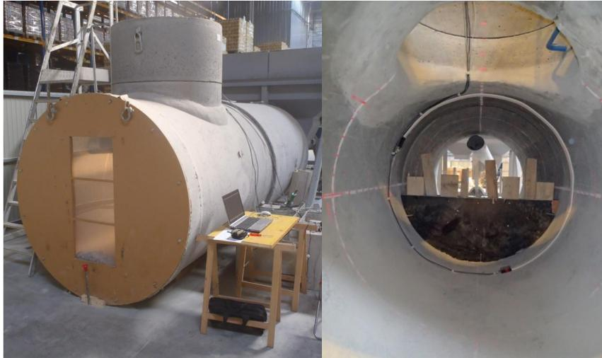
**Figure 4.9:** TDR sensor calibration inside the metric emplacement test pipe.
