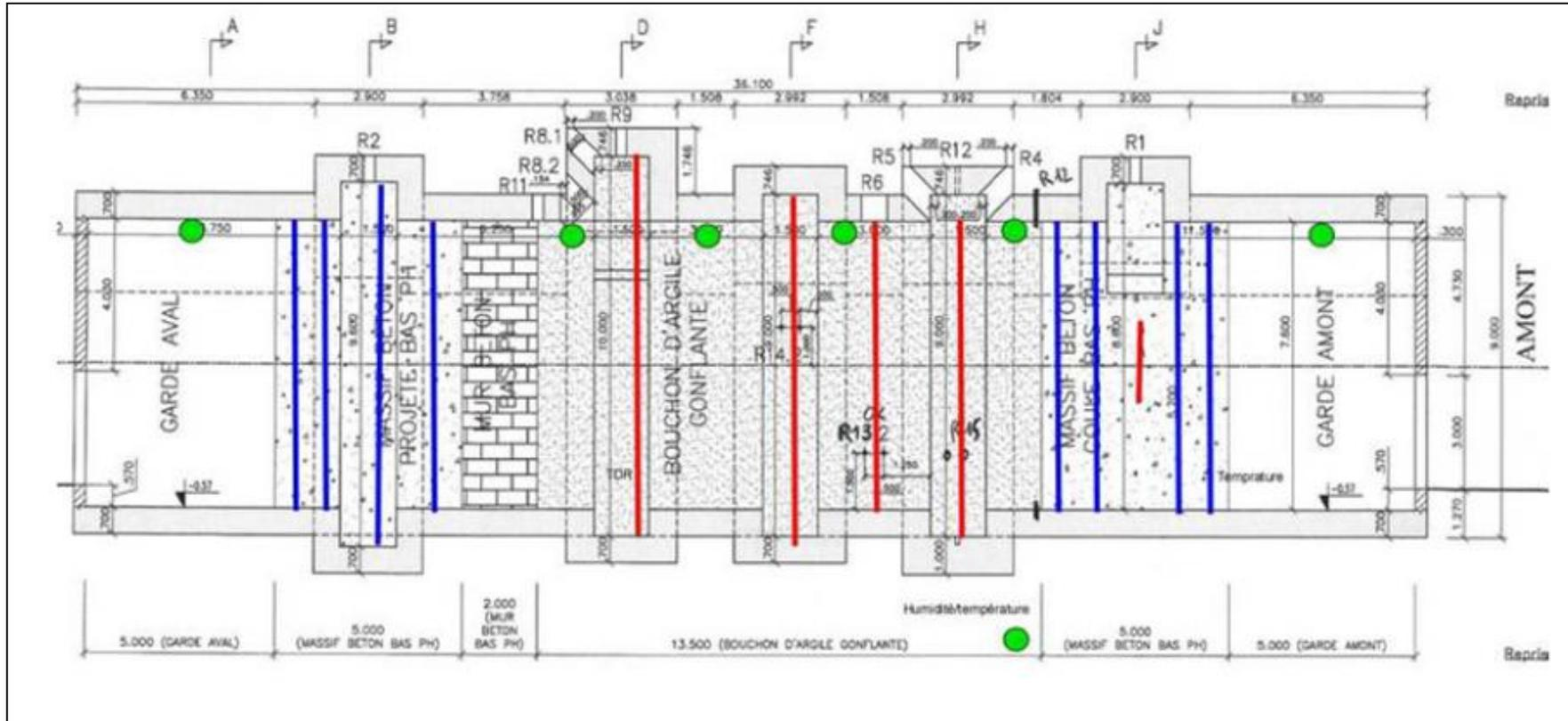
**Figure 4.3:** Location of the different sensors in FSS (blue: strain and temperature sensors in the low-pH concrete containment walls; green: relative humidity and temperature sensors; red: TDR sensors located in the swelling clay core).
