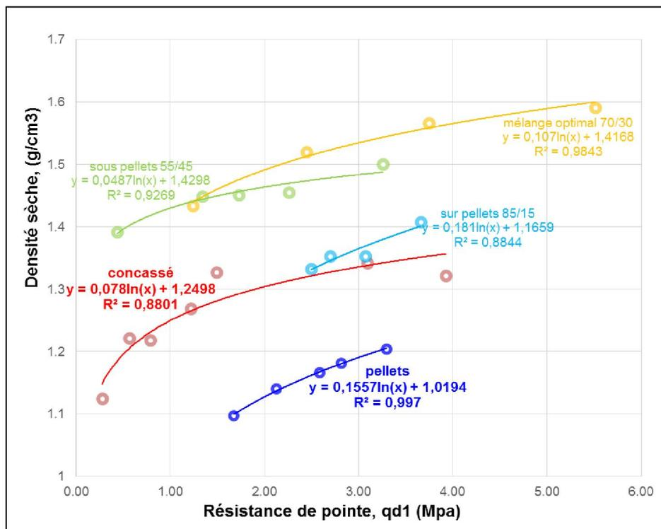
**Figure 4.11:** Calibration curves for the five bentonite mixes tested. “Densité sèche” means “dry density”, “mélange” means “mix”, “concassé” means “crushed”, and “Résistance de pointe” means “resistance of the tip” of the penetrometer.
