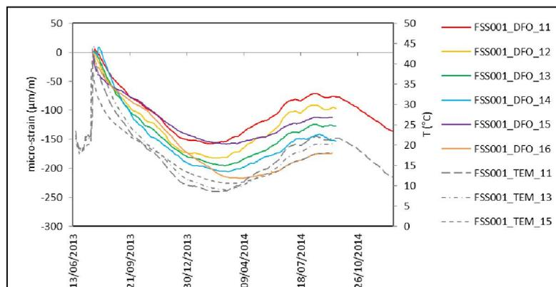
**Figure 4.5:** Temperature and strain measured for the low-pH SCC containment wall at the Section 1 location.
