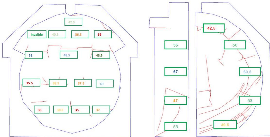
**Figure 4.15:** Results for hardness tests on the concrete (left) and shotcrete (right) containment walls (numbers indicate values in MPa).
