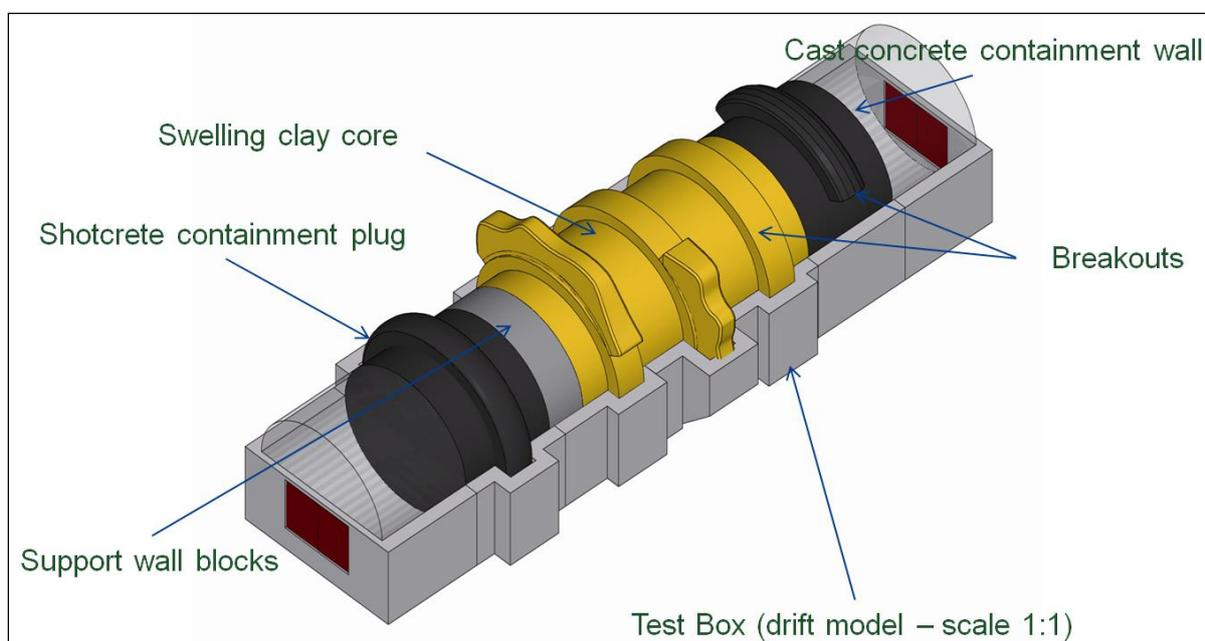
**Figure 4.2:** Schematic illustration of the FSS experiment design.
