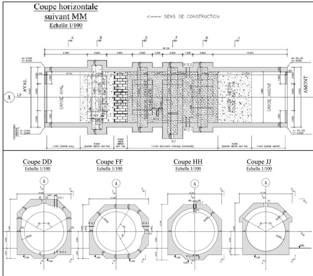
**Figure 4.7:** Longitudinal (top) and sectional (bottom) positioning of the TDR sensors.
