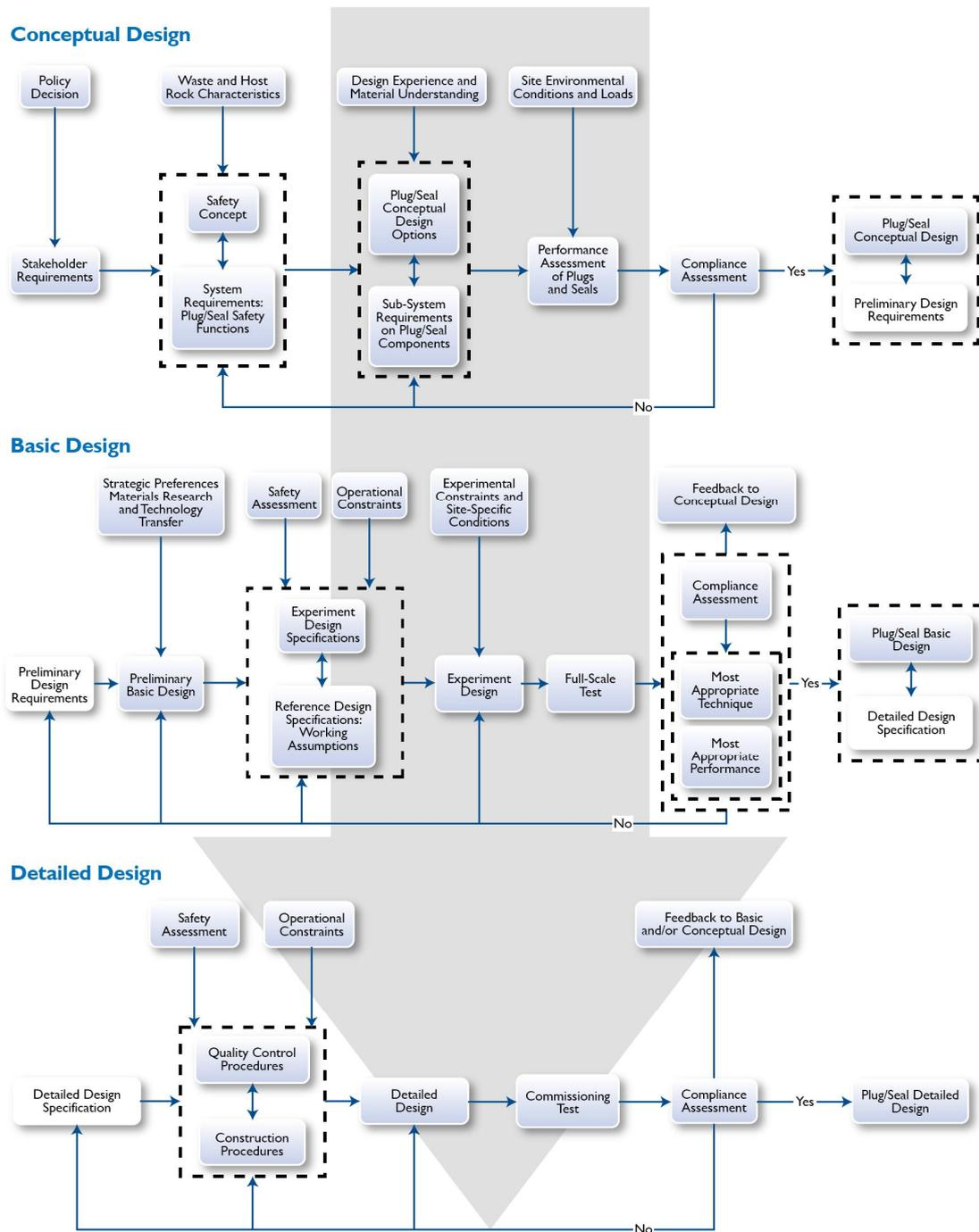
**Figure 3.1:** The DOPAS Design Basis Workflow. Dashed boxes are used to show activities undertaken in parallel.
