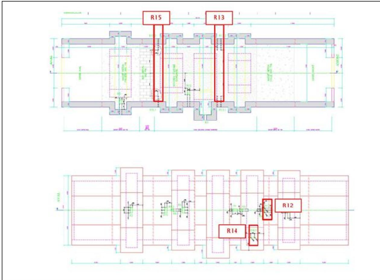
**Figure 4.4:** Location (in red) of the different pipes pre-positioned in FSS for gamma-gamma logging of the swelling clay core.
