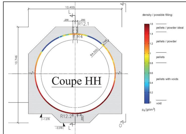
**Figure 4.10:** Illustration of TDR sensors measure of dry mix density at the HH section.
