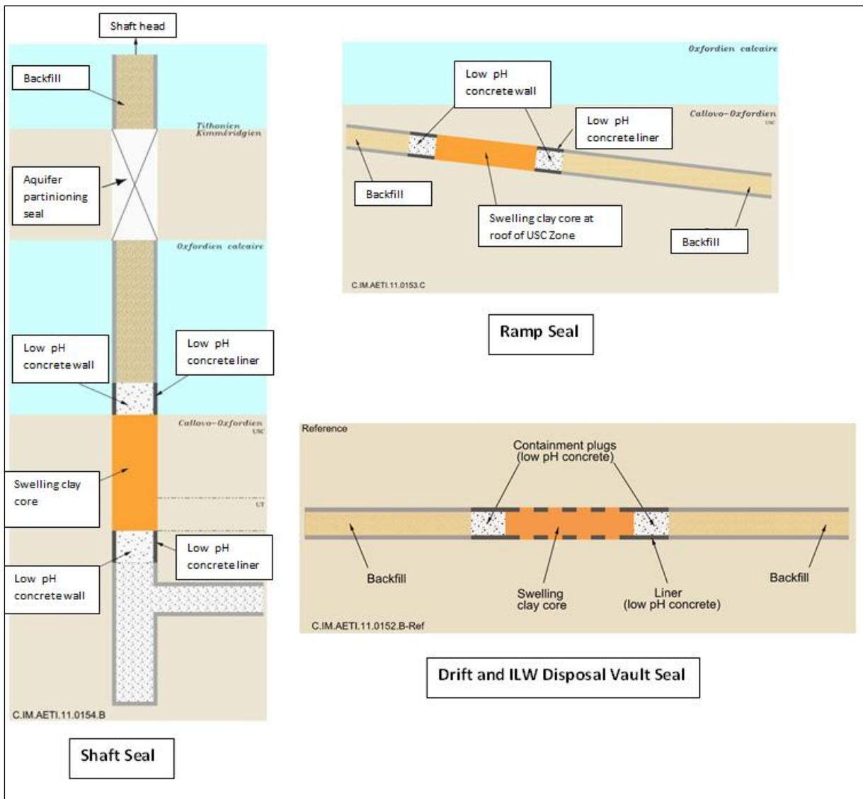
**Figure 4.1:** Schematic illustration of the conceptual designs for shaft, ramp, and drift and ILW disposal vault seals for the Cigéo reference disposal concept (Andra).
