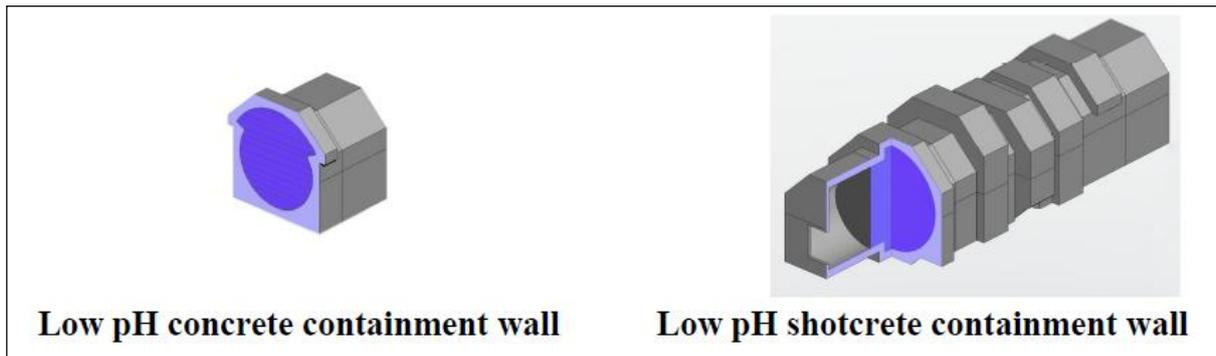
**Figure 4.13:** Sawing of the SCC containment wall (transversally, left) and the shotcrete containment wall (transversally and longitudinally, right) in the “clever” dismantling activities of FSS.
