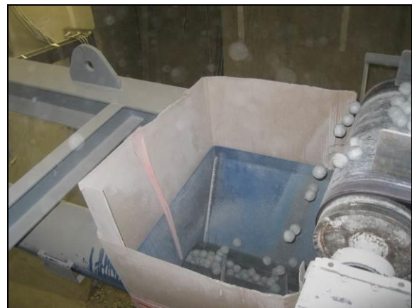
Figure 2.14: Emptying of an octabin containing bentonite pellets (left) and a big bag with bentonite powder (right) into hoppers.
