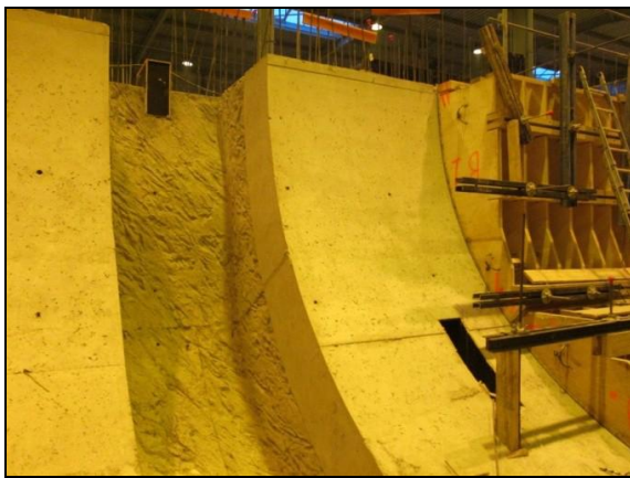
c) the folio pasted on the wood circular inner form to simulate the argillite walls
