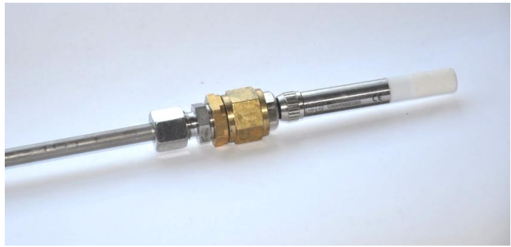
Figure 5 - RH sensor including cabling protection
