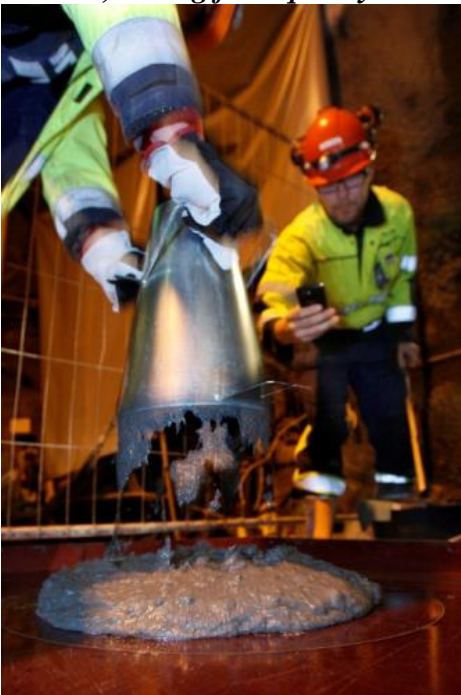
Figure 3. Checking t500 during DOMPLU slump flow test, field quality control.
