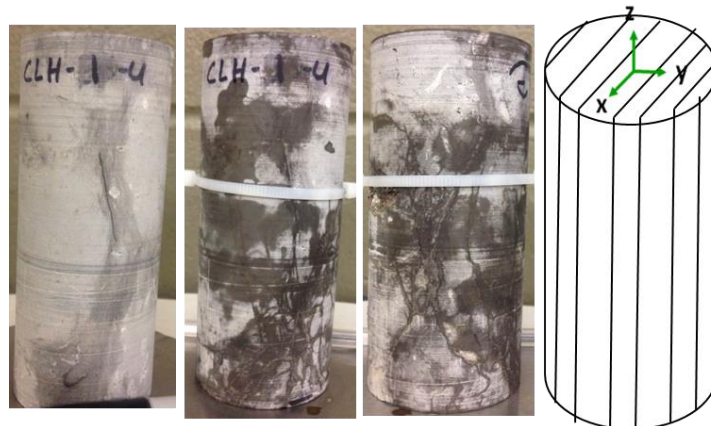
Figure 3-2. Failure mode of specimen CLH-1-U (left image shows intact specimen) and the 3D sketch corresponding to the seismic velocity measurement.
