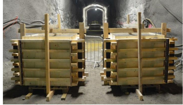
Figure 2. Example of 1m 3 quality control blocks produced with POPLU experiment.
