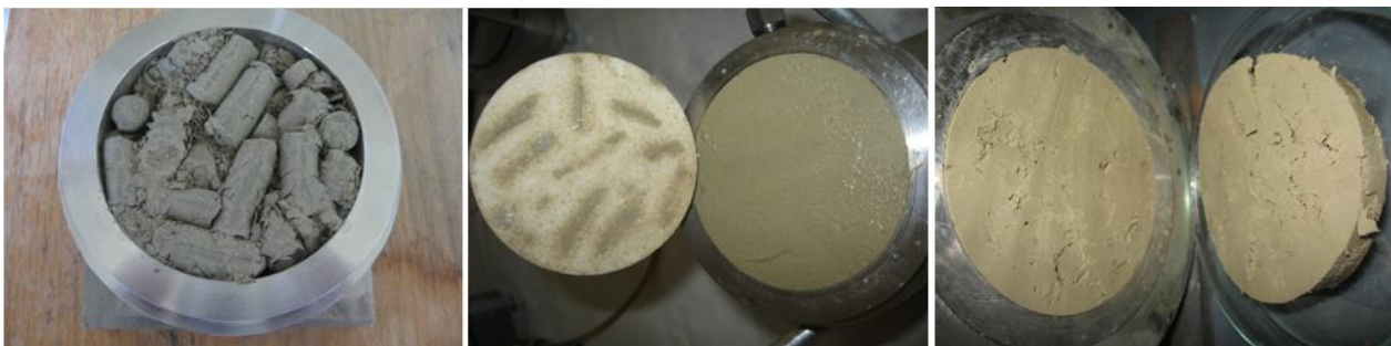
Figure 3-5 State of bentonite pellets before (left) and after 3 days of its saturation (right). Picture in the middle shows the point of water entrance into the sample, the right one the material from the middle of the sample.
