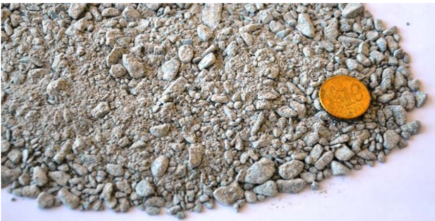
Figure 1: Photo of the granulated bentonite mixture (GBM) produced for the FE experiment.
