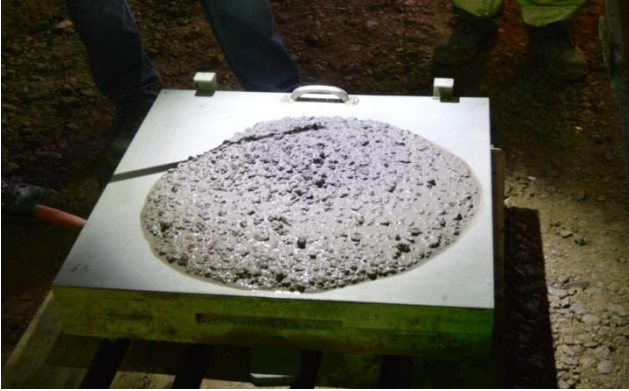
Figure 1. Appearance of POPLU ternary mixture, during field quality control testing.
