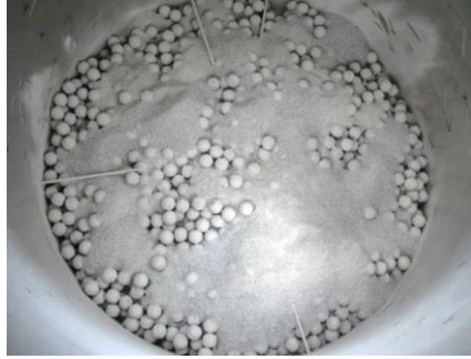
Figure 2 Installation of the first 100 mm of the pellets / crushed pellets mixture
