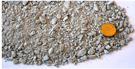
Figure 2: Photo of the granulated bentonite mixture (GBM) produced for the FE experiment.
