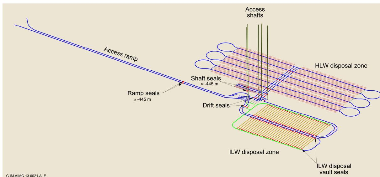
Figure 1.1: Location of the seals (red dots) in the Cigéo concept
