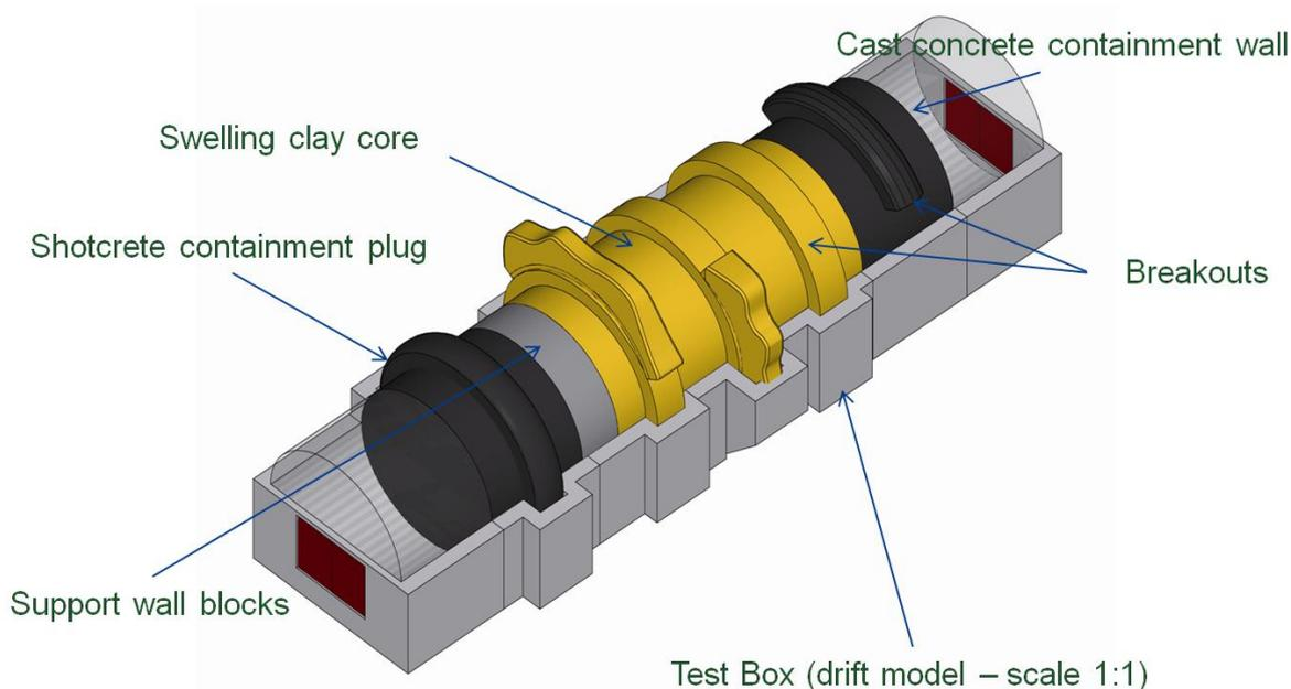
Figure 2.1: Conceptual design of the ANDRA FSS test.
