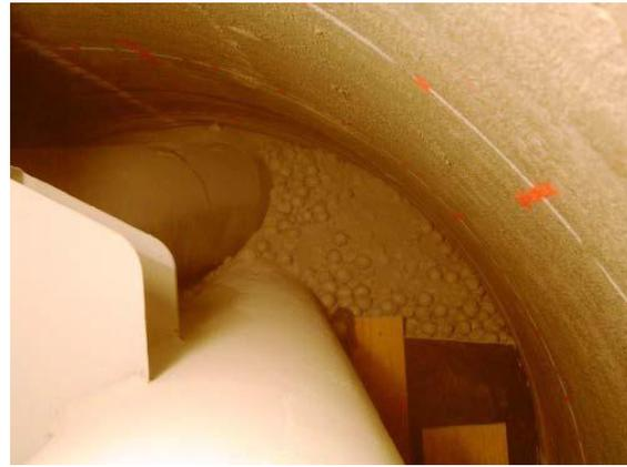
Figure 5.2: Mock-up tests of the bentonite pellet-powder mix using conveying augers
