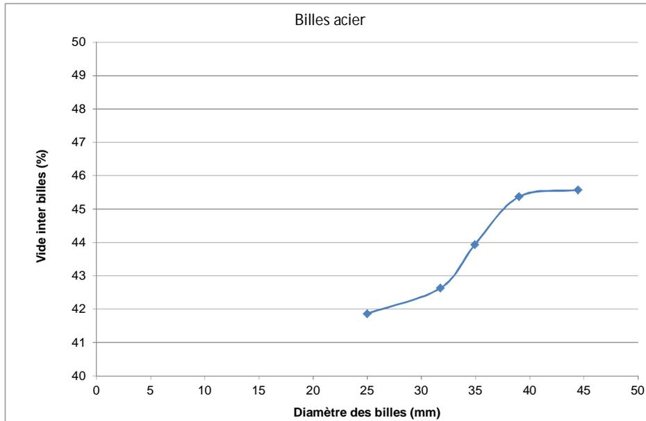
Figure 4.5: Evolution of the “inter-ball” space ratio as a function of the ball diameter
