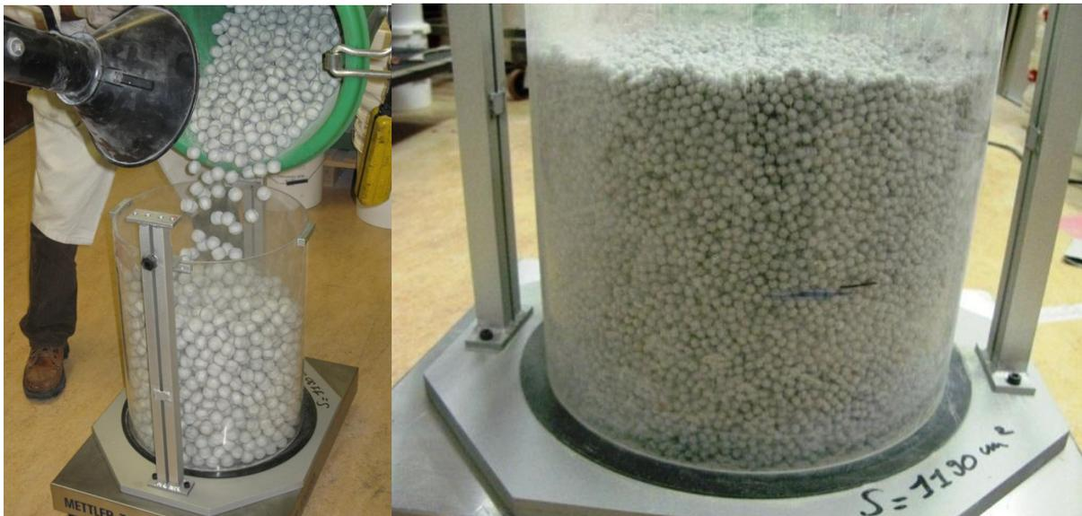
Figure 4.6: Emplacement tests with 28mm (left) and 7 mm (right) OD pellets
