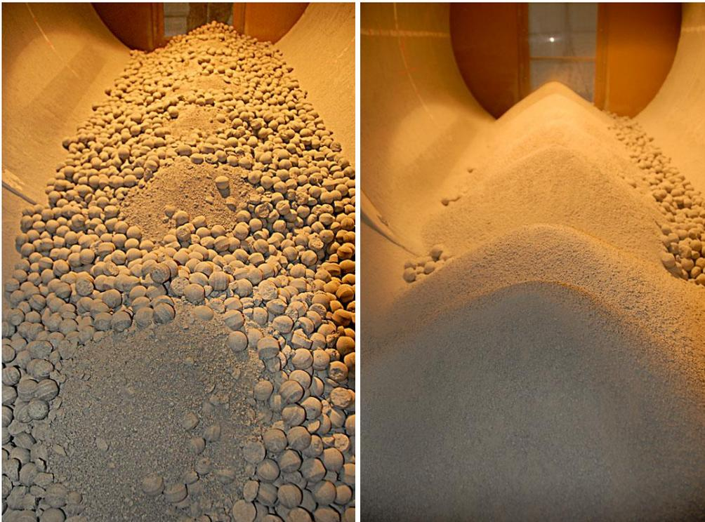
Figure 5.3 : Progressive backfilling of the mock-up pipe
