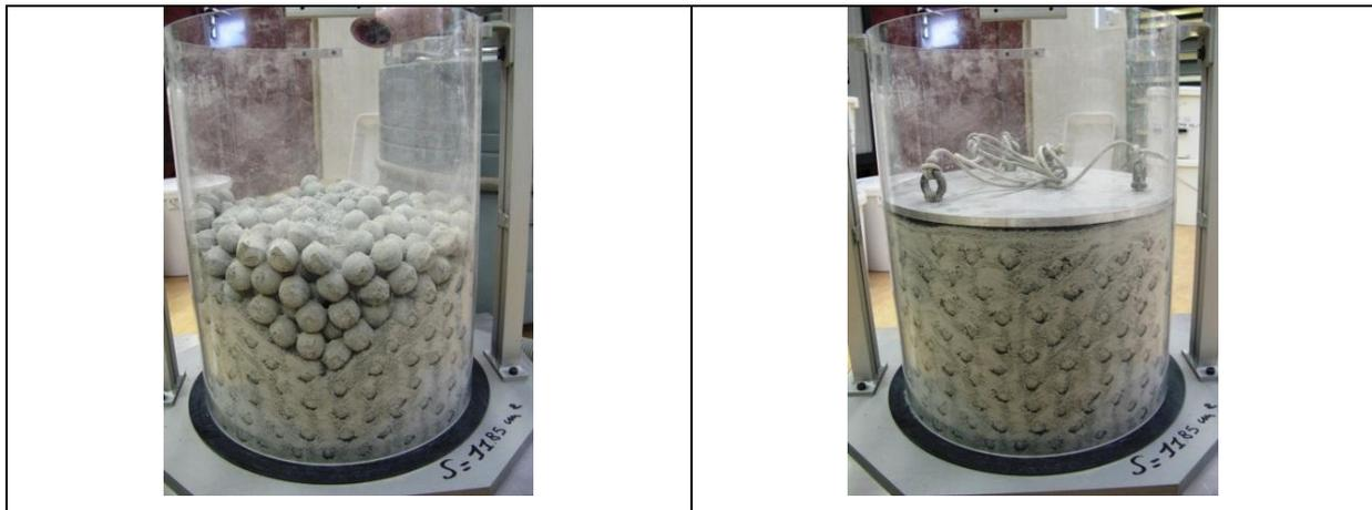
Figure 4.11: Backfilling test with 32mm OD pellets and crushed powder RE13-007
