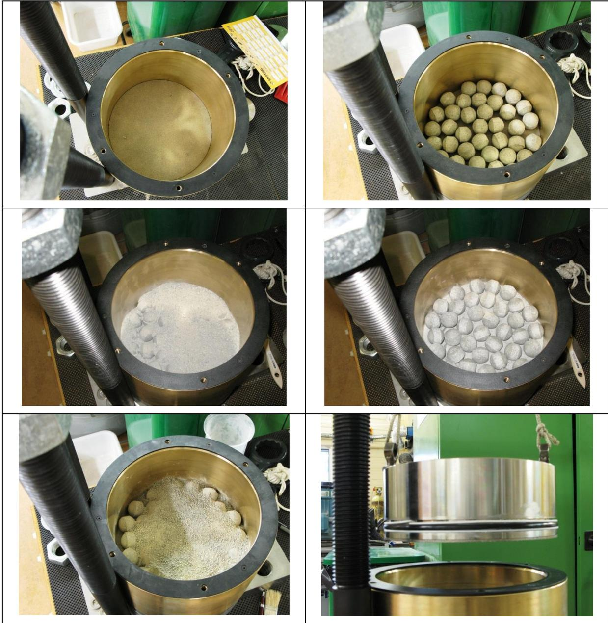
Figure 6.2.1: Illustration of oedometric test cell backfilling with the FSS mix
