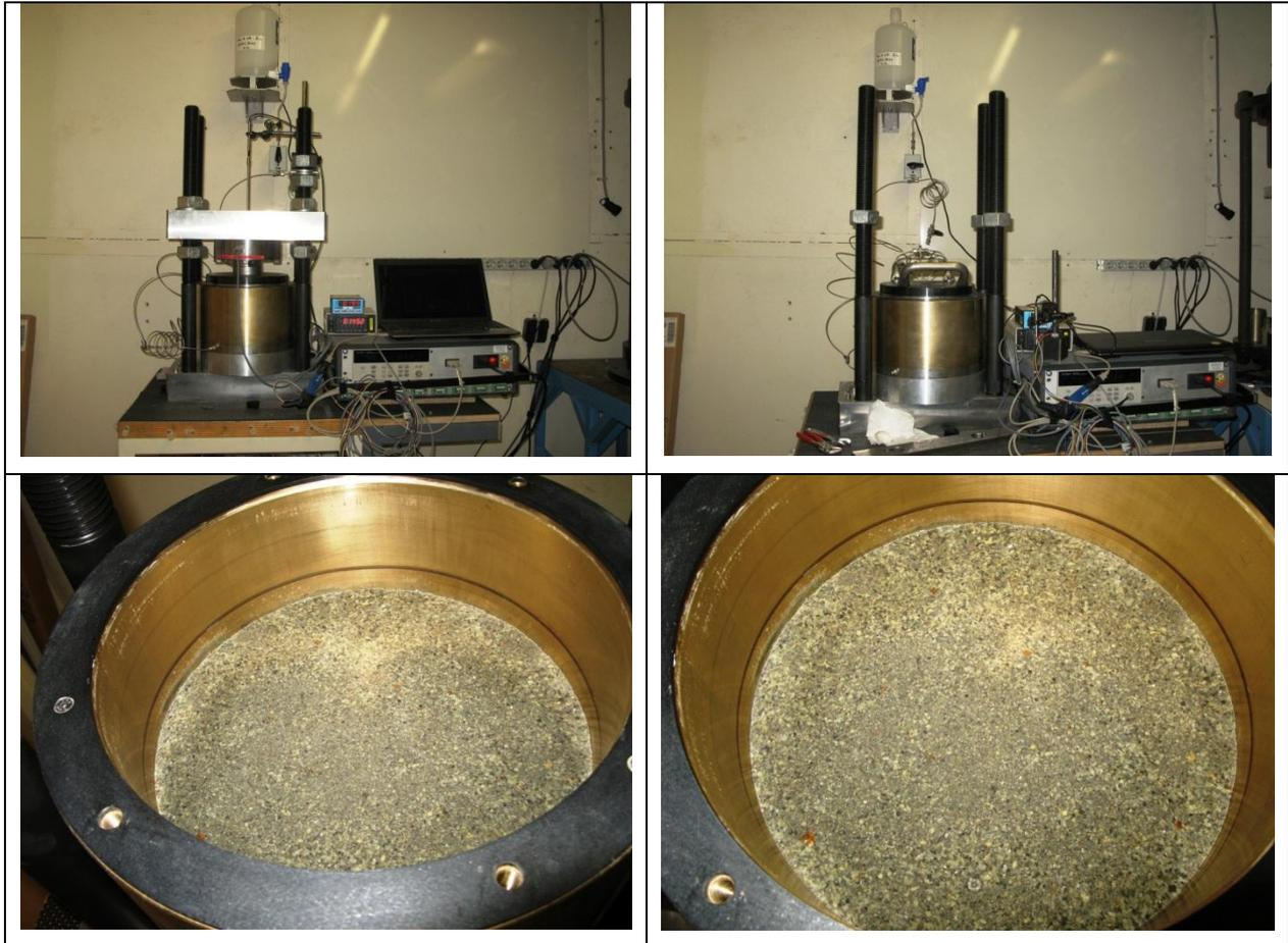
Figure 6.2.2 : Dismantling of test cell and view of saturated/homogenized FSS mix
