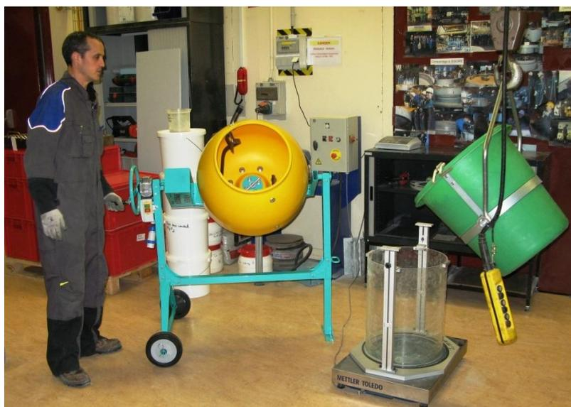
Figure 4.4: View of mixer, polycarbonate cell and tilting bucket used
