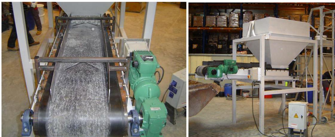
Figure 5.5 : Incorporation into the emplacement test set-up of a pellet conveying belt
