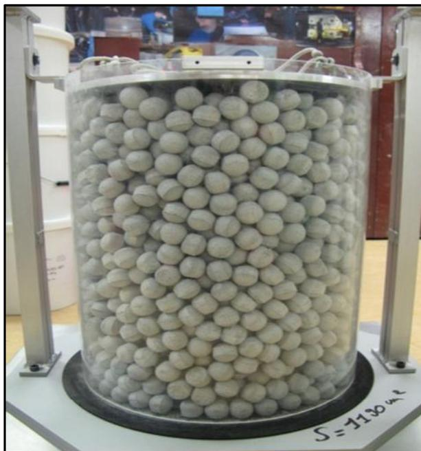
Figure 4.1: Measurement of bulk density with 28 mm OD pellets
