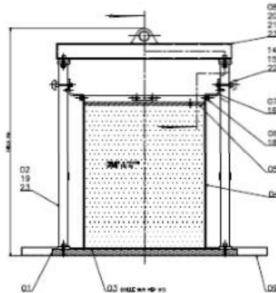
Figure 3.1: Polycarbonate test cell (ID 390mm, H 500 mm) used for the visualizing and weighing of the various pellets and powder assemblies
