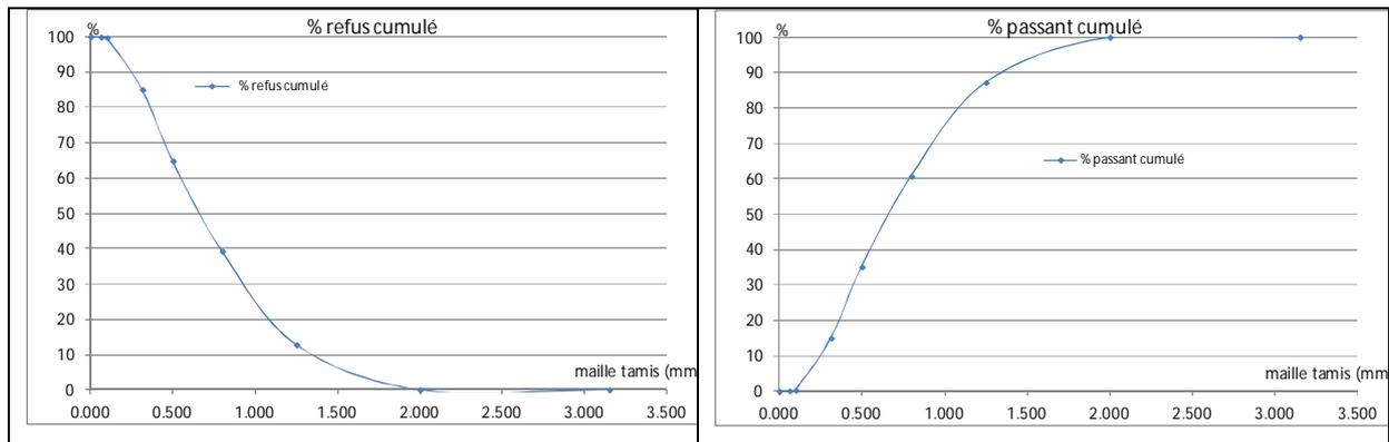
Figure 4.2 : Granulometry of bentonite WH2 powder - Reference LECBA RE12-012
