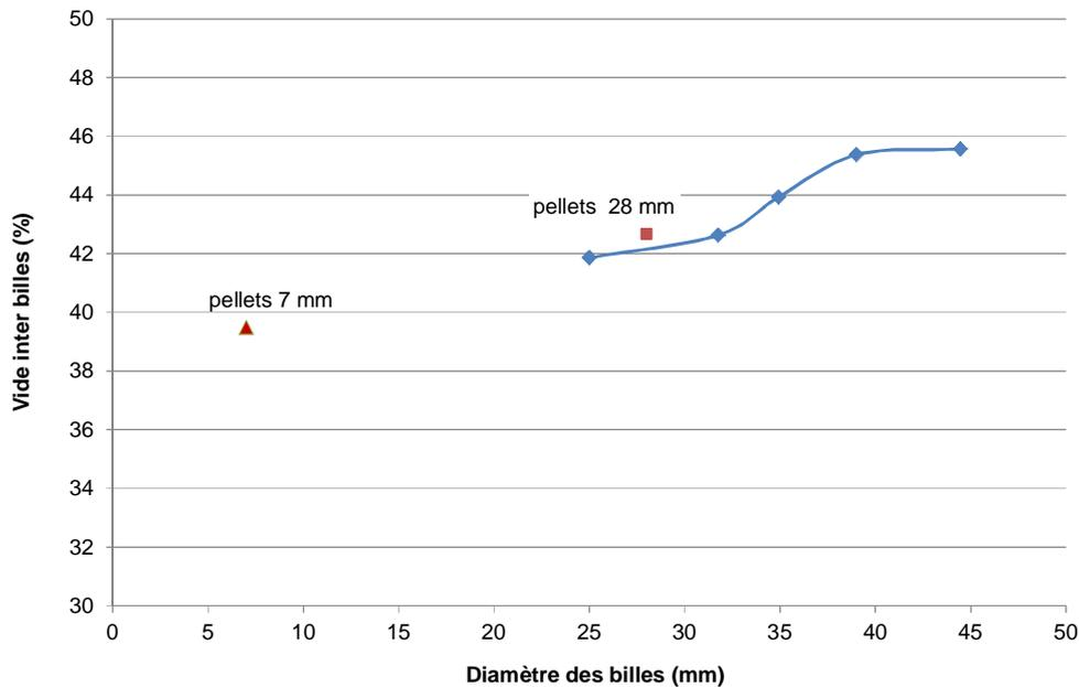
Figure 4.7: Comparison of the inter-pellets void as a function of the pellet diameter
