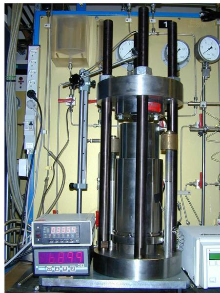
Figure 3.2: Test Cell (ID 120 mm) for measurement of swelling pressure and permeability
