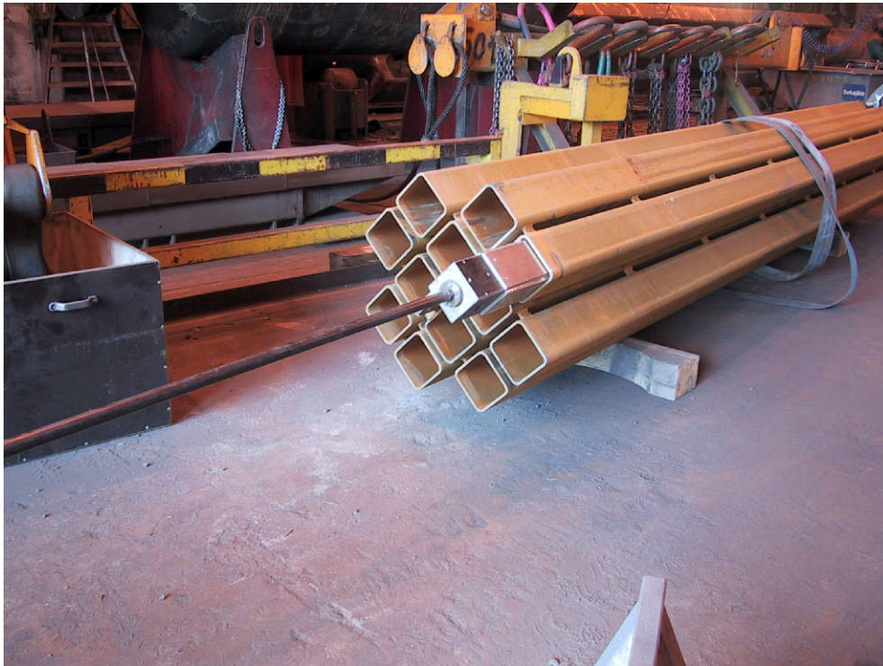
Figure 2. Control of straightness of the square tubes with a gauge.
