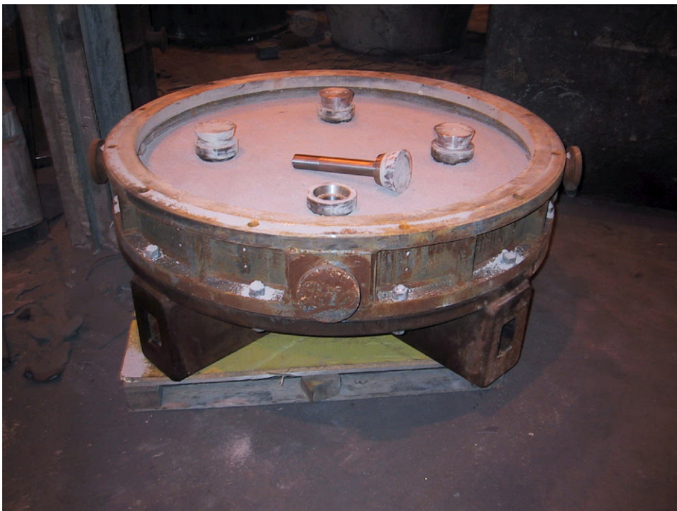
Figure 4. Bottom of the mould as prepared.
