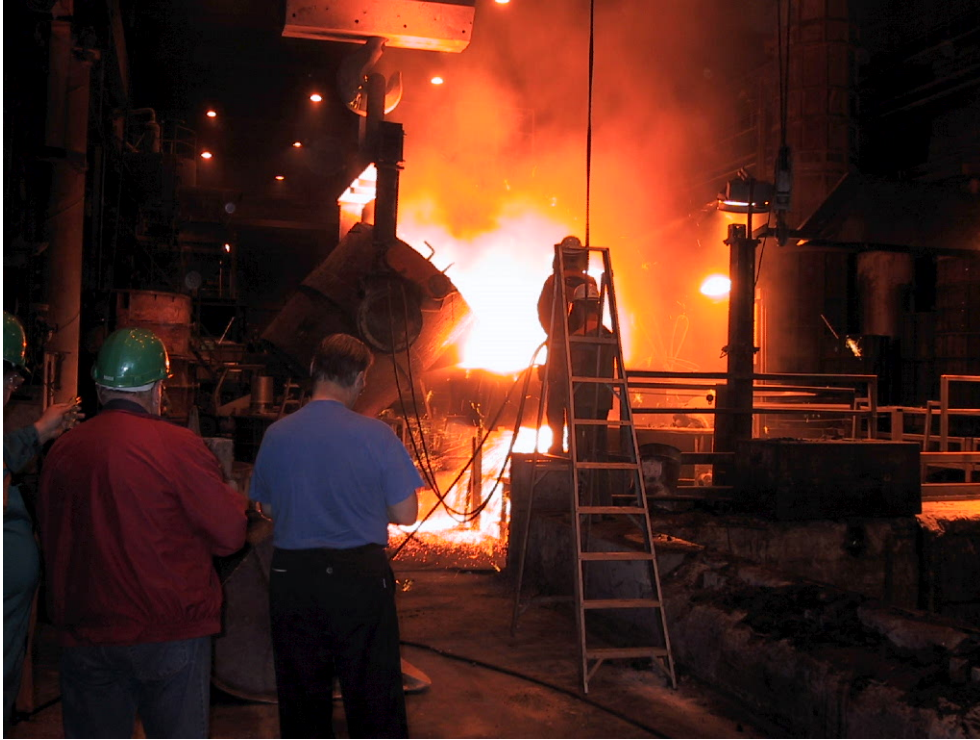
Figure 13. In the end of casting some overflow of melt iron was happening due to oversized charge.
