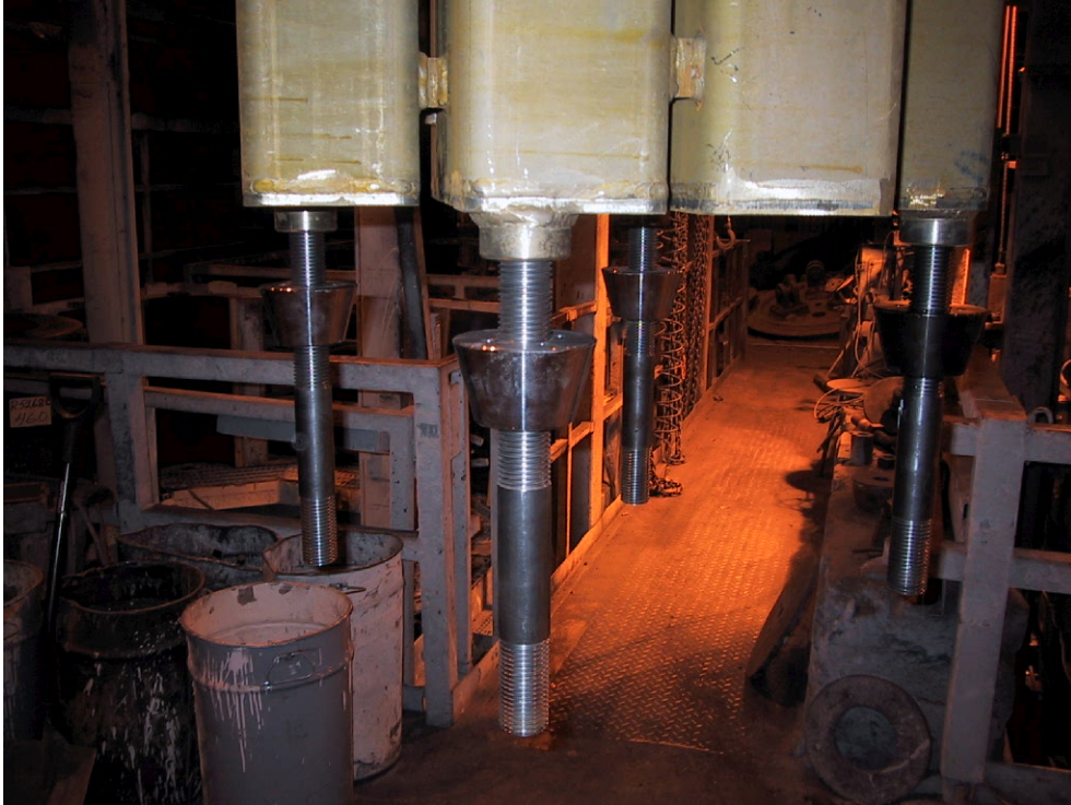
Figure 5. Steel cassette is installed as stained condition into the mould.
