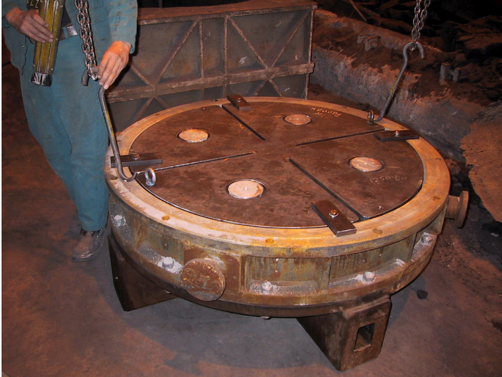
Figure 3. Bottom of the mould is formed from a chill structure (steel plate).
