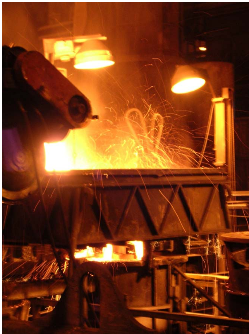
Figure 12. Beginning of casting the canister insert. Photo Jussi Heinonen.
