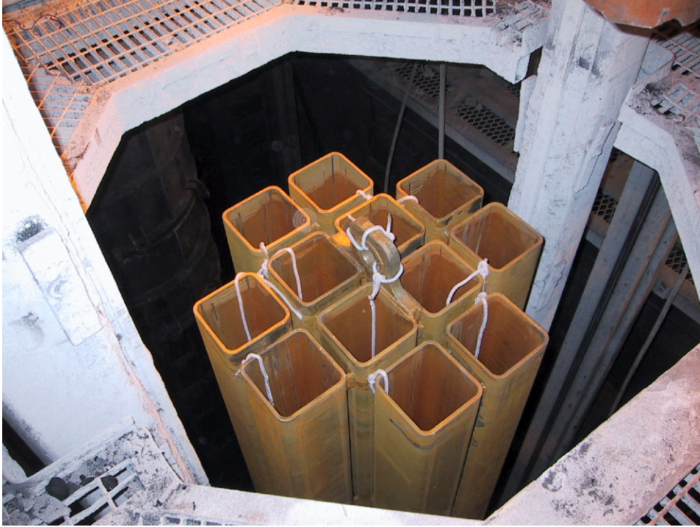
Figure 7. Steel cassette is supplied with gas exhaust strings.
