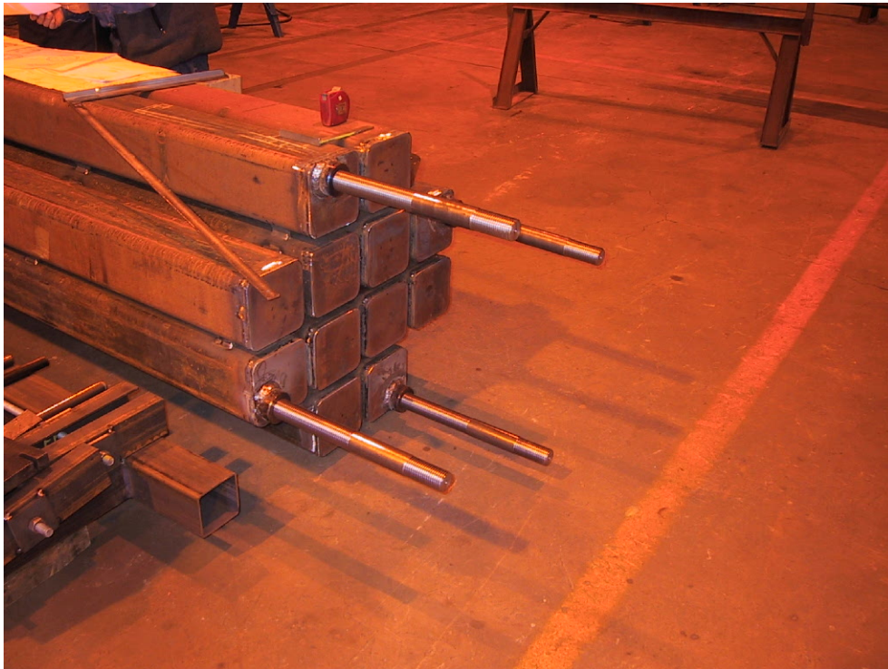
Figure 1. Steel cassette as welded.
