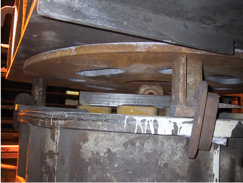
Figure 9. Pouring basin from below. Some 100 mm gap is reserved for cassette expansion upwards during casting.
