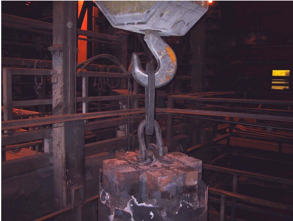
Figure 14. After cooling down the cast block was lifted up from the casting pit and cleaned.
