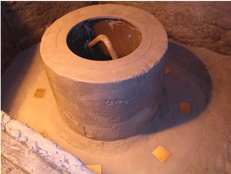
Figure 10. Pouring basin for the melt iron seen from above. See openings in the basin bottom covered by square steel plates. Photo Jussi Heinonen.
