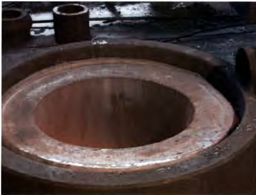
Figure 8. After the first piercing the cup was too much eccentric
