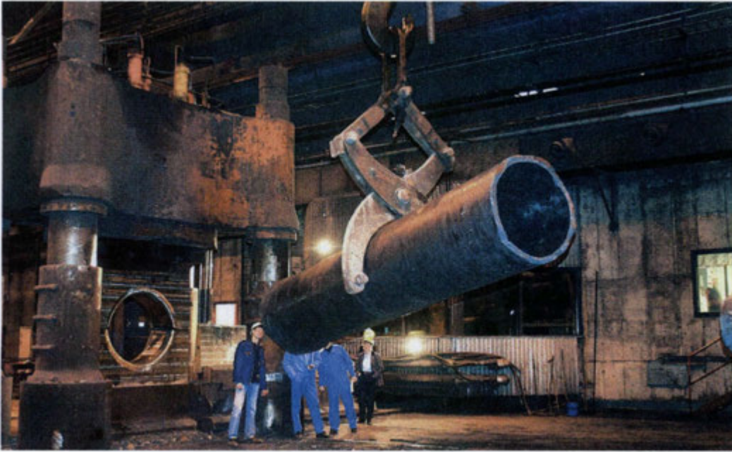
Figure 16. A nearly ready forged cylinder. The semi-circular tools are in the press.
