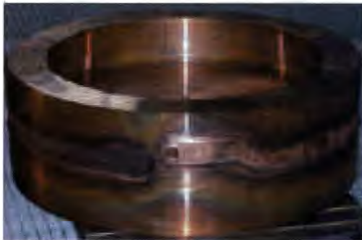
Figure 23. A complete lid closing FSW weld (TWI).
