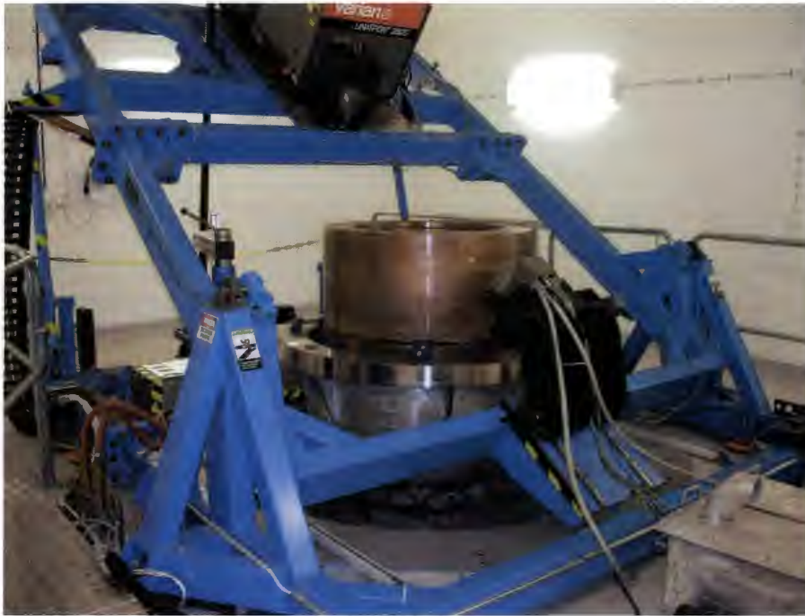
Figure 25. A linear accelerator, 9 MeV for the lid weld radiographic inspection.
