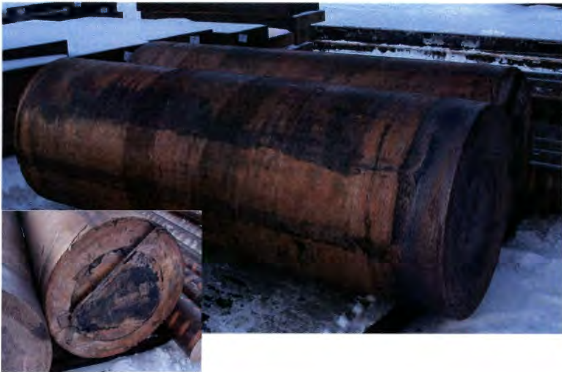
Figure 6. The big billet cast. The start end dovetail pointed out in the down left hand corner.
