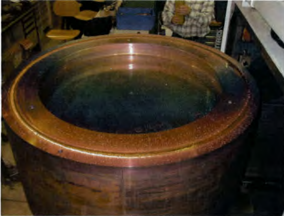
Figure 21. Ready lid closing EBW test at Steigerwald GmbH, 150 kV, beam power 40 kW.
