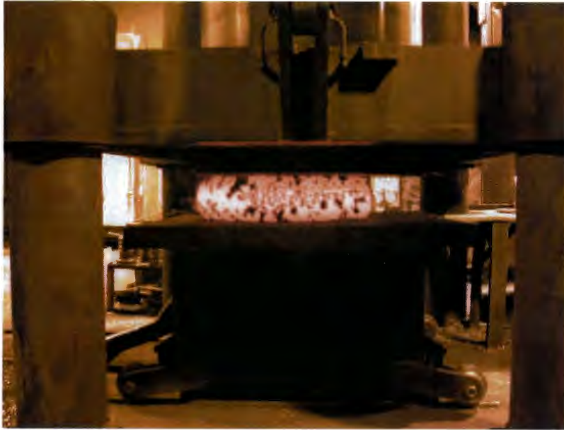
Figure 18. The cast block is hot pressed down to a cake.
