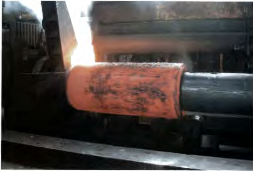
Figure 9. One of the successive expanding phases in the pierce and draw process.
