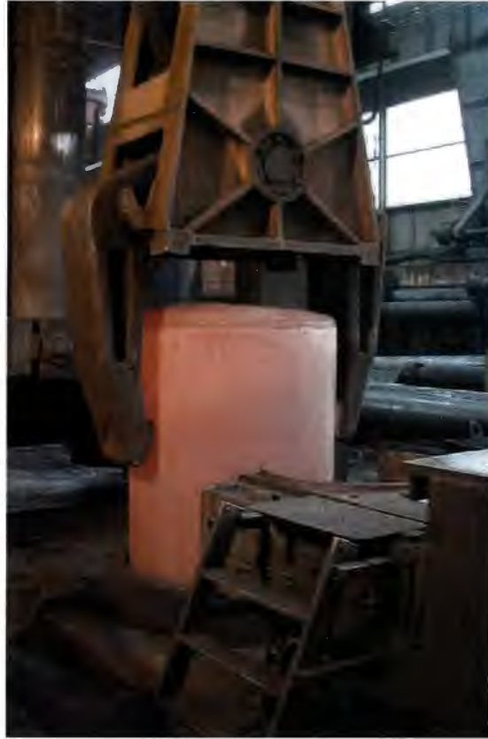
Figure 7. Positioning the billet into the container for upsetting.
