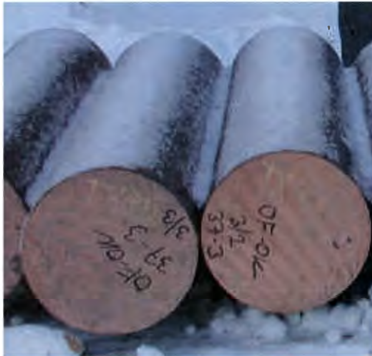
Figure 17. The 350 mm casts for the copper lids and bottoms.
