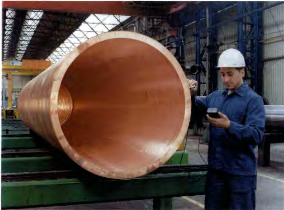
Figure 11. The canister with integrated bottom after final machining to be inspected manually by ultrasound during the development to verify the automatic inspection.
