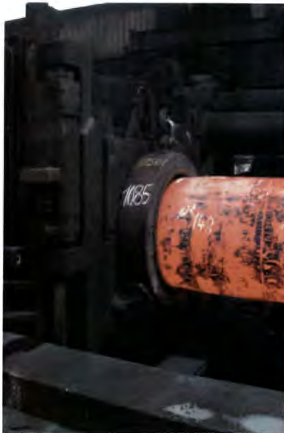
Figure 10. One of the successive drawing phases in the pierce and draw process .
