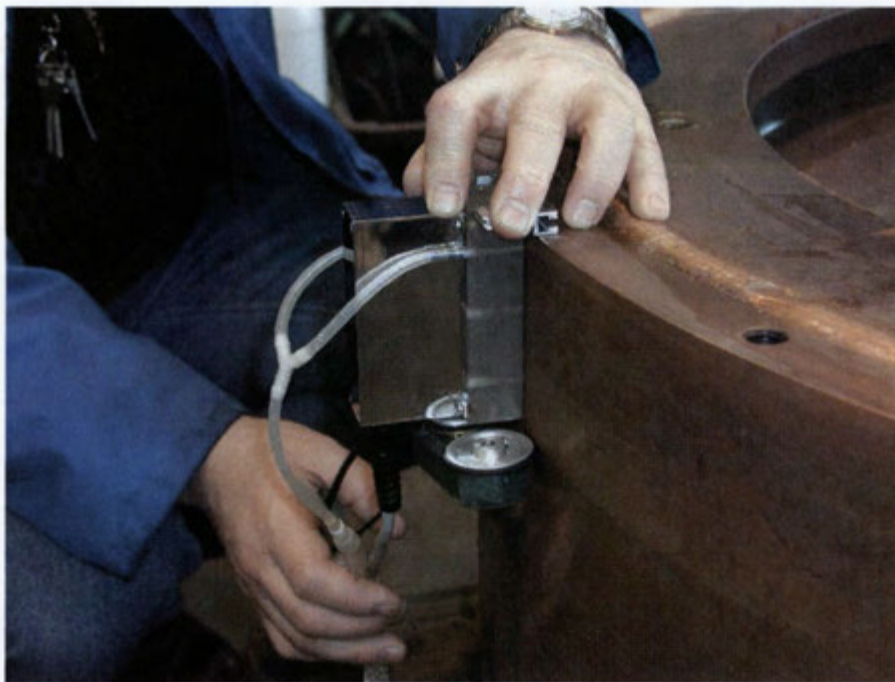
Figure 24. Manual Phased Array Ultrasonic inspection of the lid weld (Inspecta Oy).
