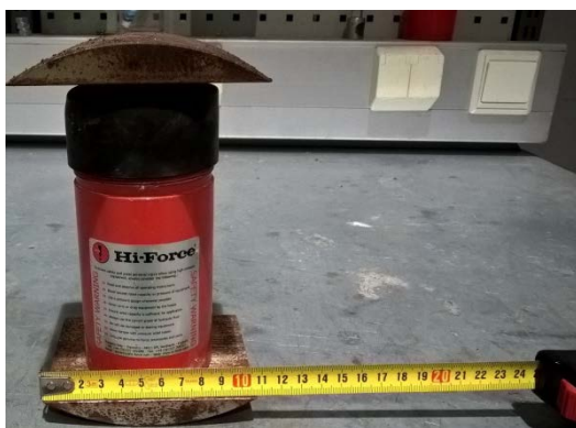
Figure 3-3. Jack baseplates with a jack between them on the left, baseplate dimensions in millimeters on the right.
