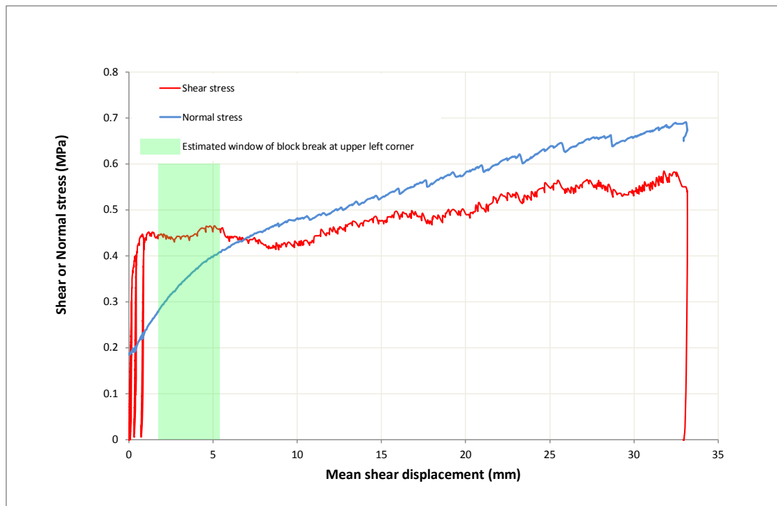
Figure 5-5. Shear and normal stress in MPa vs. mean shear displacement, based on the estimated fracture surface area ( 0.319 \text{ m}^2 ) and combined jack/bolt forces. The estimated window of time for which the test block develops a fracture in the upper left corner is indicated by a shaded green area.
