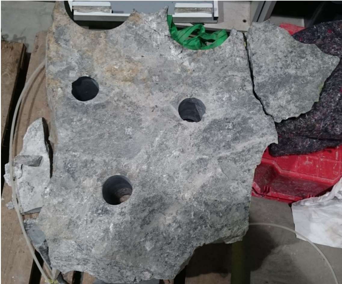
Figure 4-4. The fracture surface of the block along with the upper left part of the block that broke off during shear, located in the upper right part of the image. Note the smaller part that also broke off the right side of the block, located on the left side of the image.
