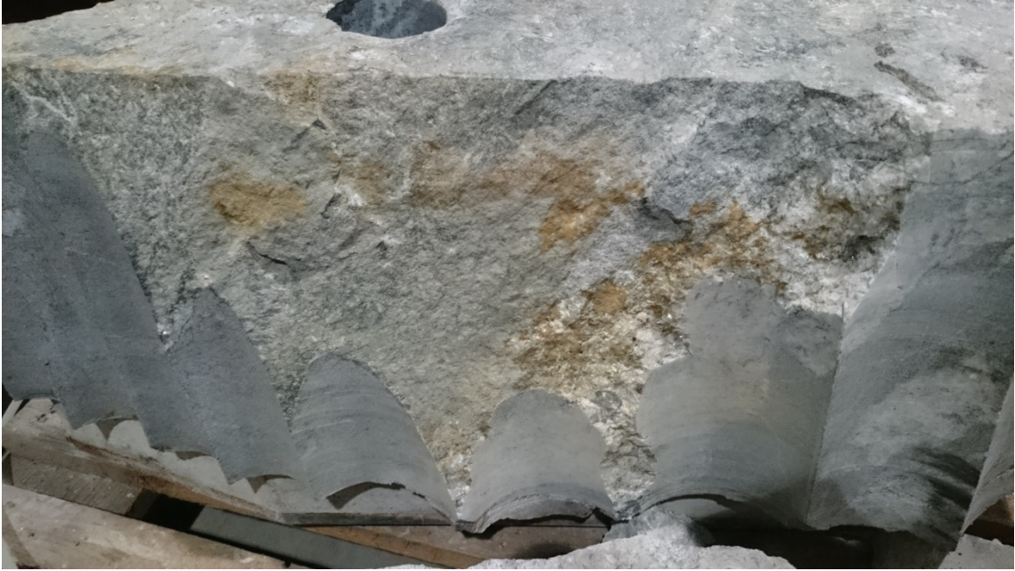
Figure 4-7. A close-up of the natural fracture surface on the right hand side of the block.
