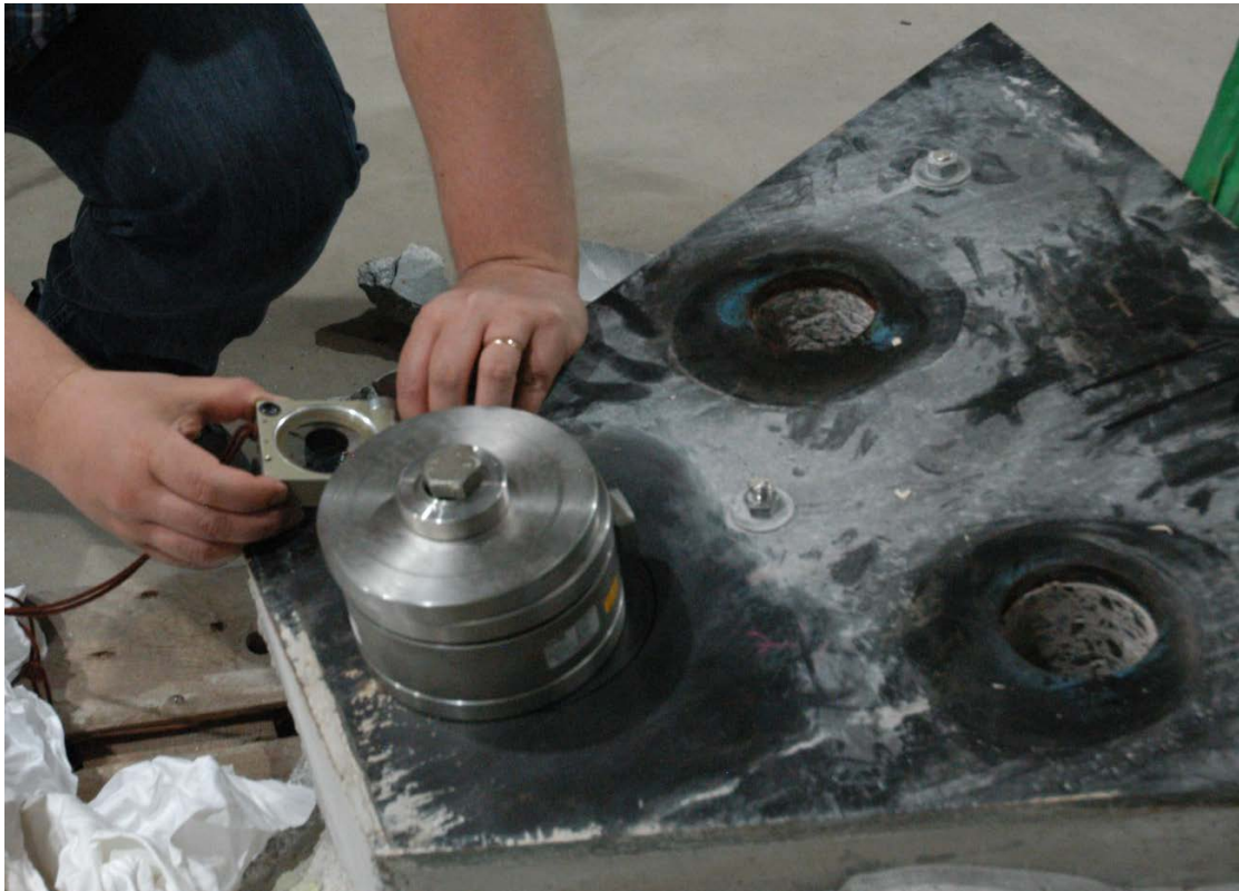
Figure 5-7. Tilt testing of the bolt faceplate and steel plate interface. Note that tilt testing was performed with extra bolt faceplates on top of the original faceplate and load cell configuration so as to minimise adhesion of the lubricant used between the steel plate and the bolt faceplate.
